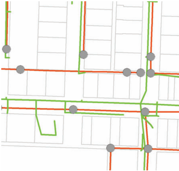
FIGURE 6.81 In this example the storm drains and sewer drains are different colors but the symbol is the same. The manholes are not transparent and are smaller than in the previous example to provide equal focus to the storm and sewer drains.
