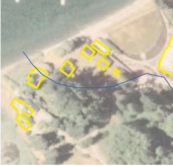
FIGURE 6.98 A high-resolution orthophotograph is the background for these building footprint data. The footprints are outlined so that the orthophotograph can be seen underneath them. The orthophotograph is slightly lightened and only those buildings within a 150-foot buffer of the stream are visible.
