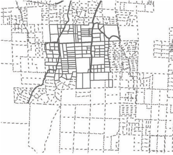
FIGURE 6.45 In this example, the parcels are dotted around the outskirts of town to convey the impreciseness of their boundaries, and the in-town parcels are depicted with solid lines to convey precision. The legend would indicate that the solid lines are surveyed parcels and the dotted lines are hand-drawn parcels.
