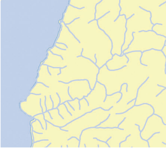
FIGURE 6.9 This is a basic stream map. All streams, regardless of stream order (hierarchy), are the same line thickness and color. The color of the stream lines matches the color of the outlet water.
