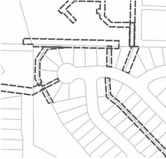
FIGURE 6.82 Easements can be shown in a dashed-line pattern to differentiate them from parcel lines. In this case, the easements were converted from polygon format to polyline format so that the dashed-line pattern would remain consistent (not overlapping).
