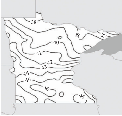
FIGURE 6.64 This black-and-white temperature isoline map has labels that show what the temperature is along that line. Although some GIS software can place labels like this automatically, you may need to use halo text for the labels (especially if using graphics software) or use a symbol with text that has a white background (such as a road sign symbol without the outline).
