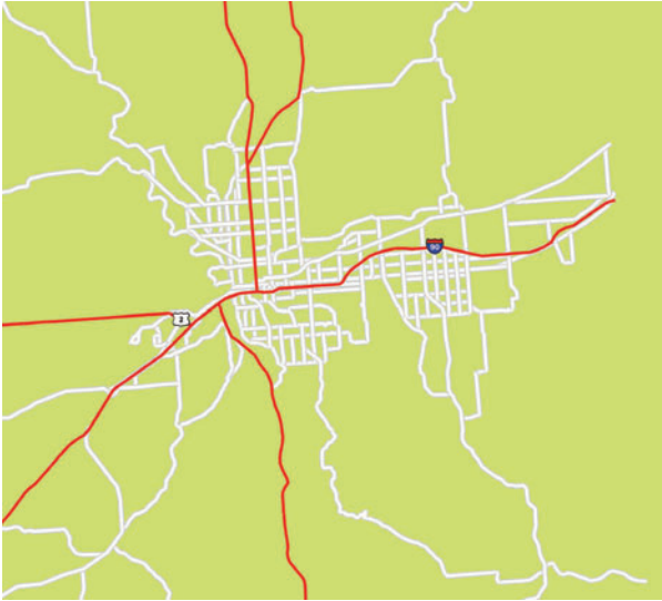
FIGURE 6.3 A classic land background is shown here. It is green with a hint of brown (RGB: 209 224 115). The minor roads are white with gray line edges. Solid red lines form the main arterials.
