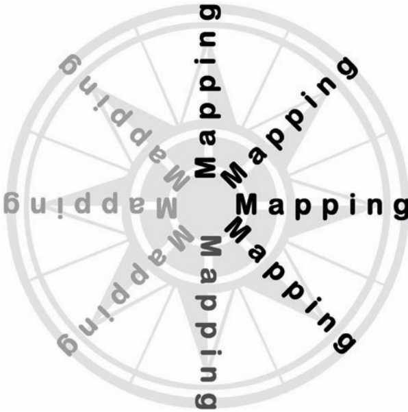
FIGURE 4.20 This graphic is a tool to help you determine which way a label or other type of text ought to read on the printed page. The bolder the text for the word “Mapping,” the better the placement in terms of readability.
