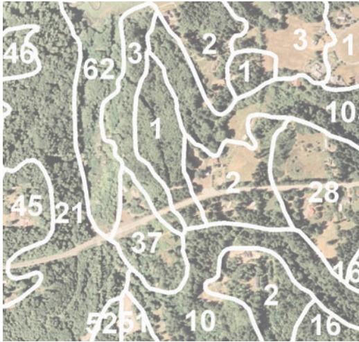
FIGURE 6.102 Because this map displays two overlapping polygon datasets, the soil data are shown as outlines and labels only. If you tried to use a transparent fill symbology for the soils polygons the colors of the orthophoto would mix with the colors of the soils polygons and not create a cacophony of colors, none of which would match the map's legend colors.
