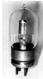
his original Audion tube, a crude forerunner of the triode. By placing an additional electrode between the filament (cathode) and plate (anode), he discovered the ability of the resulting device to **amplify signals of all frequencies**. A few volts' difference at the grid would make a large change in the plate current and could lead to a much larger voltage change at the plate; the result was voltage and power amplification.
