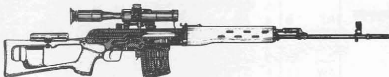
The Dragunov is equipped with a PSO-1 4x optical sight whose reticle is illuminated by a small battery. The scope is capable of detecting an infra-red source.
