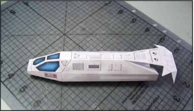
Step 2: After the nose section has dried, begin gluing the area around the cockpit making sure the exterior edges align properly. Once the cockpit area is glued, proceed to glue the bottom of the fuselage forming the tube shape of the final piece.
