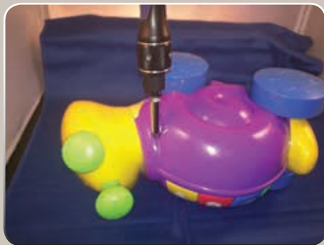
This fancy precision screw driver uses bits, and can't fit into the holes.
