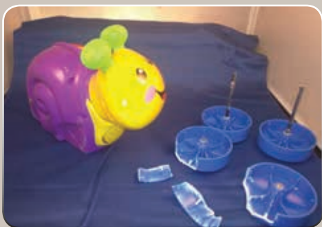
A Hacksaw was used to cut these metal rods to take the wheels off.
