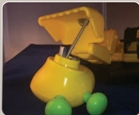
Diggerpillar's head is about to be fastened using a toggle bolt. Due to the angle of the scoop, this would have been a very difficult “glue-up” to attempt. A toggle bolt was chosen as a simpler operation.
