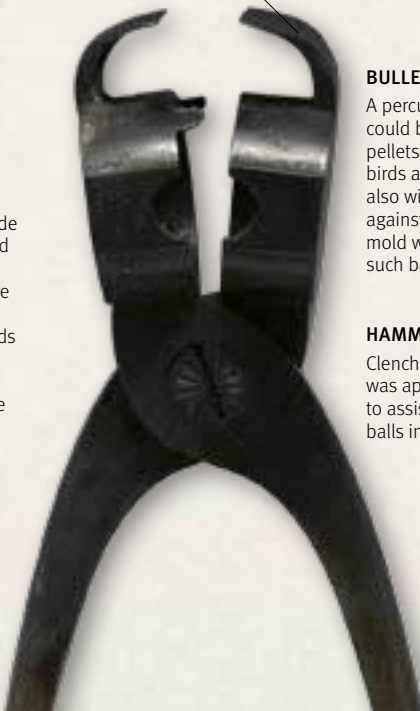
Cutters for removing flashing from moulded bullet
