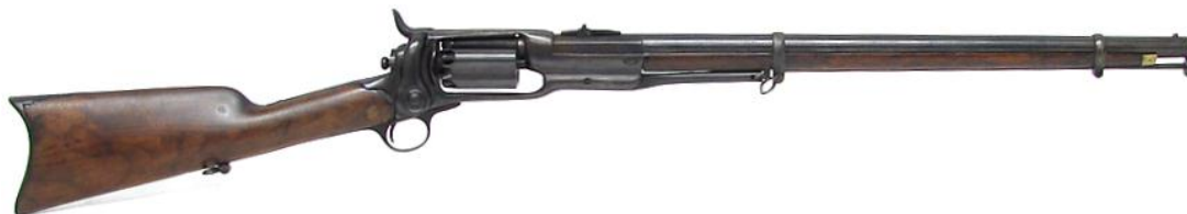
USA, Colt Full Stock Percussion Sporting Rifle, 1856-1864, Single Action, 6 shot Cap & Ball Revolver, .44 cal, 9.5 lb. Also .36, cal with 6 shots, and .56 cal with 5 shots
