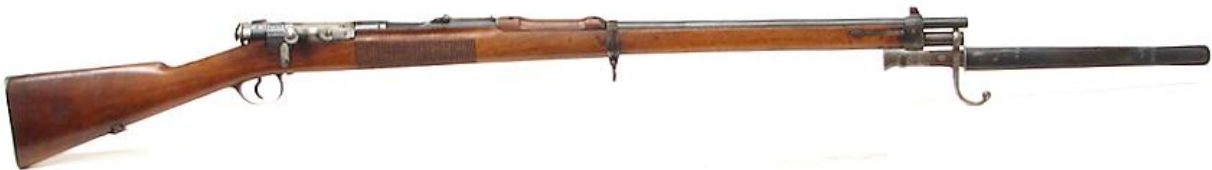
Japan, Murata Year 22 Rifle, 1889, Bolt Action, 8 shot Tube Mag under barrel, 8 mm x53R, 8.5 lb. (with bayonet)
