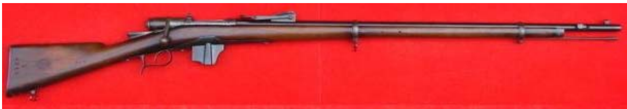
Italy, Vetterli-Vitali Rifle, 1887, Bolt Action, 4 shot Integral Mag, 10.4 x47R mm, 10.2 lb.
