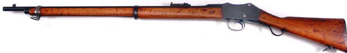
England, Martini-Enfield Rifle, 1895, Lever Action, Single Shot Dropping Block, .303 cal British Rimmed, 9.0 lb.
