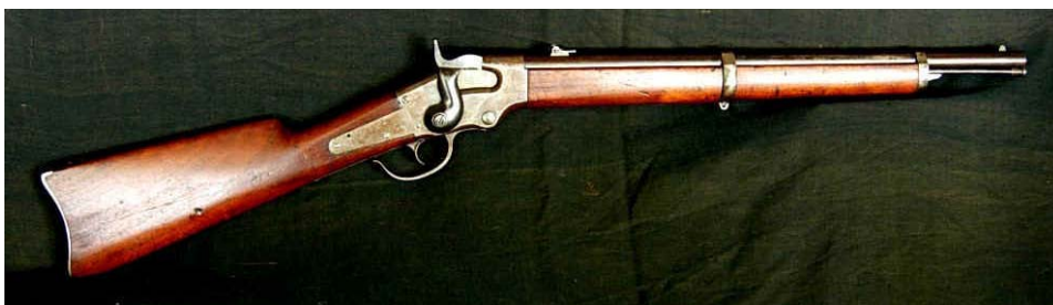
USA, Ball Repeating Carbine, 1864, Lever Action, 7 shot Tube Magazine under Barrel, .56-50 cal Spencer RF, 9 lb.
