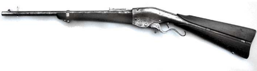
Also: Evans Repeating Carbine Mod 2, 1877, Lever Action, 28 shot Tube Mag in Stock, .44 cal Evans Long CF, 8 lb.
