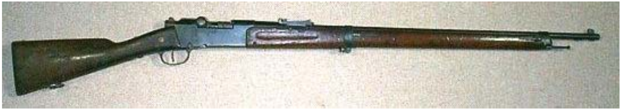
France, Lebel Mod. 1886 & 93 Rifle, 1886, Bolt Action, 8 shot Tube Mag under barrel, 8x50R mm Lebel RF, 9.75 lb.
