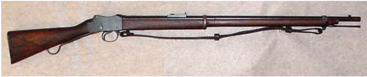
England, Martini-Henry Rifle, 1870, Lever Action Single Shot Dropping Block, .450-577 cal Martini-Henry, 9.0 lb.
