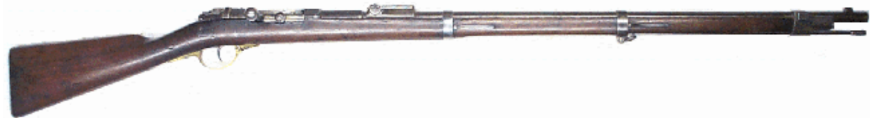
Germany, Mauser Mod. 71 Rifle, 1871, Bolt Action Single Shot, 11 mm Mod.71, 10 lb.
