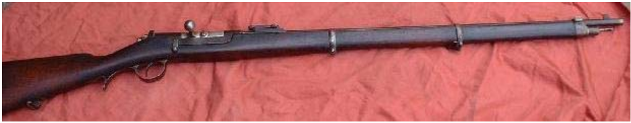
Austria, Kropatchek Mod. 1878 Rifle, 1878, Bolt Action, 8 shot Tube Mag under barrel, 11 mm, , 9.5 lb.
