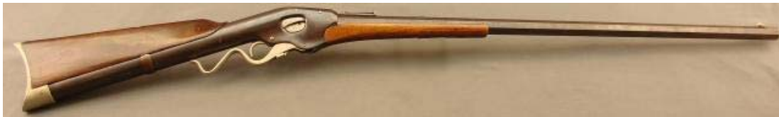
USA, Evans Repeating Rifle Mod 1, 1873, Lever Action, 38 shot Tube Mag in Stock, .44 cal Evans Short CF, 9 lb.
