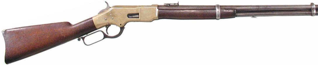
USA, Winchester Mod. 1866 Rifle, 1866, Lever Action, 15 shot Tube Mag under barrel, .44-40 cal SRC RF, 9.5 lb.
