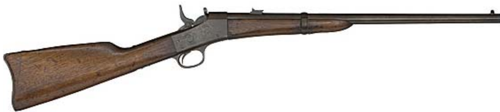
USA, Remington Mod. 1866 Cavalry Carbine, 1866, Lever Action, Single Shot Rolling Block, .50 cal RF, 8 lb.
