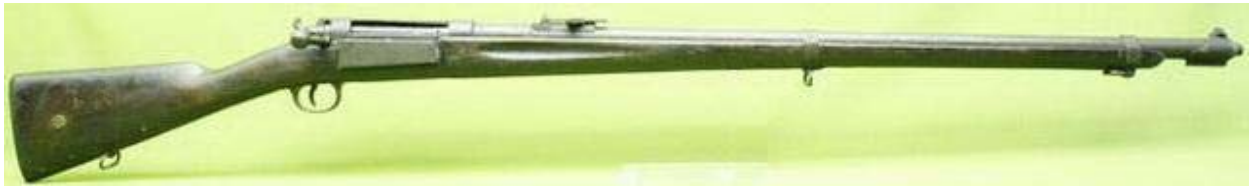
Denmark, Krag-Jorgensen Mod. 1889 Rifle, 1889, Bolt Action, 5 shot Integral Mag, 8 mm, Danish Rim, 9.5 lb.
