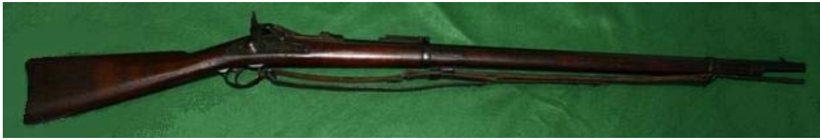
USA, Springfield Mod 1873 Rifle, 1873, Single Shot Side trap door, .45-70 cal, 9.3 lb.
