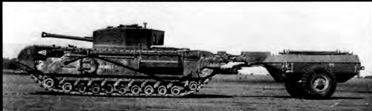
A Crocodile Flamethrower tank with attached fuel tank. This heavily armored vehicle is built on a modified Churchill chassis with a 75mm gun, flamethrower with a 75 yard range, and 2 machine guns.
