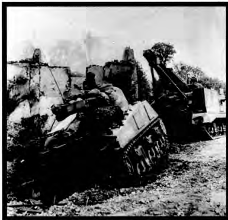
An Armored Recovery Vehicle digs out a wrecked Sherman.
