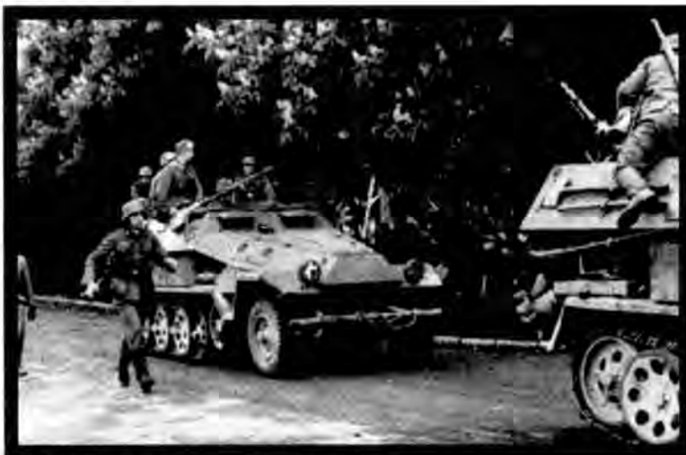
The versatile German halftrack was used to carry troops, machine guns, 75mm antitank guns, and even flamethrowers.
