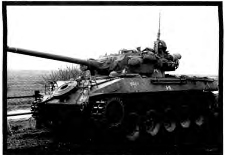
The M24 Chaffee with its 75mm gun was designed to replace the Stuart, but had little additional armor.
