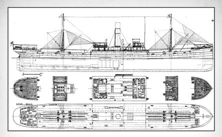
in tanks like the sea water ballast tanks. Coal is stored in coal bunkers. Lateral stability is maintained by ballast tanks and longitudinal trim by the fore and the aft peak tanks. White navigation lights are mounted on the main masts with green lights on the starboard (right) side and red lights on the port (left) side of the ship.
