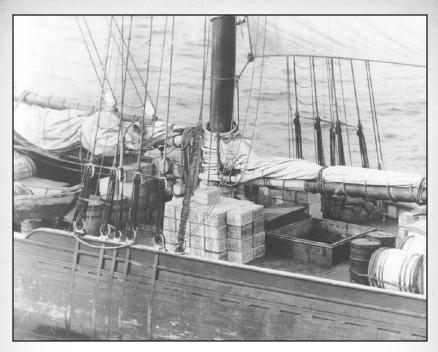
accessing the rigging. The main deck would also include the hatches to the holds. Some ships may have a raised deck aft of the main mast. This area is known as the quarterdeck and usually includes the ship's wheel and binnacle. Often it will also include sky lights to a cabin below.
