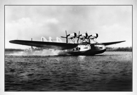
Savoia-Marchetti S.66: A double-hulled Italian flying boat with three engines mounted above the wing. Introduced 1932. Photo above.
