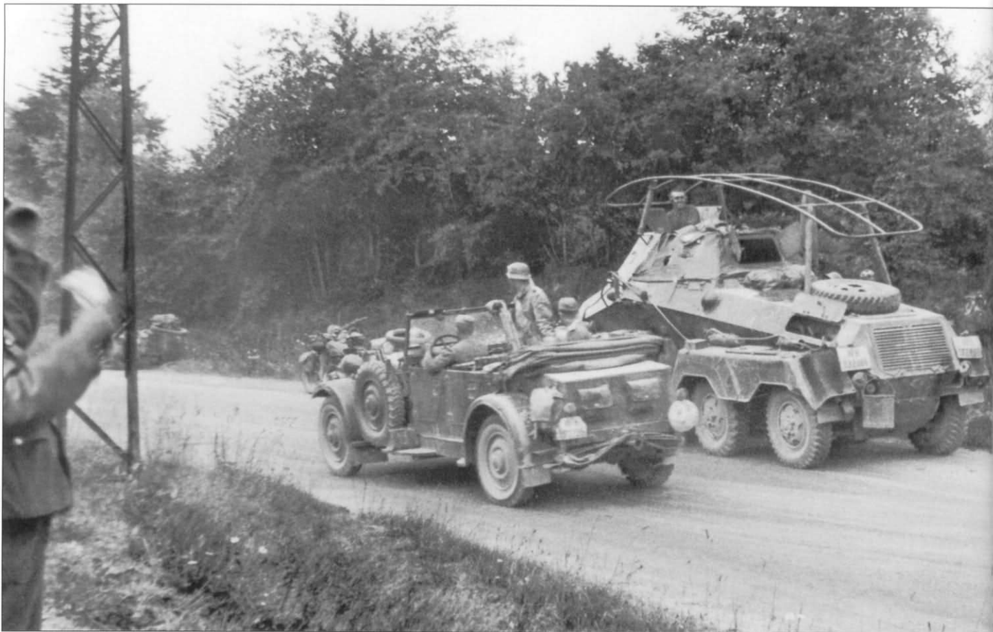
An Adler Type 3 GD passenger car passes an Sd.Kfz. 263 Panzerfunkwagen stopped on a road with some motorcycle combinations. The Adler was one of a multitude of makes and models of automobiles that were used by the Germans in many roles, including command and radio cars, prime movers, infantry transport, and reconnaissance. The armored car has a national cross on its rear ventilation grille.
