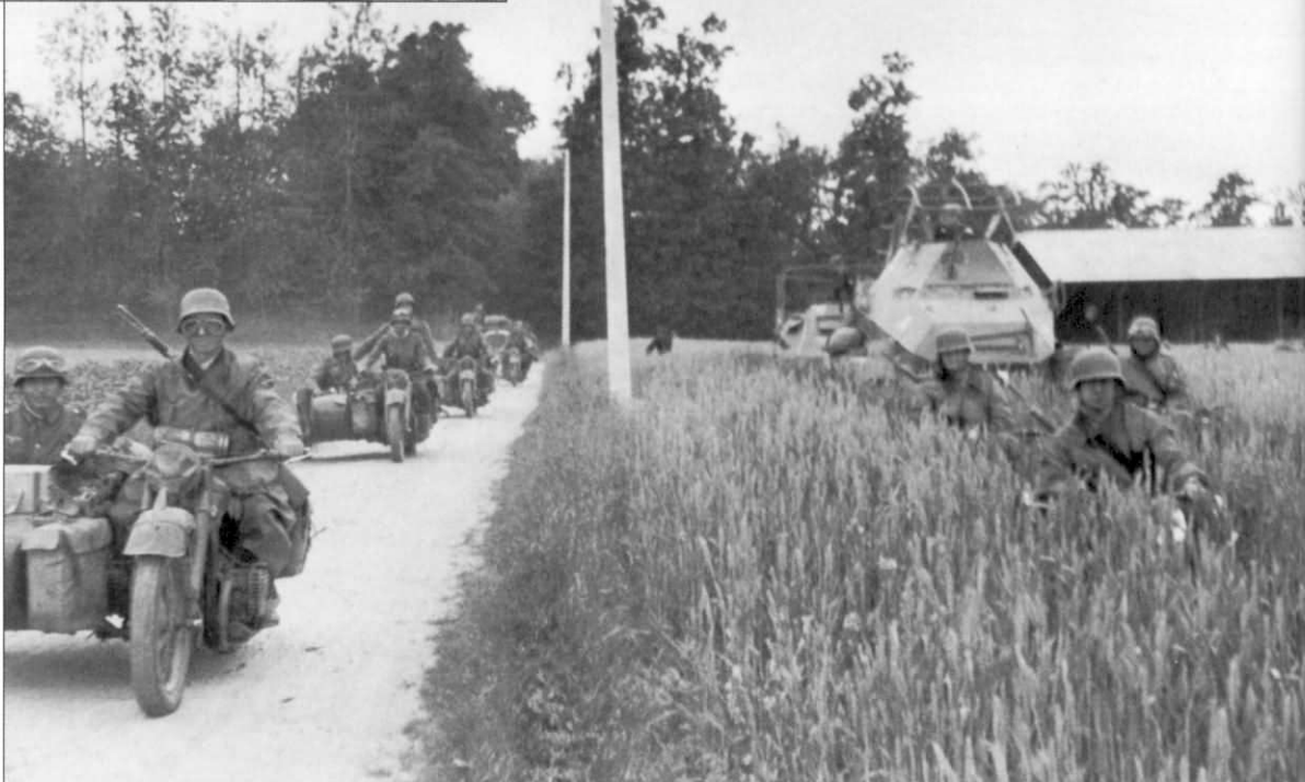
A column of Kradschützen riding BMW R-12 motorcycle combinations pass elements of the 7.Panzer-Division command group in a field of tall grass. Behind the three motorcyclists is an Sd.Kfz.263 Panzerfunkwagen, followed by an Sd.Kfz.223 leichter Panzerspähwagen (Fu). Visible on both sides of the 8-wheeled armored car is the letter "A", which was used on Rommel's personnel 263 armored car, although it may have been a common marking within the Divisional Stab (headquarters) unit.
