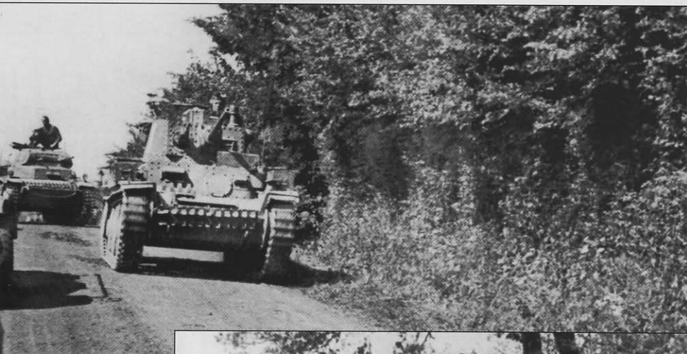
Reconnaissance elements of Rommel's 7.Panzer-Division, presumably from Aufklärungs Abteilung 37, in the vicinity of Cherbourg on June 18, 1944. An Sd.Kfz.223 with its frame antenna folded down follows two Sd.Kfz.232 (8 Rad) and a Sd.Kfz.263 is to the left. Notice the command pennant frame on the side of the nearest armored car.
