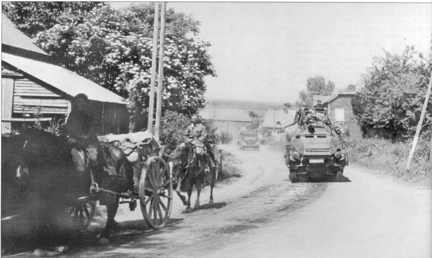
An Sd.Kfz.263 8-wheeled armored radio car travels around a bend on a French road past a horse-drawn unit. The Sd.Kfz.263 was a valuable asset for the signals platoons by providing long range radio communications. It was equipped with a high-powered wireless set, large frame antenna, and a 9 meter telescoping rod aerial for use when halted. Rommel also used one as a command vehicle during the 1940 campaign.
