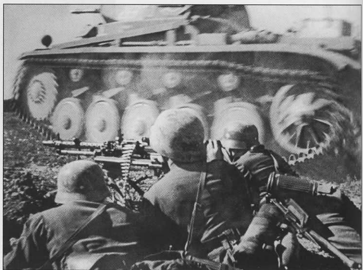
The Panzerkampfwagen II was the most numerous tank to take part in Fall Gelb and Fall Rot. Although still effective as a reconnaissance vehicle, by 1940 it was obsolete as a main battle tank. Armor thickness was one problem and this photograph provides a unique view of the additional armor plate on the lower hull front. The picture is a still taken from the German propaganda film "Sieg im Westen" (Victory in the West). The tactical number "114" is prominently painted in red with white outline.
