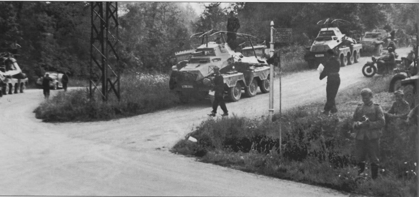
Reconnaissance elements of Rommel's 7.Panzer-Division, presumably from Aufklärungs Abteilung 37, in the vicinity of Cherbourg on June 18, 1944. An Sd.Kfz.223 with its frame antenna folded down follows two Sd.Kfz.232 (8 Rad) and a Sd.Kfz.263 is to the left. Notice the command pennant frame on the side of the nearest armored car.
