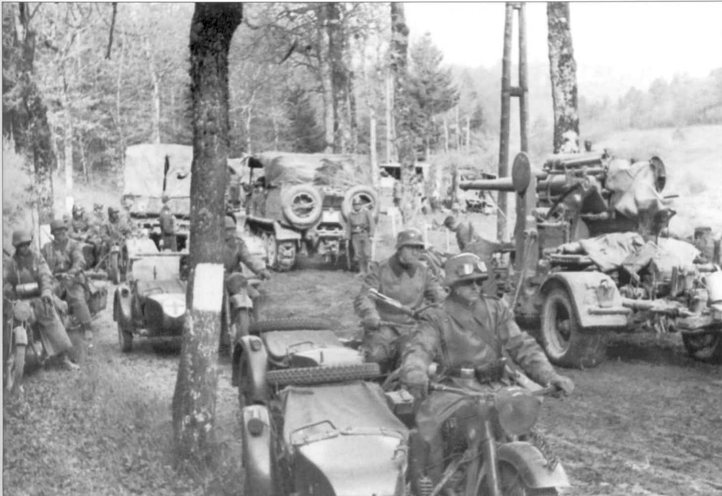
An interesting mix of vehicles traverse a road in the Sedan area. To the right a Daimler-Benz Type DBs7 half-track is in the process of hooking up an 8.8cm Flak 18 anti-aircraft gun. This was one of the many types of prime movers built in the 1930s by various manufacturers until the introduction of the most common version of the Sd.Kfz.7 built by Krauss-Maffei. In the foreground are BMW R12 motorcycle sidecar combinations while halted in the ditch to the left is a column of Kradschutzen (motorcycle rifleman) mounted on what appear to be DKW NZ 350 motorcycles. Other than the Red Cross on the third sidecar and the standard Wehrmacht license plates, no other markings are visible on any of the vehicles.
