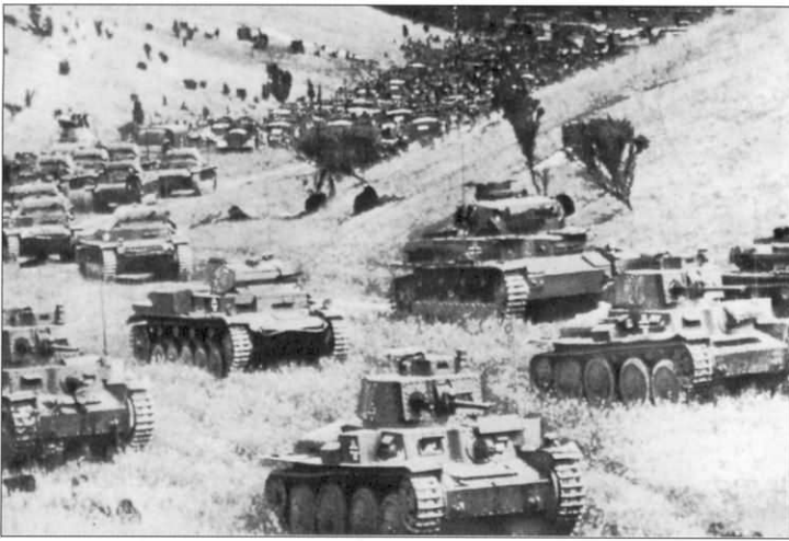
Massed elements of Rommel's 7.Panzer-Division leave the Somme River valley through La Grande Vallee on June 5. Numerous types of armored vehicles can be seen, including three Pz.Kpfw.38(t) Ausf. B or C, a single Pz.Kpfw.IV Ausf.D with another Pz.Kpfw.IV in front of it, at least nine Pz.Kpfw.II Ausf.A-C, and an Sd.Kfz.263 armored car. Passenger cars and trucks of every type appear in the distance. Considering that most of the Panzer-Divisions had over 150 tanks at the start of Fall Rot, those seen in the photo are only a very small portion of the armored vehicles in 7.Panzer-Division.
