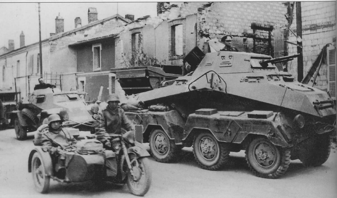
An Sd.Kfz.231 (8 Rad) and Sd.Kfz.223 pause in a heavily damaged French town while a BMW R12 motorcycle sidecar combination passes by. Most markings are obscured except for the national cross on the lead armored car but the divisional insignia of 6. or 7.Panzer-Division is just visible on the front of the radio car. The commander of the 8-wheeled armored car is wearing the Schirmmütze or officers peaked service cap.
