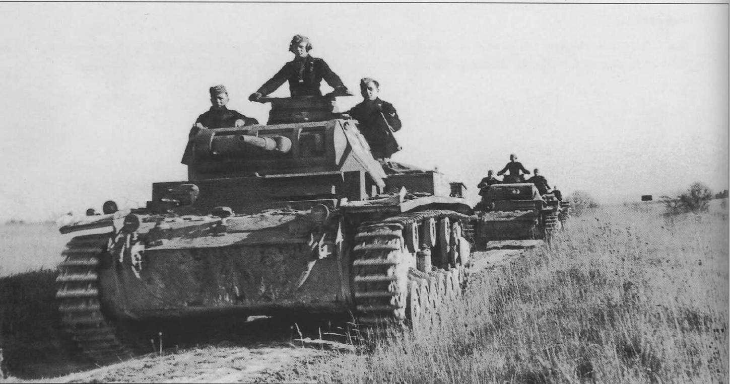
A column of Pz.Kpfw.III advance along a dirt track while the turret crewmen catch a breath of fresh air. The lead vehicle is an Ausf.F, while the second is an E model since it is missing the brake cooling air intake covers on the glacis plate. Barely visible on the turret side is the stenciled bison insignia of the 9.Panzer-Division's Pz.Rgt.7. A national cross is located on the field fitted stowage box mounted on the fender.
