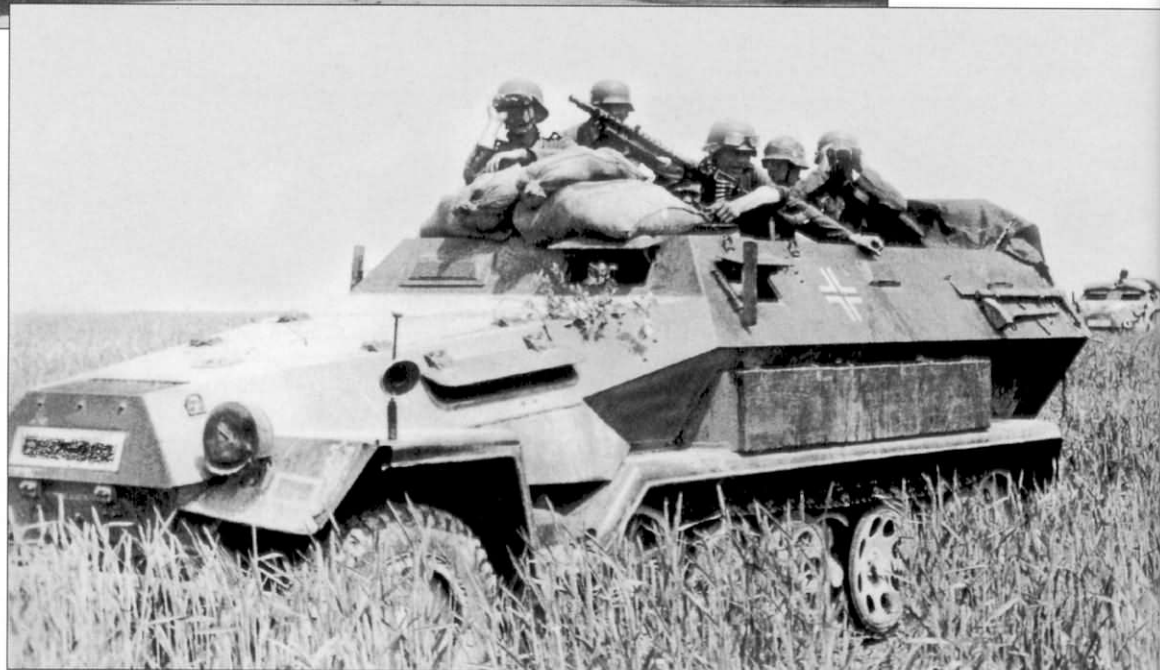
A group of Sd.Kfz.251 Ausf.A halftracks halt in a field in the Aisne sector of France to observe something in the distance. The oakleaf emblem of 1.Panzer-Division is visible on the fender as well as the tactical symbol for motorized infantry. Sandbags are being used to provide protection for the MG34 machinegun, which is mounted on a swing arm identical to the one carried above the rear doors. Later versions of the Sd.Kfz.251 were equipped with a shield for the forward machinegun due to the experiences in France and Poland.
