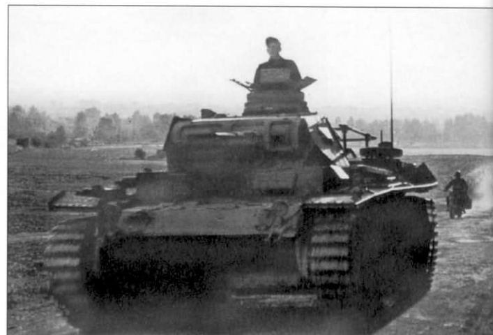
With its large frame antenna visible over the engine deck, a Panzerbefehlswagen III Ausf.E command tank is seen near Peronne, France, during Fall Rot. No markings are visible and this vehicle has what appears to be a Panzerkampfwagen II style armored visor cover over the driver's viewport instead of the standard Pz.Kpfw.III vision block.
