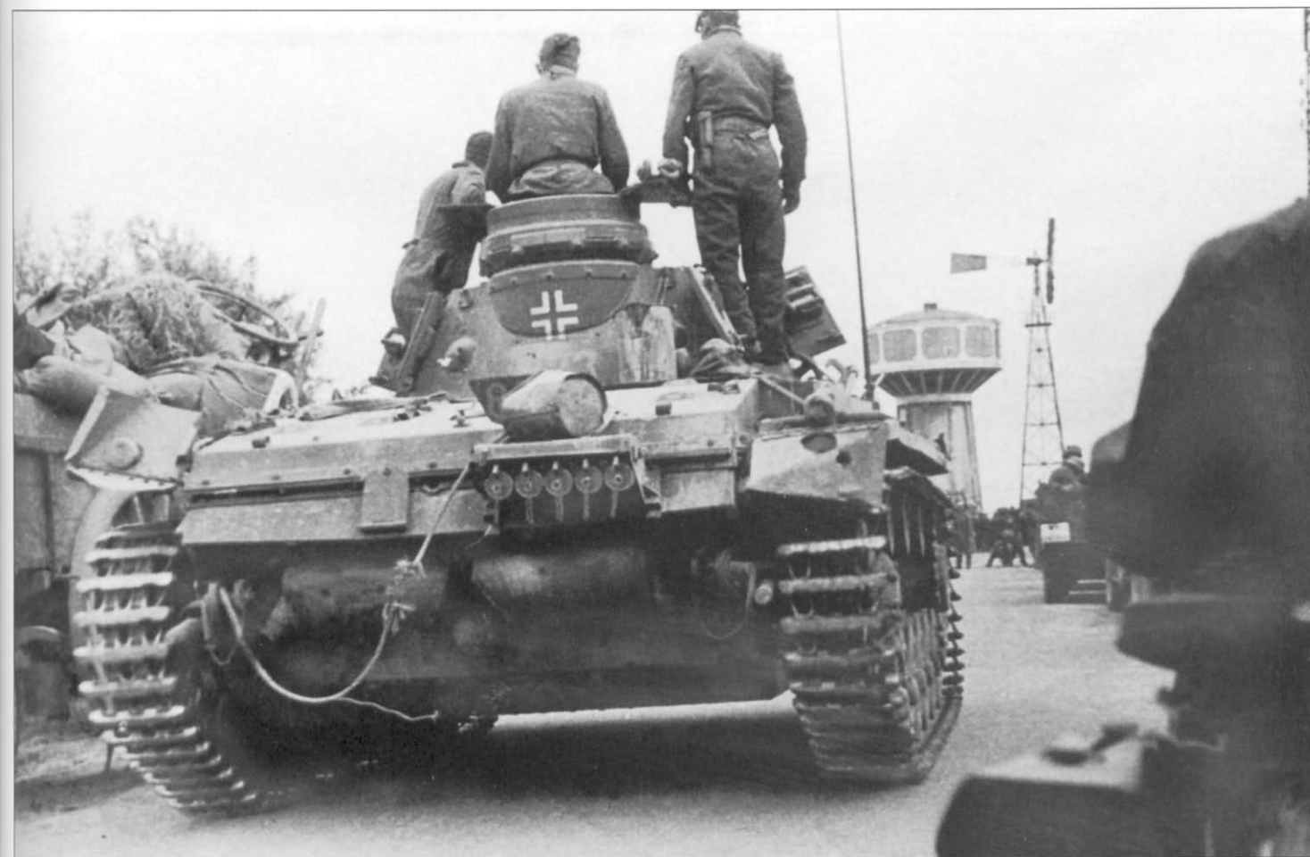
Another photograph taken a short time after the previous one, as the wagon to the left appears in both pictures. The identity of this Pz.Kpfw.III Ausf.E/F is unknown, as 7.Panzer-Division was not equipped with Panzer IIIs. A very faint turret number in yellow, "823", appears below the cupola bulge, which is also not characteristic of this division. It is possible that it belongs to 5.Panzer-Division, which operated alongside 7th for both Fall Gelb and Fall Rot, and has somehow become mixed up with the wrong unit during the advance. The tail of the windmill seems to be painted in the French tricolor.
