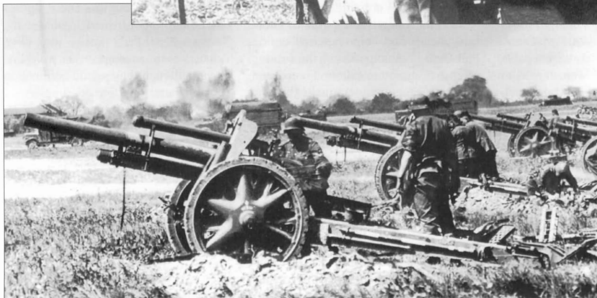
A battery of 10.5cm leFH 18 field guns with their prime movers and ammunition trucks in the background. Each panzer division was authorized one artillery regiment with 3 battalions, two equipped with 10.5cm guns and the other with 15cm guns. A battalion had 3 batteries, each with four guns as seen here. The third leFH 18 appears to have just fired, as the barrel is in full recoil.
