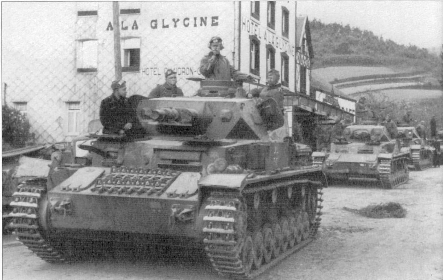
Travelling through the Belgian town of Vresse on May 12, a column of Pz.Kpfw.IV approach their crossing location over the Semois River. The Semois was the first major river obstacle that Pz.Gruppe von Kleist had to cross. The lead vehicle is an Ausf.D, while those following are either Ausf.B or C. The 2.Panzer-Division emblem of 2 yellow dots appears below a yellow rhomboid both on the lower hull plate and beside the driver's visor. A small "5" next to the lower one signifies the 5th company. The following vehicle displays similar markings but the divisional sign has been moved to a centralized location on the upper superstructure plate.
