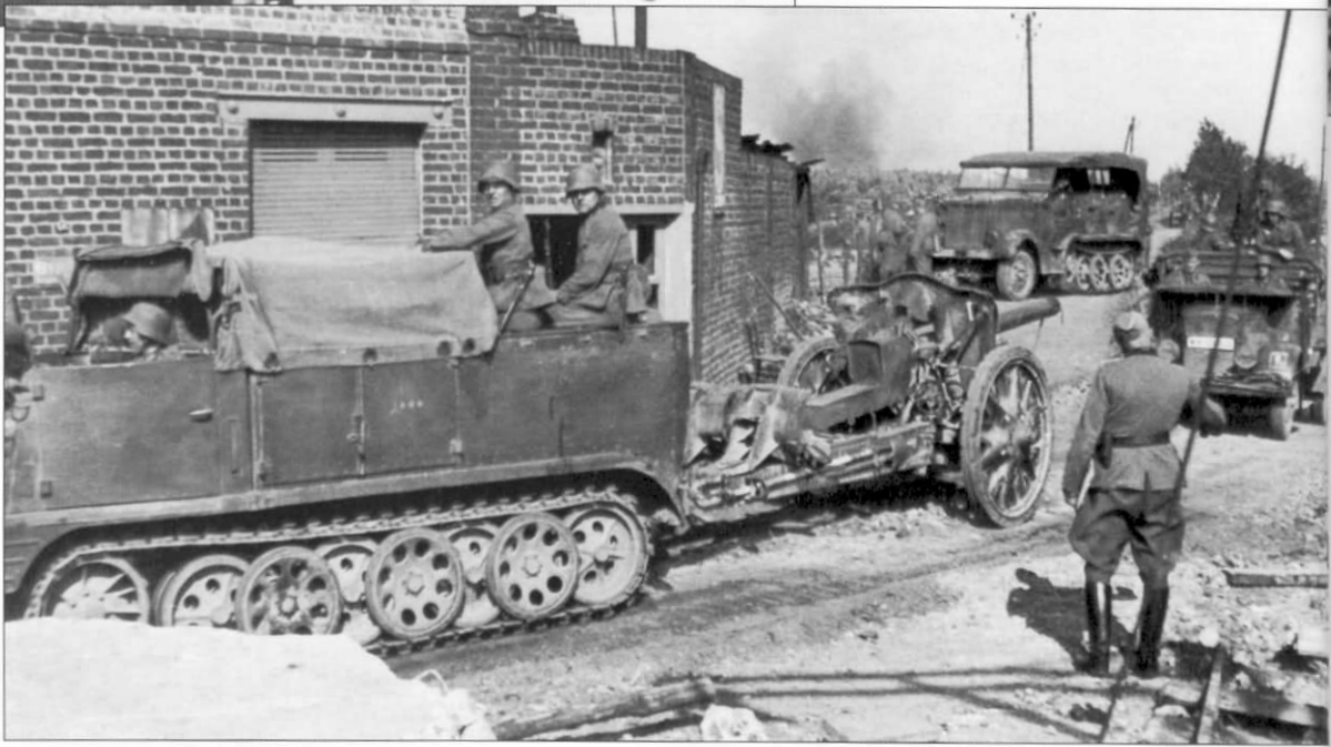
An Sd.Kfz.11 halftrack displaying the 7.Panzer-Division symbol on its stowage locker door tows a 10.5cm leFH 18 through a destroyed French town, possibly Le Bassee. Behind it is a 3-ton truck with its license plate mounted in an unusual position on the radiator grille. The 5-ton halftrack in the background is the engineer's version of the Sd.Kfz.6.
