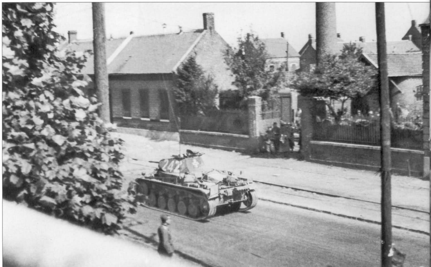
A Pz.Kpfw.II Ausf.A-C moves quickly down a French street in a town that appears untouched by the effects of war. From the style and color of the turret numbers, this vehicle is probably from 7.Panzer-Division as this was one of the only units to display this style. A prominent black and white cross is on the turret rear. Note that the crew has been careful to leave the white aerial recognition rectangle on the engine deck unobstructed.
