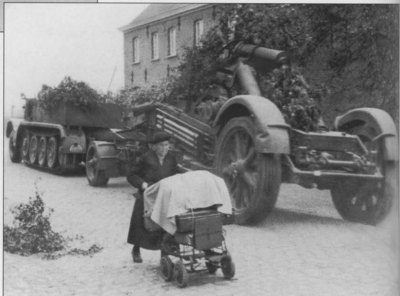
German heavy artillery on the move during Fall Rot. While many artillery units were still using horse power, the panzer divisions were equipped with mechanized units to allow them to keep pace with the advance. Halftracks were the most common form of motive power for the heavy artillery pieces such as those seen in these two photographs. The first picture is an 8-ton Sd.Kfz.7 towing a 15cm sFH 18 (heavy field howitzer 18), the most common large caliber piece in the Wehrmacht's inventory.
