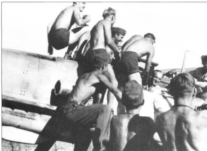
Groundcrew swarm over the F-4/trop (note mounting holes for the absent dust filter immediately below the gun trough) of Hauptmann Wolfgang Ewald. This photograph was reportedly taken in July 1942, although the reason for the obvious excitement remains unknown - unless perhaps it is the announcement of Ewald's appointment as Kommandeur of III./JG 3 (he replaced Major Karl-Heinz Greisert, who was killed in action against I-16s on 22 July)
