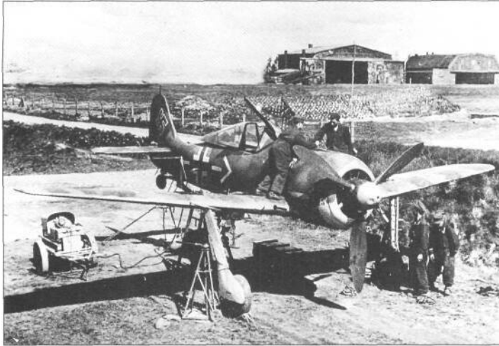
The Geschwaderkommodore's machine undergoes gun calibration following routine servicing away from the frontline at Dorpat, in Estonia, on 18 July 1944. Major Anton Mader's Fw 190A-6 wears a white command chevron and bars, as per regulations. The scheme worn by the A-6 is typical of that adopted by the recces assets of Luftflotte I in the northern sector of the front, and consisted of an upper surface camouflage pattern of green and brown
