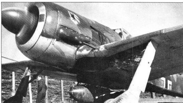
A bomb-carrying Fw 190 seen in the spring of 1943. The weapon mounted to the centreline ventral stores rack is an SB 500 kg High Explosive (HE) bomb. This type of weapon was the favoured ordnance for the Gruppe on the Russian Front, although a single SB 1000 kg bomb could also be carried, as well as smaller 250 and multiple 50 kg devices
