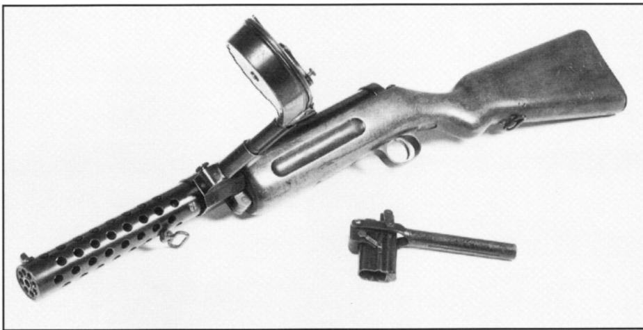
The MP18 was one of the first sub-machine guns to be used in action. Note the 32-round 'snail' magazine, developed for the Artillery Model Luger, and its loading tool. The magazine affects the balance of the MP18, canting the weapon sharply to the left even when empty. (Pattern Room Collection)
