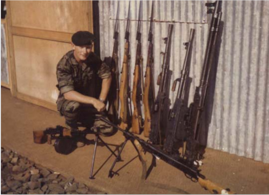
A display of enemy weapons captured on missions. Against the wall, from left to right, are: four 7.62mm Type 53 (M1944) carbines, two 7.62mm SG-43 machine guns, and a 12.7mm DShKM 1938/46 machine gun. At the front are a 7.62mm RPD light machine gun to the left and a 7.62mm DP light machine gun to the right. (James Bolen via Steve Sherman)
