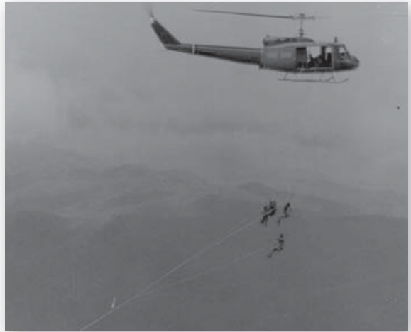
Four men of RT Marine of CCN are lifted out by a McGuire-rig extraction system fitted to a 57th Aviation Company UH-1H. The men could not be hoisted into the helicopter, but had to ride below it. (Frank Greco via John Plaster)
