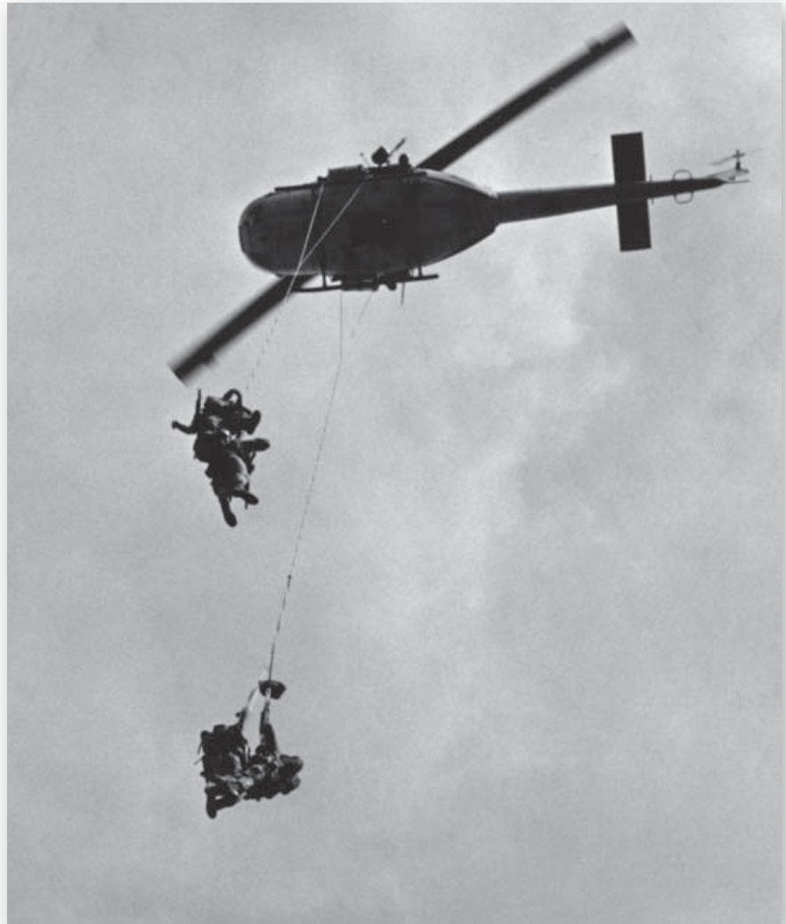
A UH-1H Huey extracts an RT during training using STABO rigs. This was a harness arrangement incorporated into the recon man's web gear in lieu of load-bearing equipment suspenders. A Special Forces NCO and two officers developed the system in 1969 at the MACV Recondo School. (Dale Boswell via John Plaster)
