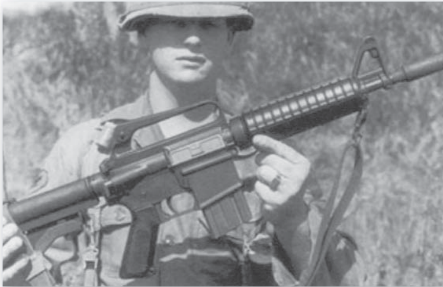
The 5.56mm XM177E2 submachine gun was issued to many recon teams. Its compact design was ideal for use by LRP. This is a 20-round magazine. Curved 30-round magazines were extremely rare. (US Army)
