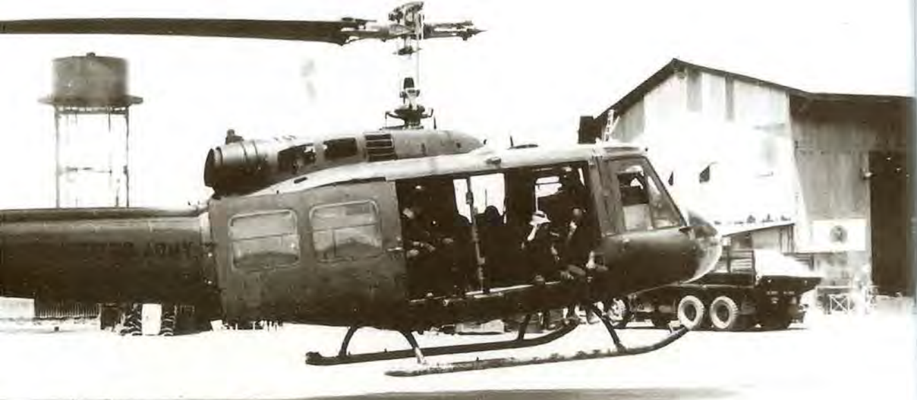
A UH-1H "slick" with the troop compartment doors locked open. It is in ground effect, hovering as it taxis to its takeoff position. (Leroy "Red" Wilson)
