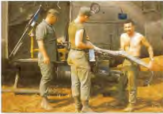
Ground crewmen prepare a machine-gun flexible ammunition chute for loading aboard a UH-1B gunship. the door gun is a 7.62mm M60D.
