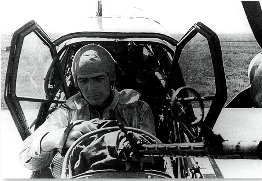
A Bf110 operator/gunner preparing his single MG15 for action; ten 75-round double-drum magazines were carried. Rear armament was progressively improved to twin MGs, but was never adequate.
