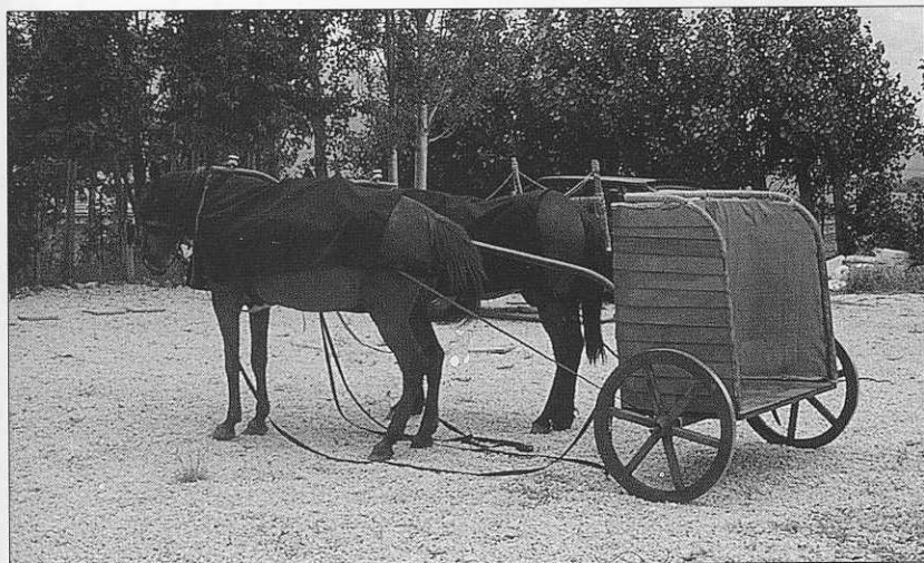
Hittite chariot, reconstructed. Chariots had to be light enough to ensure speed and manoeuvrability in battle, but also sufficiently robust to carry three warriors, and endure the rigours of a long campaigning season.
