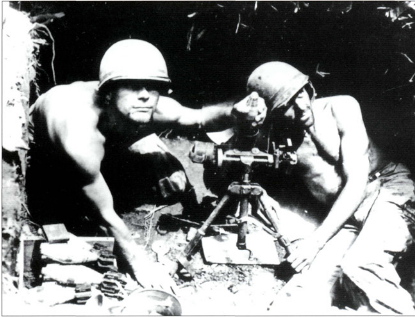
The small M2 60mm mortar, like this one in a deeply entrenched firing position on Bougainville, was the fire-support weapon at company level. It could fire HE, smoke, and illumination rounds. (USMCRC)
