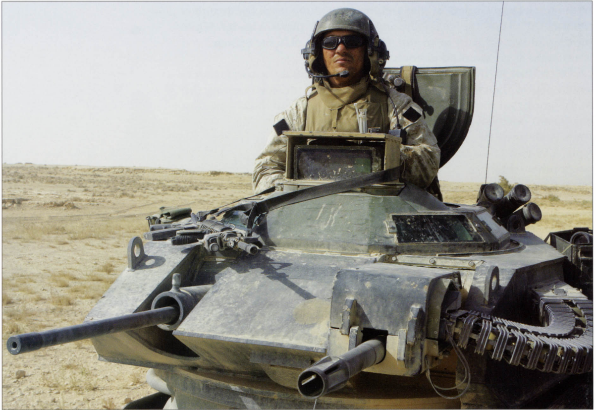
ABOVE A small electric turret, or “up-gun” perched above a Marine AMTRAC houses a .50 cal. machine gun and a MK19 automatic grenade launcher. The track commander typically mans the up-gun. (Photo courtesy USMC)
