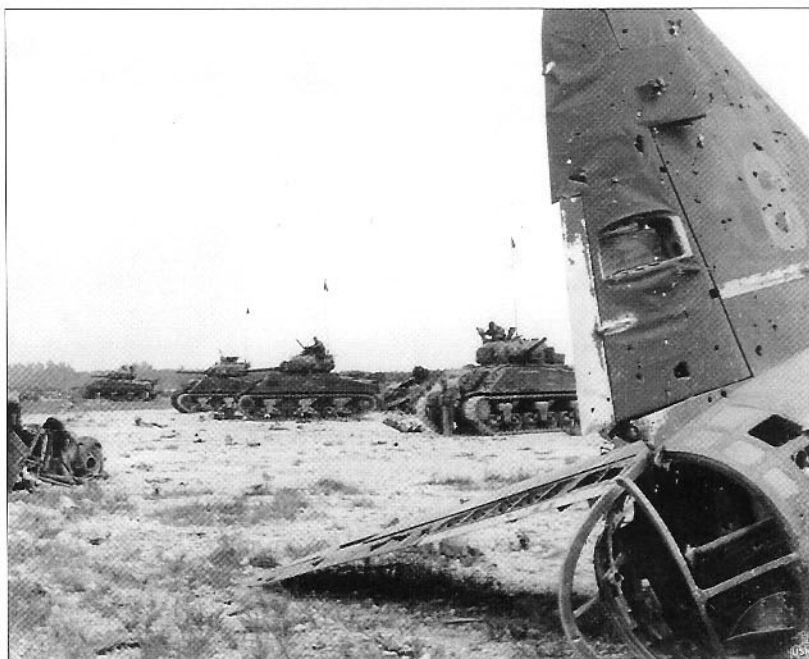
M4A2 tanks of A Company, 1st Tank Battalion, form on the middle of the airfield at Peleliu, after the defeat of the ineffectual Japanese tank charge there. The unusual display of pennants on the radio antennae demonstrates how little Marine Corps tankers feared Japanese antitank guns at this point in the war, although track blocks are mounted on turret sides and hull front as extra protection. (USMC photo)
