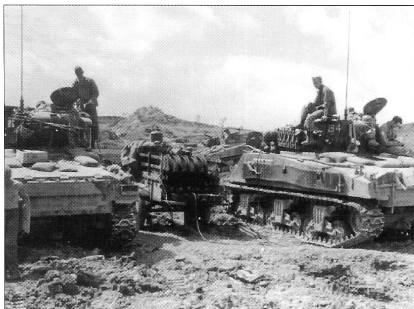
Two crews of B Company, 1st Tank Battalion, are using a lubrication unit during a lull in the Battle of Okinawa. This battalion worked against the supply "system" and was able to keep their late-model twin-diesel M4A2 tanks through the end of the war. (USMC photo)
