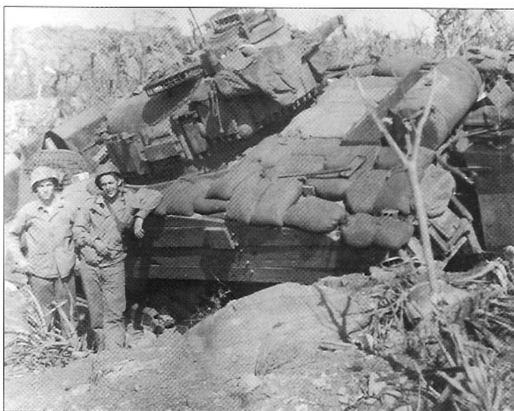
These tankers of C Company, 4th Tank Battalion, on Iwo Jima have a hard day's work ahead, digging out their bogged dozer tank. Note the improvised protection: timber sides, sandbags over the engine armor, and birdcage hatch covers. The cylindrical light tank auxiliary fuel cell was filled with water for distribution to the infantry they supported. (Author collection)
