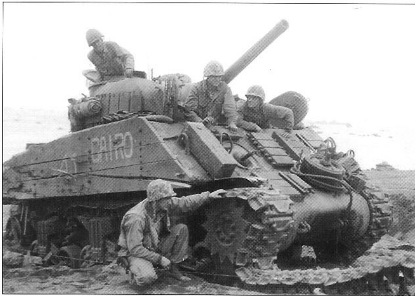
Another view of a tank of C Company, 4th Tank Battalion, on Iwo, showing how the wood planks supported a 4in. layer of reinforced concrete, making the tank proof against the Japanese 47mm antitank gun on the side. Everybody wore helmets, even in the rear area, because the Japanese artillery and mortars covered the entire island. (USMC photo)
