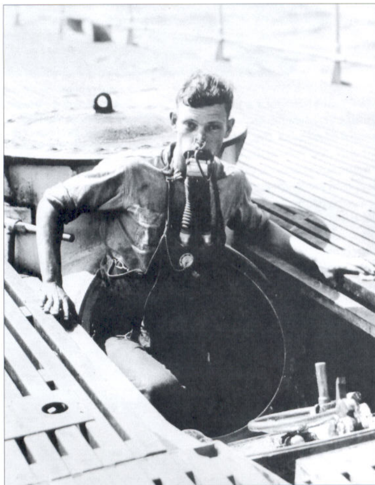
A crewman demonstrates the proper method of wearing the Momsen Lung as he moves from the aft escape trunk in this prewar photograph. (US Navy Photograph)
