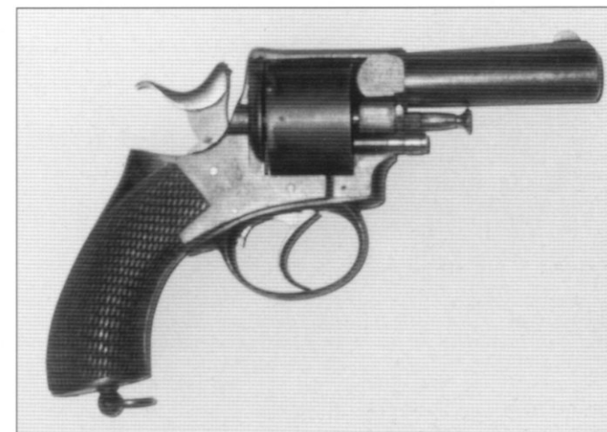
The .450 double-action Webley revolver pictured here was one of many Volunteer weapons captured from the British security forces. A variant of the earlier .442 RIC model, this revolver was manufactured around 1872. (Captain Tom O'Neill's collection)
