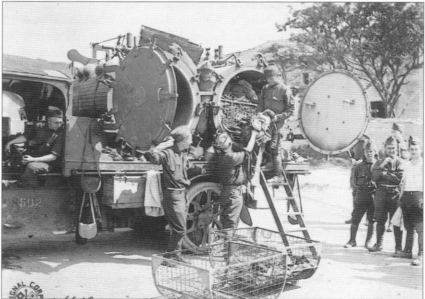
The "cootie" truck. Clothing would be put into the chambers and heated and fumigated in an effort to kill the seam squirrels, i.e. "cooties" or lice.
