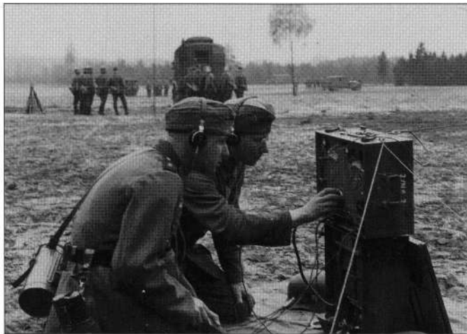
Signallers get on net during a halt in the advance. The radio is a T FuG k used by the artillery with a weight of 45 pounds. Its aerial lies to the right of the photograph, probably in the best position to send and receive in this location.
