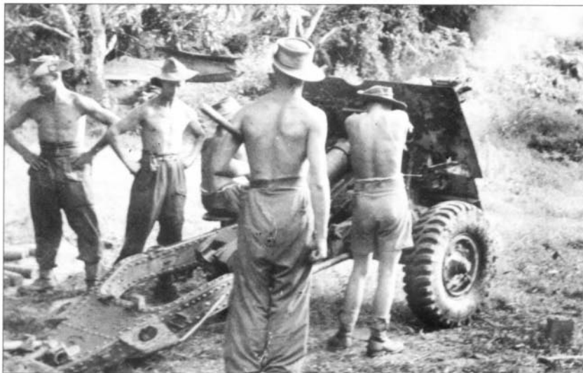
25-pdr in action. The 25-pdr was developed during the 1930s and was in production by 1940. It could fire high- explosive, smoke and armour-piercing shells. These guns were also modified for the jungle by shortening the axle length in order to improve movement. (courtesy of the Trustees of the Imperial War Museum)
