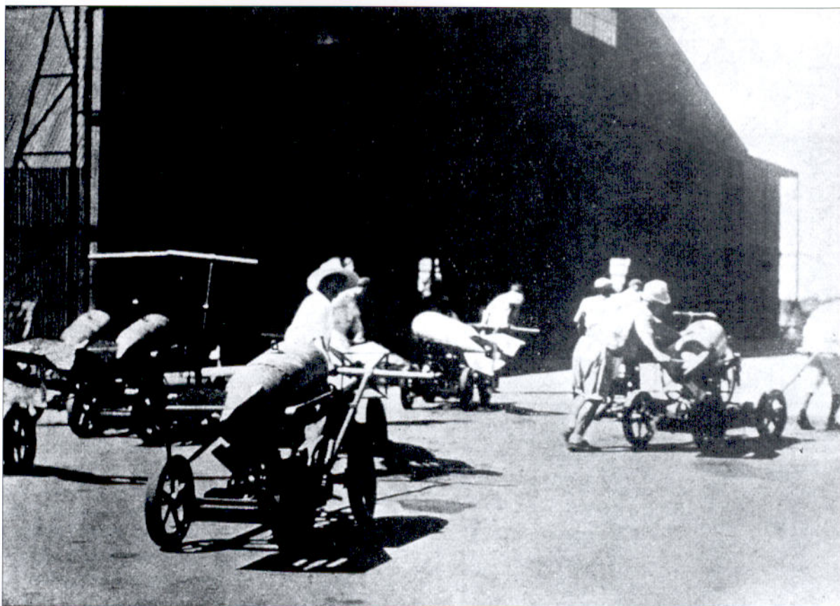
Heavier items of ordnance, such as these 250kg bombs, were carried on dollies. (via Edward M. Young)
