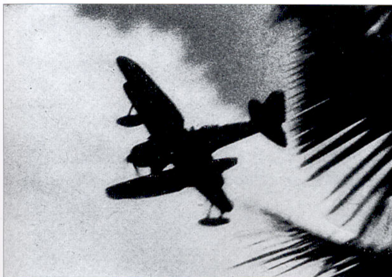
A Type 0 Observation Seaplane (F1M) takes off on a mission over the Solomon Islands. Despite its obsolete biplane configuration and cumbersome floats, the F1M performed a great service for the IJN in the South Pacific.
