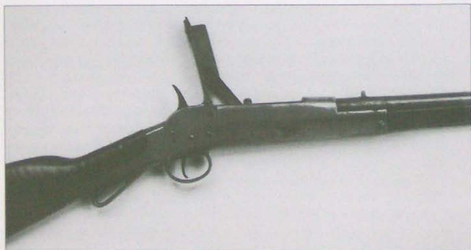
The 0.50-caliber metallic center-fire cartridge required by this Morse Carbine, made by the Greenville Military Works for South Carolina's militia, was difficult to produce in the South, making the value of this weapon somewhat limited. (Russ Pritchard collection)
