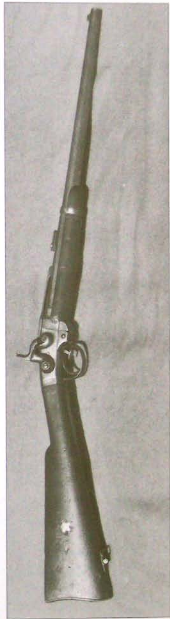
The patented Smith carbine was a US Army weapon that used a rubber cartridge which fitted into a breech that broke open. These cartridges could be refilled and used time and again, so they were useful when captured by Confederate troopers. (Chris Nelson collection)
