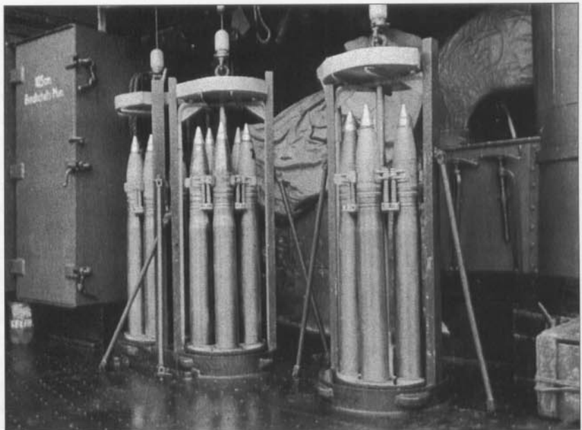
The 10.5 cm shells for the twin anti-aircraft mounts on Bismarck/Tirpitz class ships were stored below decks and brought up to the guns in special cradles via elevator shafts. This saved a huge amount of hard, physical effort for the crewmen. These modern battleships had many novel features that made life aboard much easier for the crews. (Naval Historical Center)
