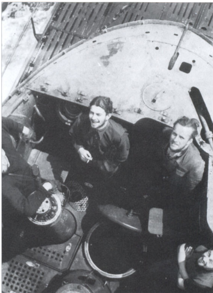
A view down into the bridge area of a Type IX U-boat. Note the extremely small open hatch through which the entire bridge watch would have to disappear in a matter of seconds in case of an alarm call from one of the look-outs. The object on which the left-hand crewman is resting his arm is the base of the UZO apparatus.
