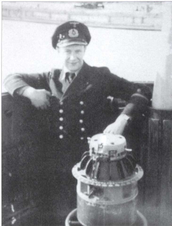
The LI of U-595 , Leutnant Emmerich Freiherr von Mirbach, on the bridge of his boat in Gotenhafen harbour, 1941. In front of him is the mount for the UZO apparatus, and at his left elbow is the navigation or 'sky' periscope.
