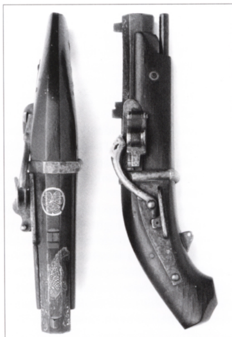
This Japanese arquebus has an external brass spring. The trigger releases the serpentine, which drops the glowing match onto the touch hole. A brass cover protects the firing pan. The barrel is fitted with a backsight and a foresight. Note the short stock, the weapon would be hand-held rather than rested on the shoulder.
