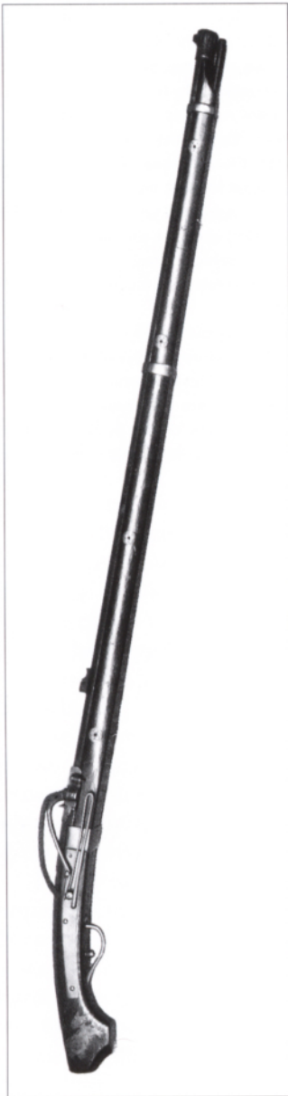
This Japanese arquebus has an external brass spring. The trigger releases the serpentine, which drops the glowing match onto the touch hole. A brass cover protects the firing pan. The barrel is fitted with a backsight and a foresight. Note the short stock, the weapon would be hand-held rather than rested on the shoulder.
