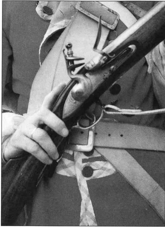
ABOVE Short land pattern firelock: lock detail – flash pan open. [Author's collection]
