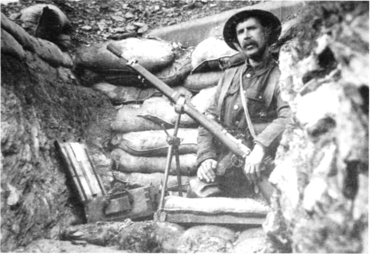
An unusual photograph of a rifle-grenade pit. The SMLE rifle has a Hales grenade inserted into the barrel. An adjustable bipod permits the weapon to be fired at the required angle. Few grenade-launching rifles were used for any other purpose, as firing rodded-grenades soon ruined barrels. The practical effect of such grenades was probably minimal, although the moral effect was useful. (Private collection)
