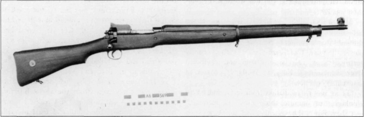
The Pattern 1914 rifle was based on the Mauser action, and originally chambered for a .276 in. (7 mm) cartridge, an extremely powerful round. The demands of war in 1914 showed the difficulties of mass producing the SMLE. The P14 was easier and cheaper to make and was rapidly converted to .303 in. Fitted with a telescopic sight, it made an excellent sniping rifle. (Trustees of Royal Armouries)
