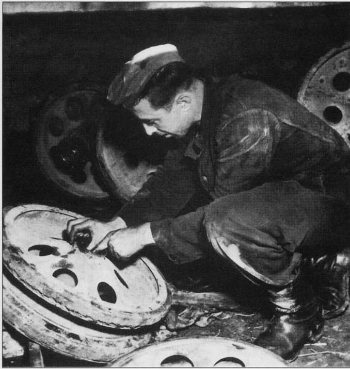
A German mechanic services the roadwheels of an Sd.Kfz.251 at night. 4.Panzer-Division suffered most of its losses due to mechanical breakdowns and not to enemy fire, which placed a great strain on the service battalion to keep the vehicles of the Division in running condition. Note how badly worn the rubber tire is on the outside rim of the wheel.
