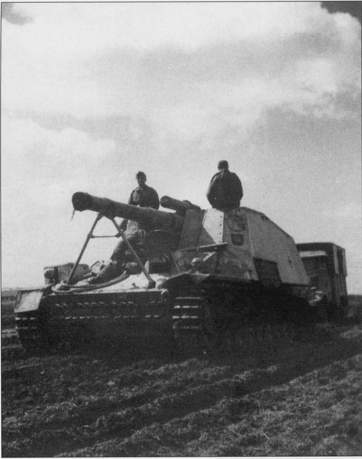
An Sd.Kfz.165 'Hummel' heavy self-propelled howitzer armed with the 15cm sFH18 of Pz.Art.Rgt.103 towing a truck through a muddy field. This is an early production series vehicle with the raised compartment for the driver only. Later vehicles had a full width, simplified superstructure. It has a coat of white winter camouflage paint over its dark sand base and has the Divisional emblem painted on the side of the fighting compartment and a large letter 'G', indicating the seventh gun in the battery, probably painted in red.
