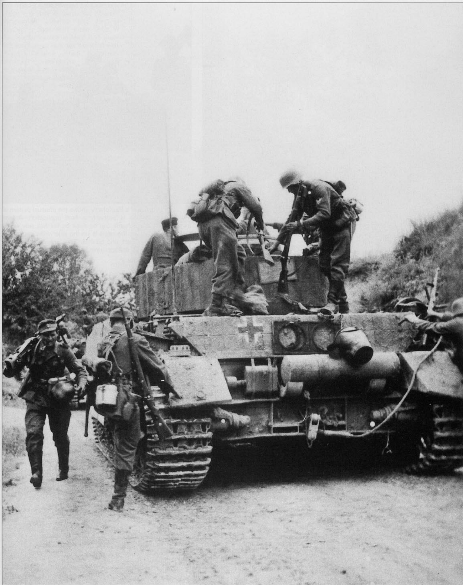
An infantry squad climb aboard a Pz.Kpfw.IV Ausf.H fitted with the wide 'Ostketten' and covered with a heavy application of Zimmerit. In the middle of June, 4.Panzer-Division finally received its 'Panther' Abteilung. The original I./Pz.Rgt.35, equipped with Pz.Kpfw.IV, was renamed II./Pz.Rgt.35. However, changing the numbering of the tanks did not happen immediately and so the Pz.Kpfw.IV continued to use their tactical numbering system starting with the numbers 1-4.
