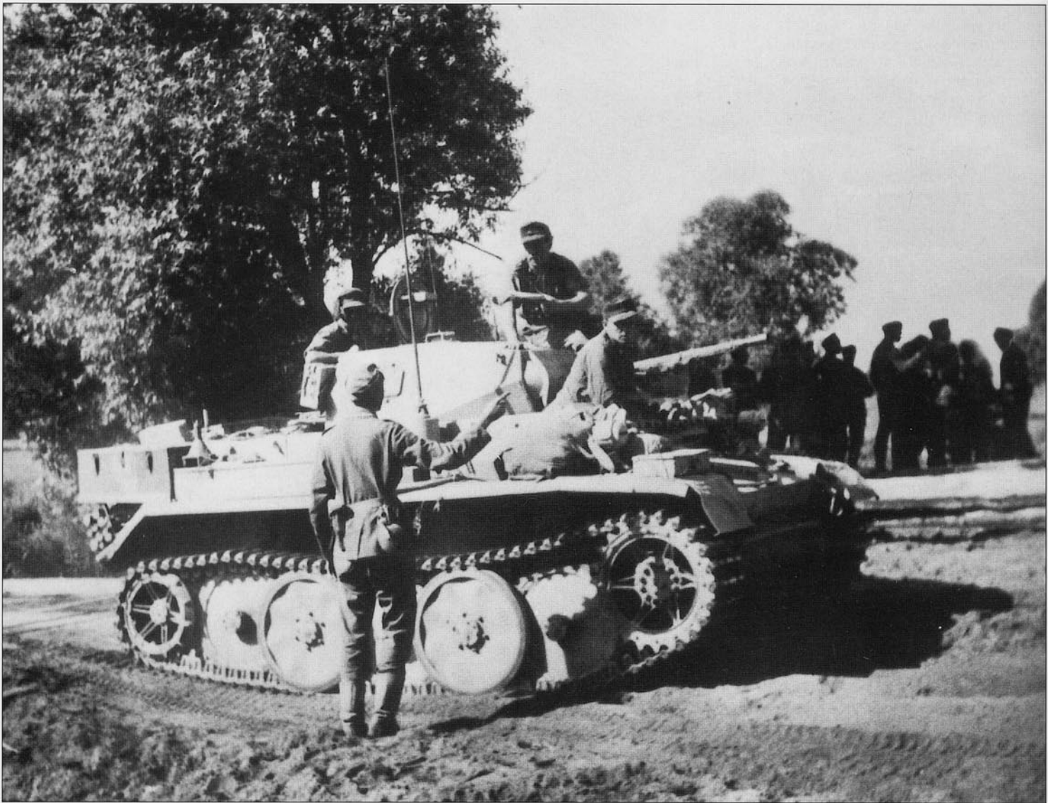
This Pz.Kpfw.II Ausf.L 'Luchs' is one of the later production vehicles received by Pz.Aufkl.Abt.4. Note the amount of loose equipment stored on the vehicle and the additional storage box mounted on the rear of the mudguard by the Division workshop. The object sitting in front of it is a 3kg hollow-charge anti-tank mine.
