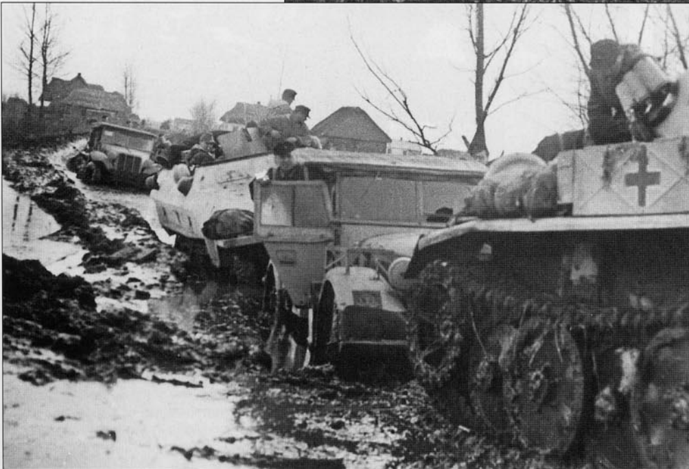
The mild weather at the end of December turned the roads into a morass which made offensive operations extremely difficult to carry out. Here we see a Pz.Kpfw.II Ausf.L 'Luchs' preparing to tow a Horch cross country car that has bogged down on a muddy village road. Behind this can be seen an Sd.Kfz.251/1 Ausf.D and an Sd.Kfz.10, also struggling with the poor conditions. The Sd.Kfz.251 appears to have received a new coat of white winter camouflage paint while the other vehicles still appear to be painted in their dark sand base color. The new Divisional emblem can be seen on the mudguard of the Horch.
