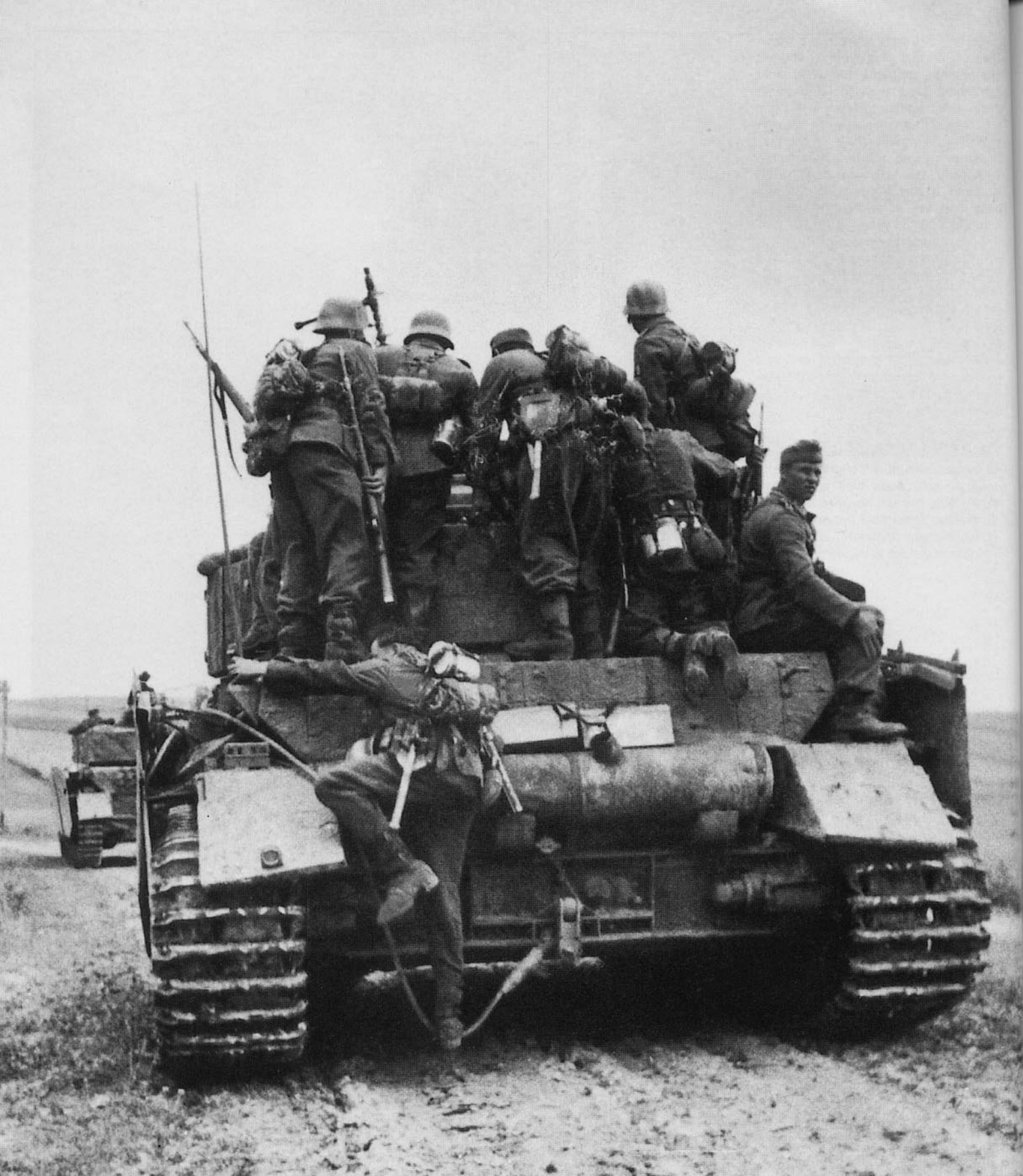
Another MG34 team climb aboard a Pz.Kpfw.IV Ausf.H that has also been equipped with the wider 'Ostkette'. The side skirt plates were fitted with an adjustable lower bracket that pushed the bottom out to provide the additional space required by these wider tracks. This tank has a heavy coat of field applied Zimmerit as well.
