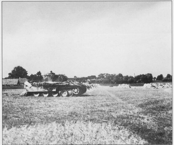
This Pz.Kpfw.V 'Panther' Ausf.G of I./Pz.Rgt.35 has been camouflaged with cut foliage and some bundles of straw picked up from the field. Two of the vehicle's side skirt plates are missing, a frequent occurrence when traveling through forested areas. Other than the conspicuous national cross on the front of the hull, no other markings are visible. During the whole month of August, 1944, 4.Panzer-Division claimed to have destroyed 240 tanks, 7 SPG's and 204 enemy guns.
