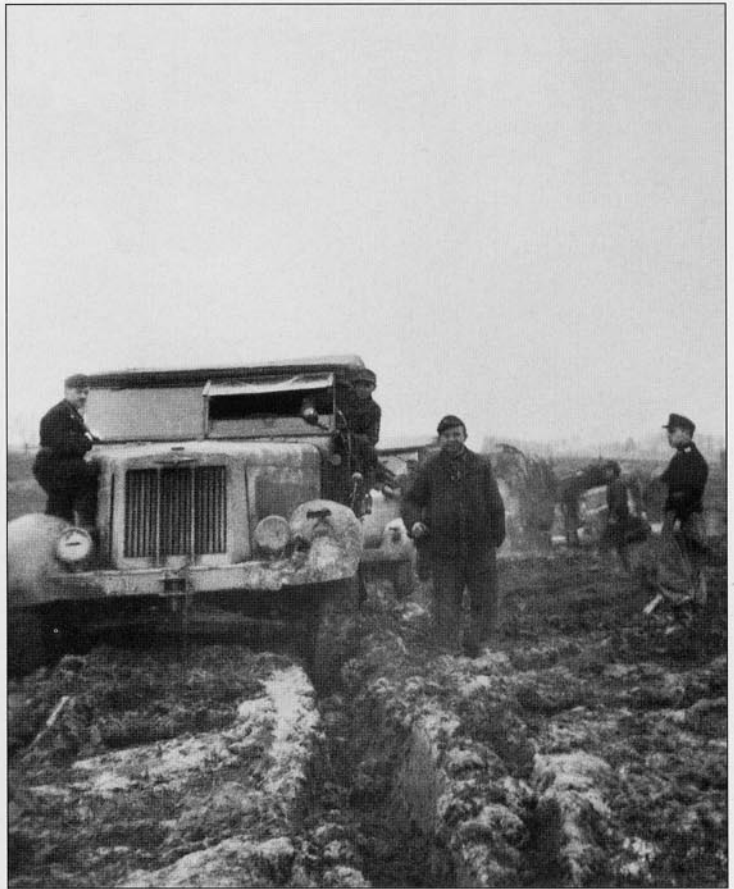
The wet, autumn weather in Kurland produced the same results as it did in the Soviet Union. Even powerful vehicles such as this Sd.Kfz.7 half-tracked prime mover, seen towing a truck, had trouble negotiating a path through the muddy fields. Conditions such as this greatly hindered offensive operations.
