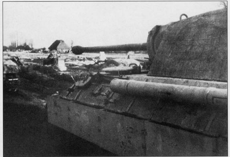
Another view along the same road. This 'Panther' Ausf.A does not have a tactical number painted on the side of the turret but has, what appears to be, a shipping stencil on the gun cleaning rod tube and a national cross on the front hull side. The Zimmerit coating is quite clear in this photo.
