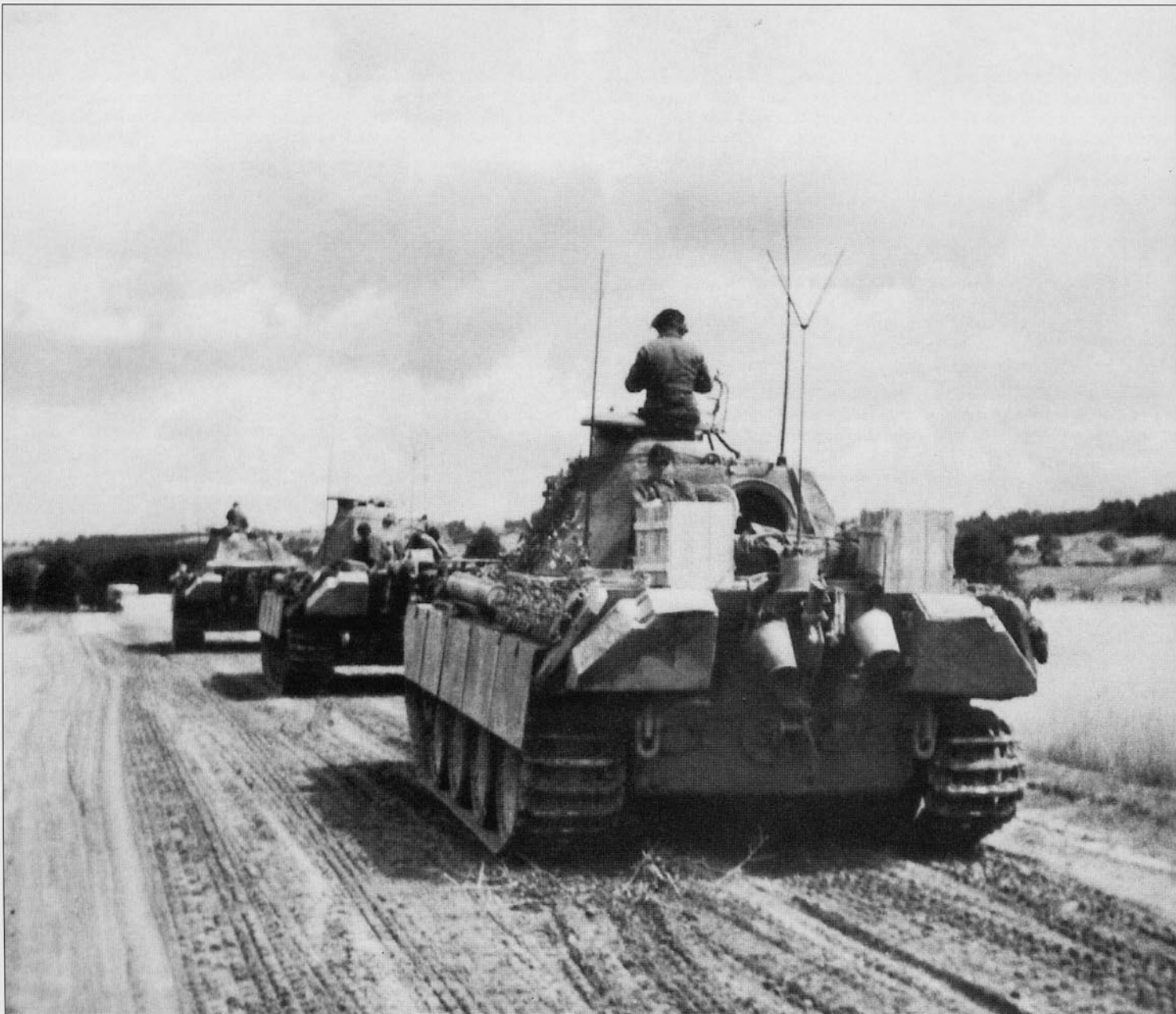
Two Pz.Bef.Wg.V 'Panther' Ausf.G follow a standard combat version past a grain field in the summer of 1944. The three antenna on each vehicle can be seen including the characteristic star antenna for the FuG8 radio set.
