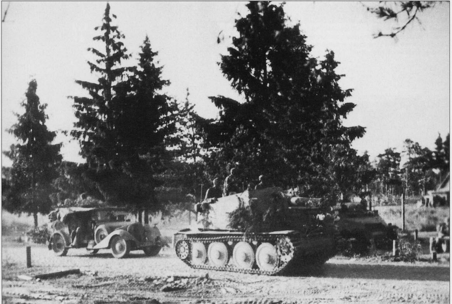
A 15cm sIG33 Ausf.H 'Grille' self-propelled howitzer, constructed on the chassis of the Pz.Kpfw.38(t), of Pz.Art.Abt.103 followed by an old Horch 830 B1 light cross country car. In the background, just in front of the 'Grille', an Sd.Kfz.251 can be seen.
