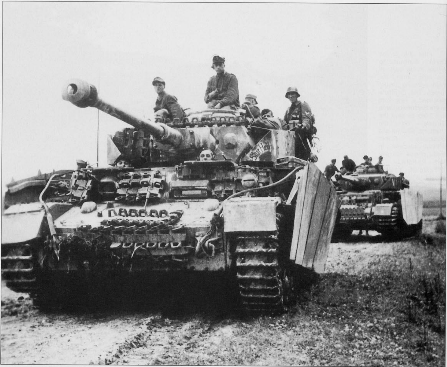
Two Pz.Kpfw.IV carrying infantry in western Belorussia around July 10, 1944. The lead vehicle is the same one seen in the previous photo and has been well protected with the addition of spare track links around the front of the hull and turret. It also has the words 'Stur Heil', the meaning of which is not clear, painted on the front of the turret skirt. Note how the side skirts are hanging on the vehicle in the background, which has been fitted with 'Ostketten', compared with the vehicle in the foreground which is fitted with standard tracks.
