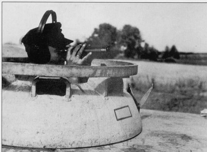
The details of the cupola can be seen clearly in this photo of a 'Panther' commander as he views the terrain ahead through his field glasses. The significance of the rectangle painted below the episcope is unknown.
