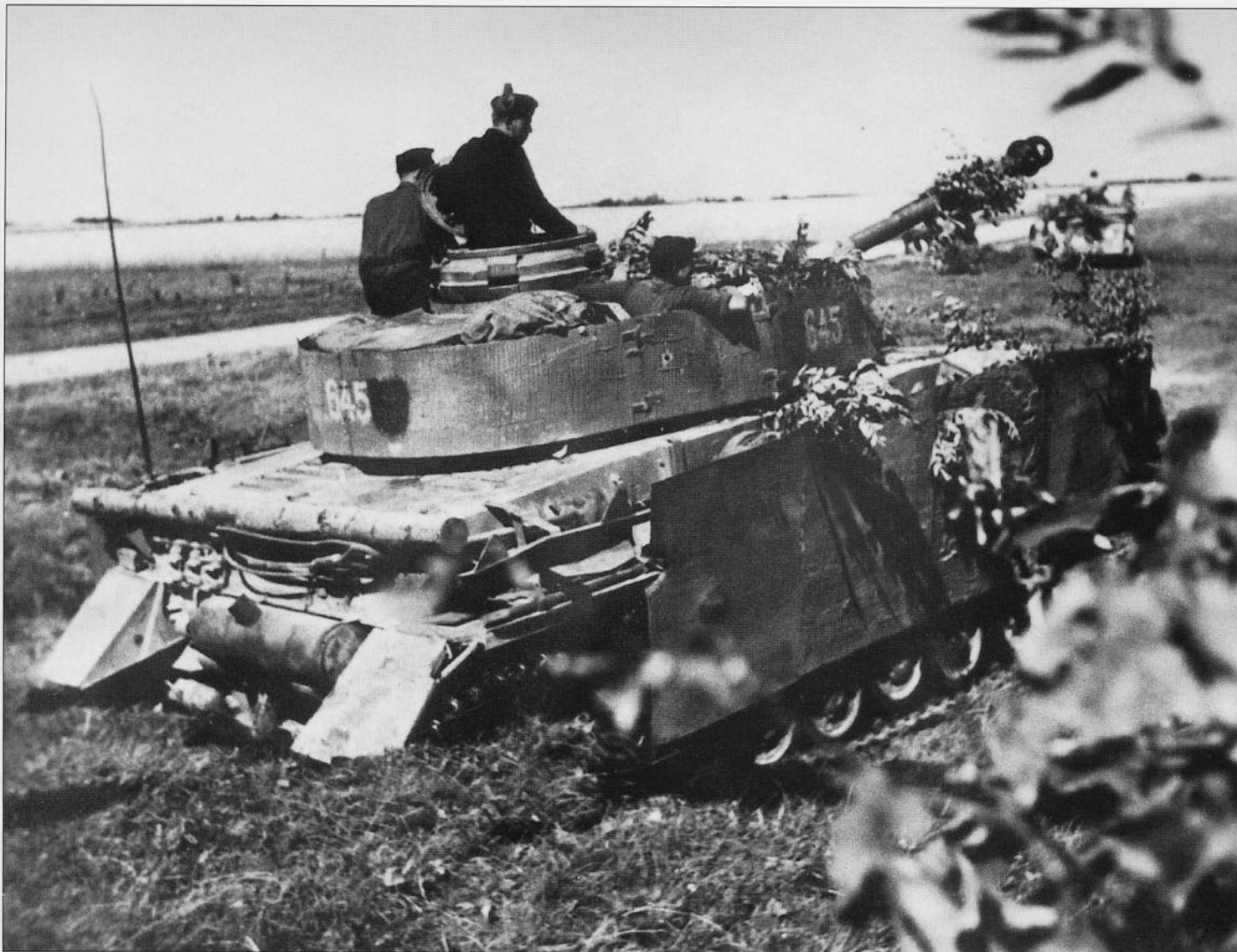
II./Pz.Rgt.35 played a minor role in the later battles in Kurland. This was due to the high rate of attrition as a result of breakdowns among the Pz.Kpfw.IV's employed in this battalion. There were instances when up to 75% of the vehicles available were unserviceable after long marches. The tactical number '645' is painted on the turret skirt in white and the Divisional emblem is also visible. The marking in front of the tactical number on the side is probably the Regimental standing bear emblem painted in red or black. Note the large hole in the rear edge of the side skirts, where an anti-tank round has exploded, preventing a potentially fatal hit on the tank. This is a Pz.Kpfw.IV Ausf.H.
