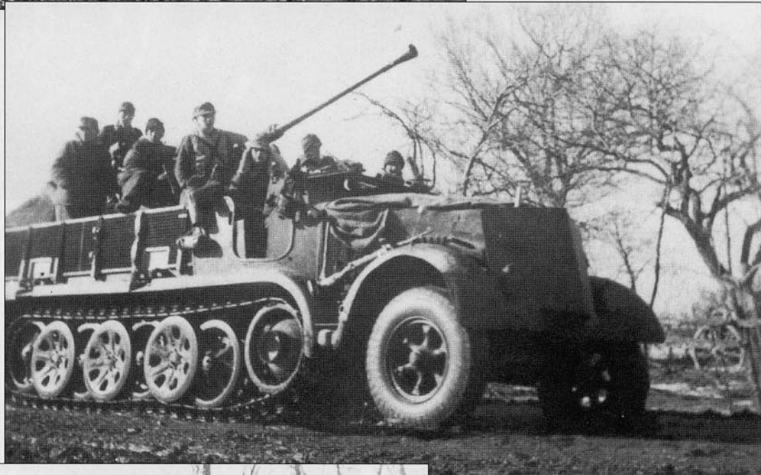
An Sd.Kfz.7/2 armed with the 3.7cm FlaK36 anti-aircraft gun of Flak.Art.Abt.71 traveling through a Soviet village in the winter of 1943/44. The vehicle is fitted with an armor plate to protect the radiator but is lacking the armored cab. It appears to be painted in its original dark gray paint.
