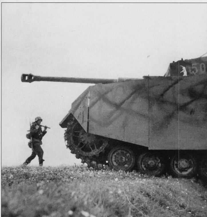
Another shot of the same tank showing the hastily applied camouflage paint on the side skirts. This style was common on many of the Pz.Kpfw.IV Ausf.H utilized by the Division at this time.
