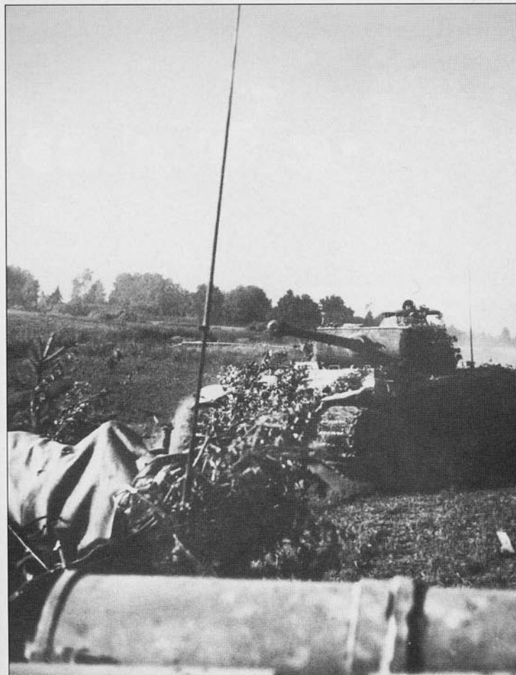
A 'Panther' Ausf.A kicks up a cloud of dust as it catches up with the rest of the platoon. The object in the foreground is the gun cleaning rod tube mounted on the rear of the engine deck of another 'Panther'. The antenna that is visible just behind is actually mounted on an Sd.Kfz.250/3 parked next to it.
