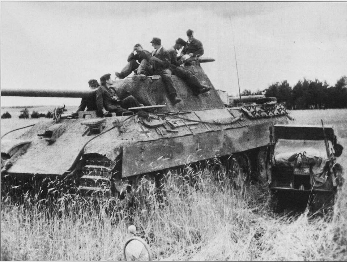
The driver of this Kfz.2 Kettenkrad has brought mail from home to one of the crew members of this Pz.Kpfw.V 'Panther' Ausf.A. Tow cables have been attached to the front tow hooks so that they can be quickly utilized if needed. On July 8 and 9, there were 4 Pz.Kpfw.IV and 10 'Panthers' out of service due to damage and breakdowns. The crew has removed the gun cleaning rod tube to the rear of the engine deck, typical for 'Panthers' of this unit. Note the small puppy on the glacis just above the MG ball mount.
