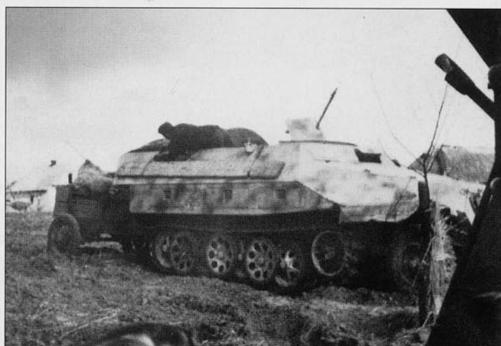
An Sd.Kfz.251/1 Ausf.D as viewed through the open rear doors of an earlier Ausf.C. It has a camouflage paint scheme of green or brown applied over the dark sand base and is towing a small trailer of Soviet origin. It is also armed with an MG34 in place of the MG42 usually carried by these later vehicles.
