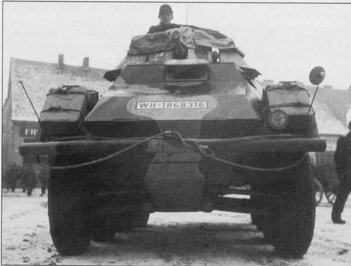
Three views of a new Schwerer Panzerspähwagen (2cm) (Sd.Kfz.234/1), which replaced the Pz.Kpfw.II Ausf.L 'Luchs' as the main combat vehicle of Pz.Aufkl.Abt.4. This photo is taken in January 1945 in the area of Danzig (Gdansk). The vehicle has been painted with a hard edge camouflage scheme of green and brown irregular patches over the dark sand base, applied using a brush. There are no visible markings other than the vehicle license number, WH-1868316, painted on the front and rear plate and a small national cross painted on the side of the turret.
