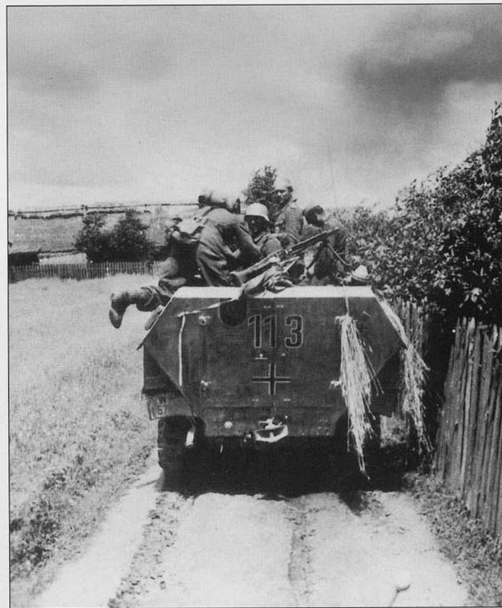
A Panzer-Grenadiere climbs into his Sd.Kfz.251/1 Ausf.D half-track on a dirt lane in a Polish village. Even though the vehicle has rear doors, it was often easier to climb over the side because of the amount of equipment stowed in the interior. This vehicle has the tactical number '113' painted in black with a white outline on the rear along with the Divisional emblem and a narrow national cross. The '1's in the tactical number are unusual in that the white outline on the left side of the vertical bar extends up through the diagonal tail. Also visible just to the right of the bundle of straw is a small black Iron Cross outlined in white, symbolic of the Knight's Cross awarded to the Regimental commander.
