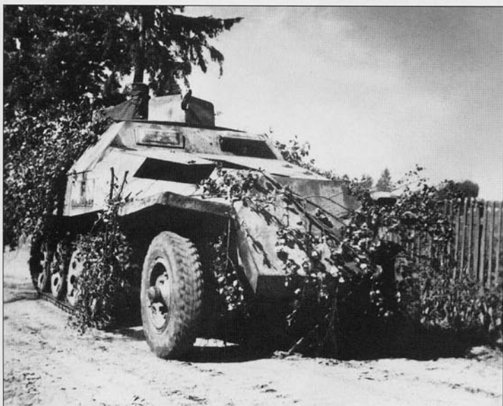
An Sd.Kfz.251/1 Ausf.D traveling down a road through a village after the battle. The markings on the front of the vehicle have been overpainted with a light color by the crew as they tended to compromise the camouflage of the vehicle and provided an aiming point for enemy gunners.
