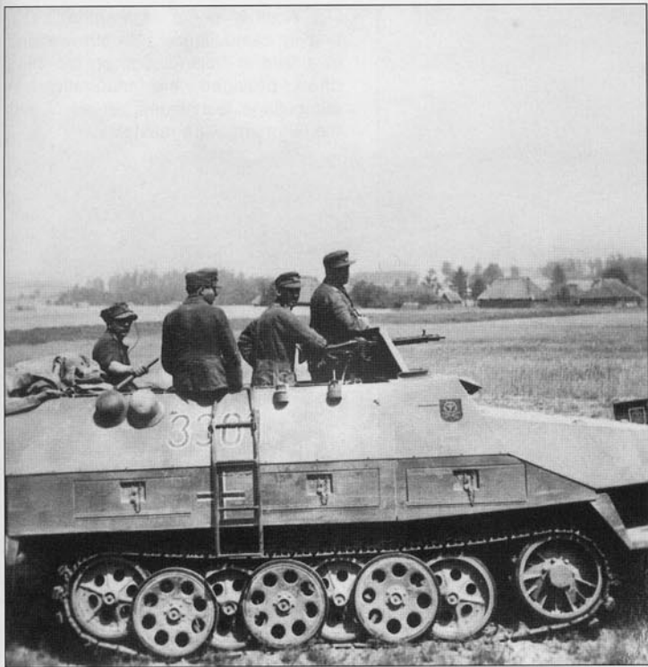
Command half-track of Pz.Gren.Rgt.33 with the Regimental commander, Oberst von Gaudecker, standing in front. This Sd.Kfz.251 Ausf.D has been field modified from its original form to serve as a radio command vehicle. There are two antenna bases on the right side and the crewman in the rear is wearing radio headphones, but there are no visible antenna. The tactical number '3301' is painted in black with a white outline and indicates this to be the command vehicle of Panzer-Grenadier-Regiment 33. The Regimental command flag is carried on the left mudguard and is black with a green stripe and has the Divisional emblem painted on it along with an Iron Cross emblem symbolizing the Knight's Cross won by Oberst von Gaudecker. On the right side of the driver's compartment, the Divisional emblem is repeated along with a faint tactical sign for a Panzer-Grenadier-Regiment below it.
