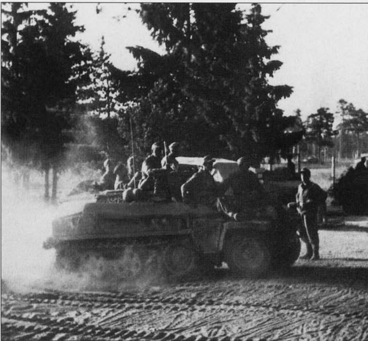
Many of the battles against the Soviets in Kurland in 1944 were conducted by small battlegroups called Kampfgruppen. Kampfgruppe Christern was formed on Pz.Rgt.35 and included Pz.Aufkl.Abt.4 under Hptm. Moler. Here we see one of their vehicles, an Sd.Kfz.250/1, one of the older models that has been modified with the addition of storage compartments over the mudguards which gave it a similar appearance to the later 'Neu' version.
