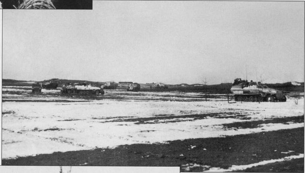
Several half-tracks from Pz.Gren.Rgt.12 or Pz.Gren.Rgt.33 crossing a field in the area of Kovel. On the right is an older model Sd.Kfz.251/3 Ausf.C radio vehicle of the battalion or company staff. On the left is an Sd.Kfz.10 and in the background is an Sd.Kfz.251/9 Ausf.D, armed with a 7.5cm KwK37 (L/24) howitzer. Two of the vehicles appear to have fairly new coats of white winter camouflage paint.
