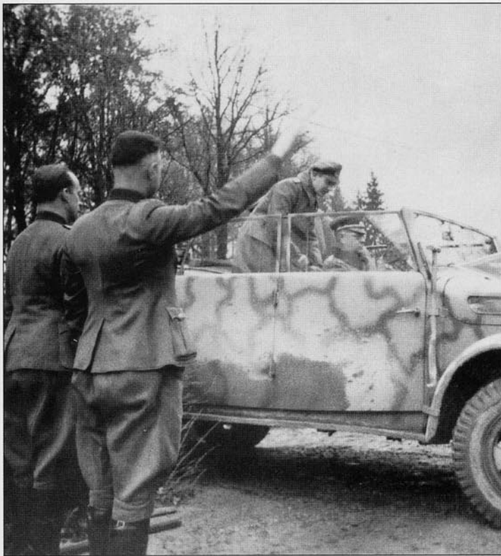
4. Panzer-Division staff officers salute an unidentified General visiting the front in his Steyr 1500A staff car. It has an interesting camouflage scheme of green, wavy lines over the dark sand base, partly obscured by both old and new mud.
