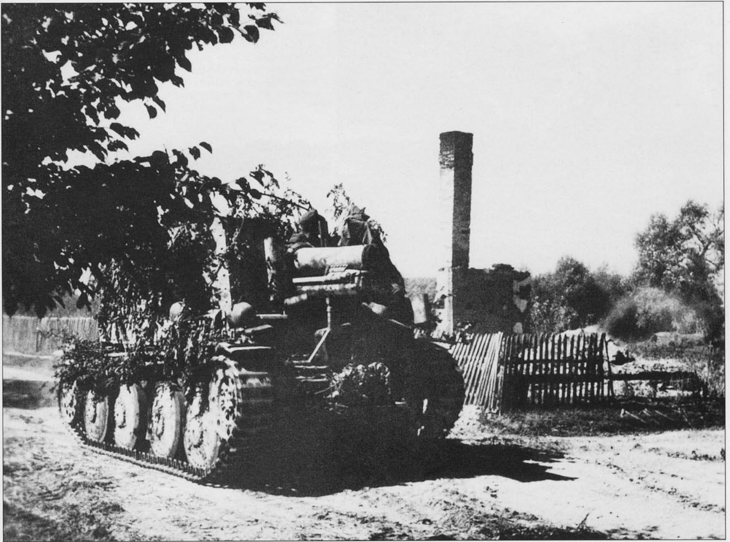
The Panzer-Grenadier Regiments had their own artillery support provided by a six gun battery of 15cm sIG33 Ausf.H or Ausf.M 'Grille' self-propelled guns built on the Pz.Kpfw.38(t) tank chassis. Most of the guns used by Pz.Gren.Rgt.12 and 33 were of the Ausf.H type.
