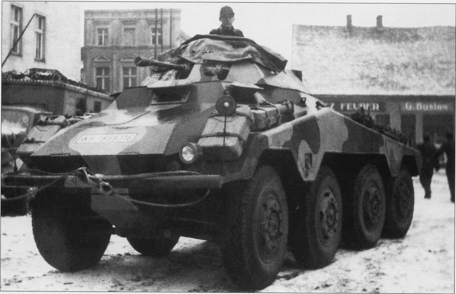
Three views of a new Schwerer Panzerspähwagen (2cm) (Sd.Kfz.234/1), which replaced the Pz.Kpfw.II Ausf.L 'Luchs' as the main combat vehicle of Pz.Aufkl.Abt.4. This photo is taken in January 1945 in the area of Danzig (Gdansk). The vehicle has been painted with a hard edge camouflage scheme of green and brown irregular patches over the dark sand base, applied using a brush. There are no visible markings other than the vehicle license number, WH-1868316, painted on the front and rear plate and a small national cross painted on the side of the turret.
