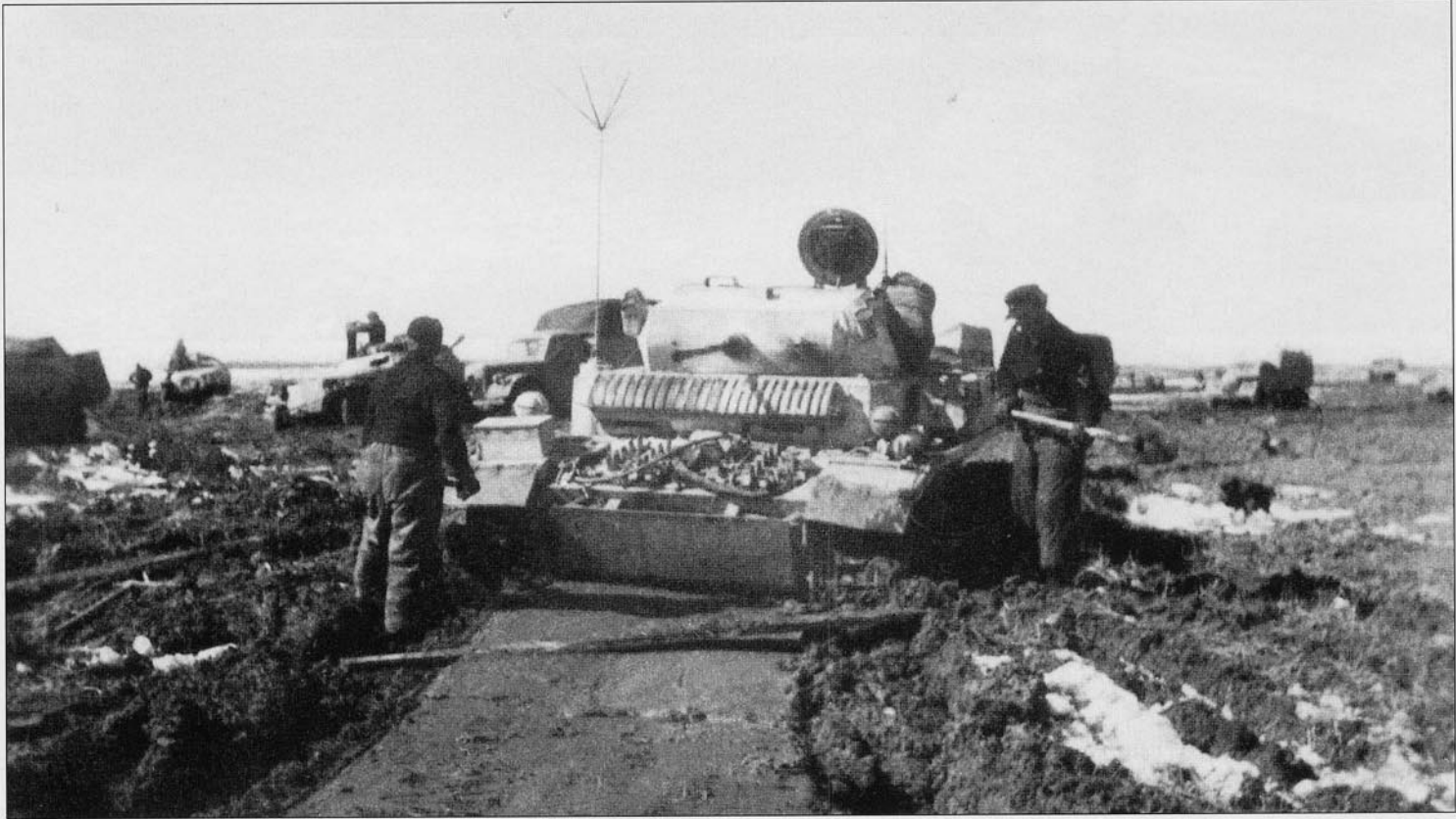
Two shots of a command version of the Pz.Kpfw.II Ausf.L 'Luchs' identified by the star antenna. In the above photo, the vehicle has become bogged down in the mud and the crew are working to free it. Even though it had a relatively high ground clearance, we can see that it has sunk down enough that the tracks can no longer move it. This is one of the original shipment of these vehicles received in the autumn of 1943 and has the spaced front armor plate and the spare idler rack on the front of the hull. The armor plate on the front of the 'Luchs' was only 30mm making it susceptible to small caliber Soviet anti-tank guns. The additional armor plate increased the protection to the equivalent of 50-60mm of armor plate.
