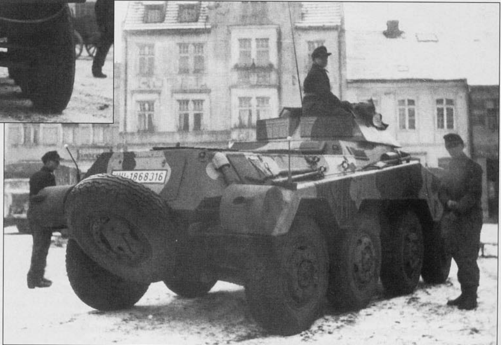
Three views of a new Schwerer Panzerspähwagen (2cm) (Sd.Kfz.234/1), which replaced the Pz.Kpfw.II Ausf.L 'Luchs' as the main combat vehicle of Pz.Aufkl.Abt.4. This photo is taken in January 1945 in the area of Danzig (Gdansk). The vehicle has been painted with a hard edge camouflage scheme of green and brown irregular patches over the dark sand base, applied using a brush. There are no visible markings other than the vehicle license number, WH-1868316, painted on the front and rear plate and a small national cross painted on the side of the turret.
