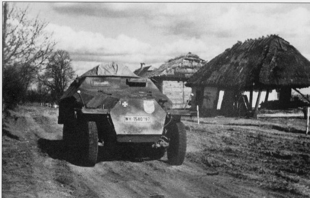
An older model Sd.Kfz.251/1 Ausf.C with a heavy camouflage pattern of green and brown over the dark sand base. It had the Divisional emblem painted on the front but it has been obscured, probably by a censor. It also displays the vehicle license number WH-1540197 and has a small Iron Cross emblem painted on the top left corner of the front plate, possibly indicating a crew member has been awarded this decoration or, perhaps, a Knight's Cross. There is a small number '3' beside it which may indicate the company to which the vehicle belonged.
