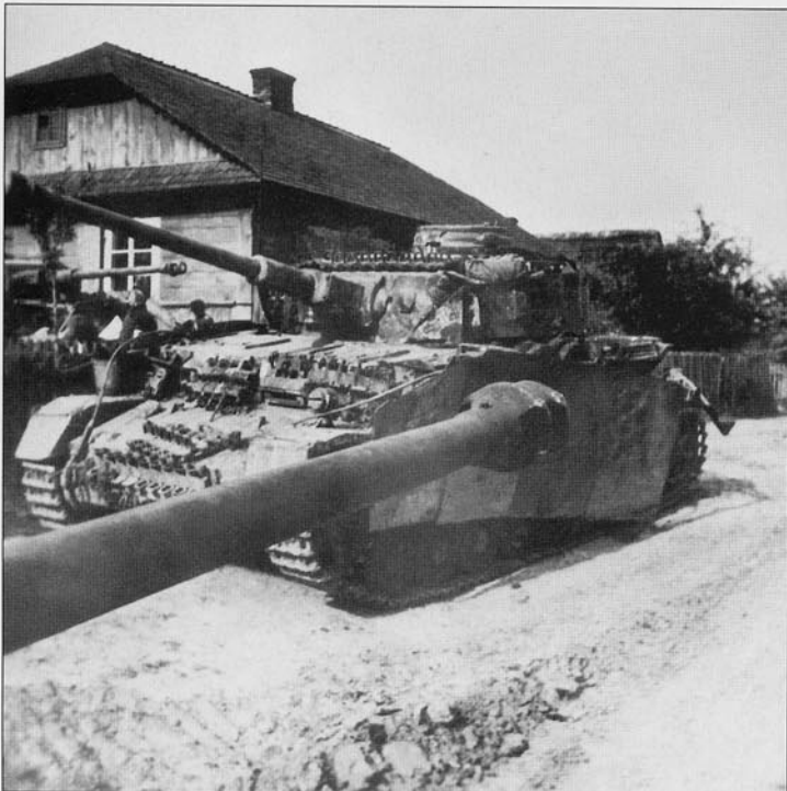
The same late Pz.Kpfw.IV Ausf.G or early Ausf.H seen in the previous photographs giving a good view of the damaged side skirts. The rear skirt is missing and the support angle has been bent back causing the skirts to almost touch the ground. This shot also shows the white standing bear emblem painted on the turret skirt along with the tactical number '532' painted in yellow.
