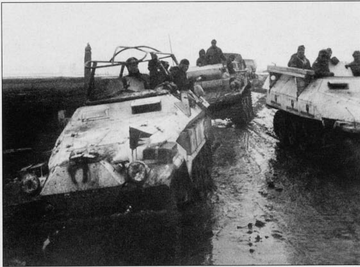
The familiar Sd.Kfz.251/6 Ausf.B command half-track of Gen.Lt. von Saucken on the left and an Sd.Kfz.251/7 Ausf.D Pionierpanzerwagen on the right followed by one of the Division's early Pz.Kpfw.II Ausf.L 'Luchs' and two transport trucks. The assault bridges normally carried by the Pionier half-track are missing and a couple of wooden planks are in their place. It didn't take long for wet, muddy conditions to compromise the winter camouflage of these vehicles.
