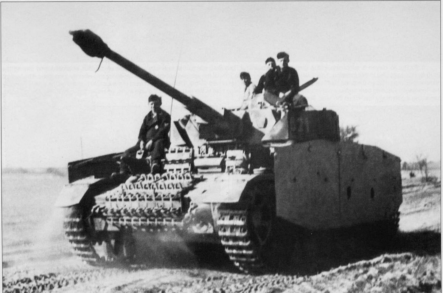
A late model Pz.Kpfw.IV Ausf.G with the later style commander's cupola. The tactical number '621' is painted in a white outline style on the turret skirt. The tank is in relatively good condition for this late stage of the war.
