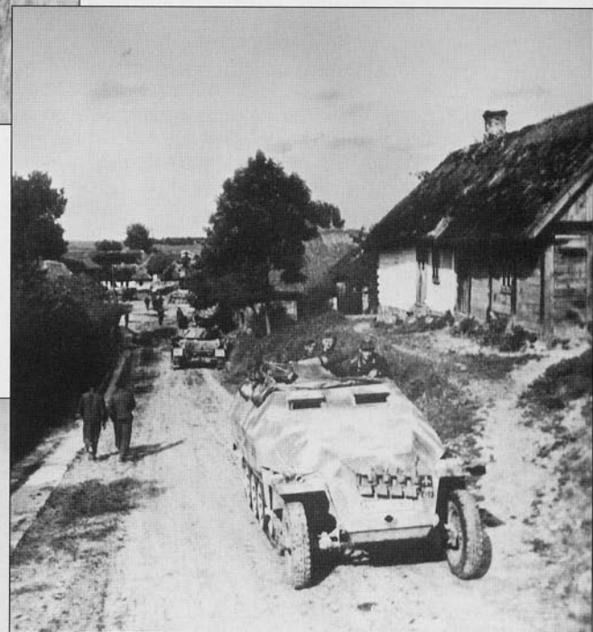
An Sd.Kfz.251/1 Ausf.D makes its way through a small village. The tactical marking to the right of the spare tracks links indicates this vehicle is from 7.Kp. of either Pz.Gren.Rgt.59 or 112 of 20.Panzer-Division. The Division suffered heavy losses and the remainder was incorporated into 4.Panzer-Division in the middle of July, 1944. The camouflage pattern is composed of large areas of green and brown on the dark sand base.
