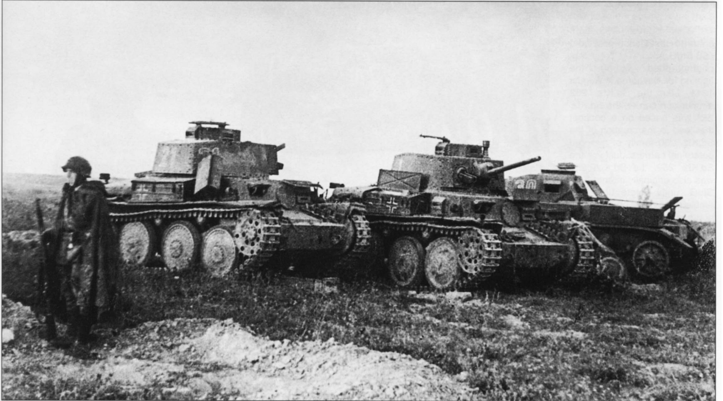
Another group of German tanks captured by the Soviets. These two Pz.Kpfw. 38(t)s and the Pz.Kpfw. II, which belonged to 7.Panzer-Division, were lost during the long, stubborn battle at the Smolensk-Moscow highway near Yartsevo in July 1941. Note the markings on the Pz.Kpfw. 38(t) at the left and the Pz.Kpfw. II at the right — they have numbers of only two digits painted in red with a white outline. The previous number of the second Pz.Kpfw. 38(t) was probably painted over. General Hermann Hoth's Panzergruppe 3 tried to finish off the Soviet troops northeast of Smolensk, but its most advanced division was stopped and counterattacked by strong enemy forces in the Yartsevo area. The fighting for Yartsevo lasted for seven days, and the town was taken and re-taken two or three times a day by the opposing forces.
