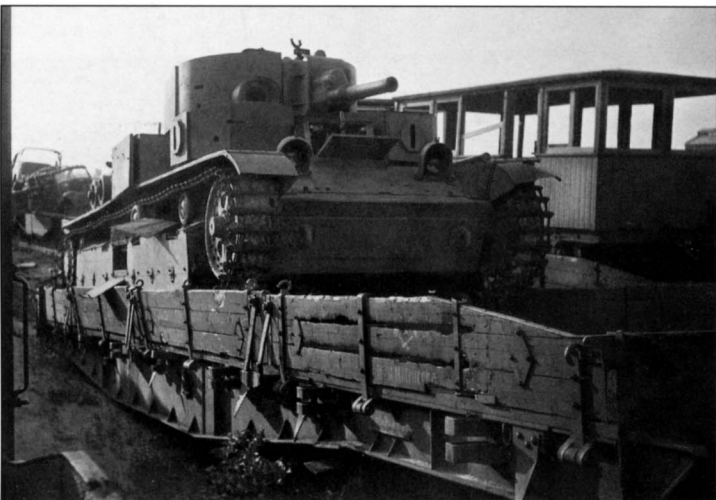
Many of the railway transports that were not destroyed fell into German hands. This photo shows a T-28 medium tank that was left behind to the enemy after its transport platform was derailed. Note what excellent condition the tank is in.
