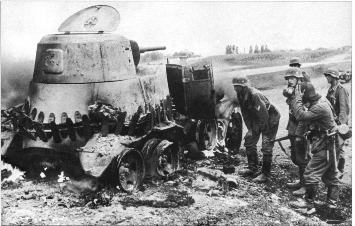
The gesture of the soldier nearest to the camera indicates his amazement at the total destruction inflicted on this BA-10. The armored car was totally demolished by a direct hit to the fuel tank. Supplementary track was strapped around the hull, which could be placed over the rear wheels to convert it into a half-track to help negotiate difficult terrain. Note the turret details: the hatch in its rear and the interior elements of the ventilation mushroom on the top hatch.
