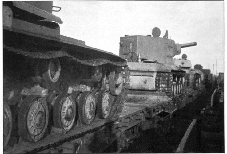
The two giants of the Red Army, the KV-2 heavy tank and the KV-1 tank (in the background), are visible in this photo. The KV-2 came as a surprise to the Germans in the early days of the war. It was invulnerable to any tank or anti-tank gun at that time and could only be stopped by heavy artillery or 8.8cm anti-aircraft guns. However, the KV-2s were prone to mechanical breakdowns.
