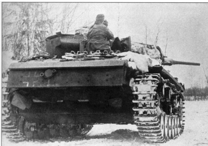
This Pz.Kpfw. III Ausf. H was photographed while patrolling village roads in February 1942, when heavy fighting erupted behind German lines. The crew members are bundled up against the cold weather of the winter of 1941/1942. The frontal part of the turret is covered with whitewash camouflage.
