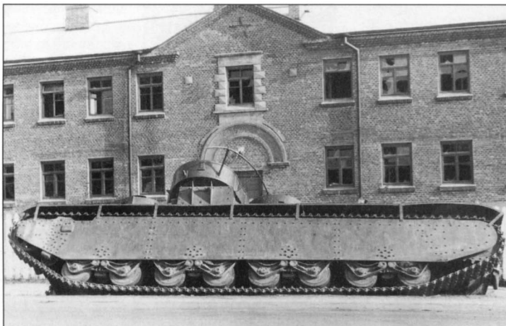
This T-35 self-propelled "fortress" became lodged in a ditch, this time in the center of a small town in front of a public services building. This is the command version from the 1936-1937 series. The massive dimensions of this tank, a length of almost 10 meters (12 yards), is shown well here. For some unknown reason all the turrets are turned in the direction of the ditch.
