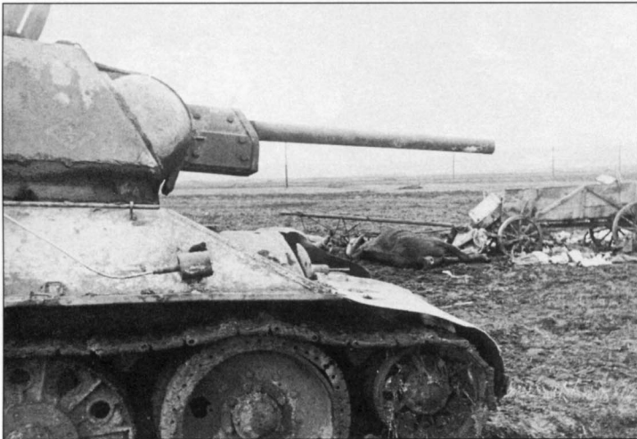
This up-armored T-34 Model 1942 was modified with additional armor by Plant No. 27. The pieces of added turret armor are easily seen in this photo. This type of modification was not popular among higher ranks of technocrats and politicians, who forced mass production of the T-34 as much as possible. They were more interested in more, rather than better, T-34s.
