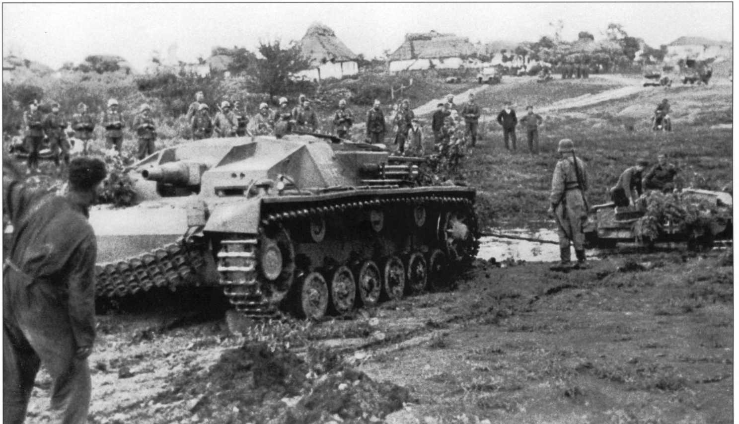
German tank crews sometimes had rotten luck. Here a friendly StuG III Ausf. D hauls another StuG III out from a muddy pool. This work would normally be done by a strong, half-track tractor. Since there were not too many of them available during the early weeks of fighting, they had to be replaced by combat vehicles.
