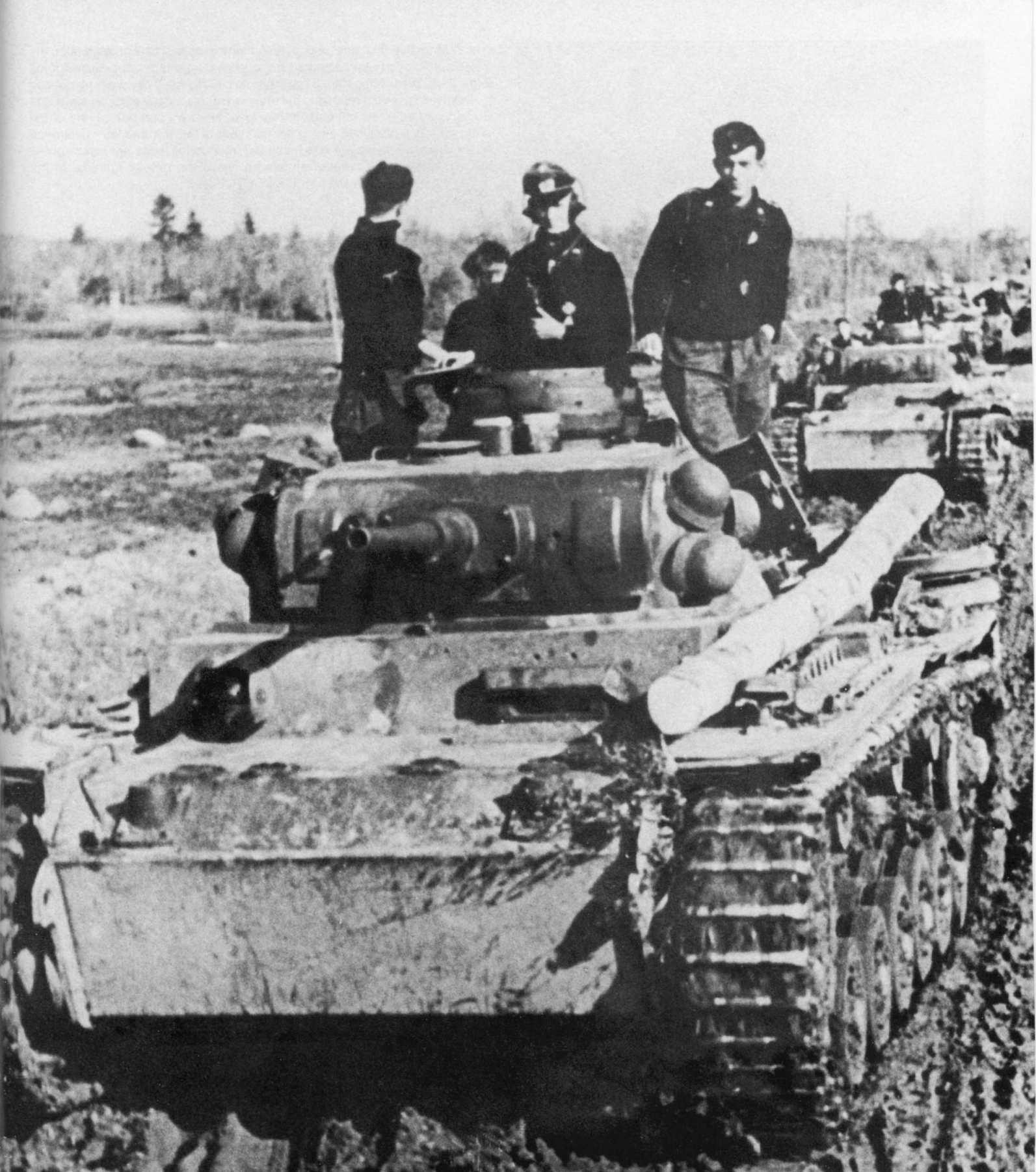
In early autumn 1942 a column of Pz.Kpfw. III Ausf. Js equipped with the short-barreled 5cm gun cautiously travels along a muddy road in the southern area of Lake Ilmen, territory controlled by Herresgruppe Nord. At this time the deadliest struggles took place in the Demyansk corridor area where 8.Panzer-Division was employed by 16.Armee and supported by the independent Pz.Rgt.203. The Pz.Kpfw. IIIs seen here may belong to the independent regiment because 8.Panzer-Division was equipped with Pz.Kpfw. 38(t)s and a few Pz.Kpfw. IVs as heavy support for the light tanks. The tanks are completely covered with mud except the gun mantlet and the gun barrel, which show the original dark gray background. The entire Panzerwaffe lost a total of 184 Pz.Kpfw. IIIs armed with the 5cm gun in September, while total production of tanks was 217 tanks.
