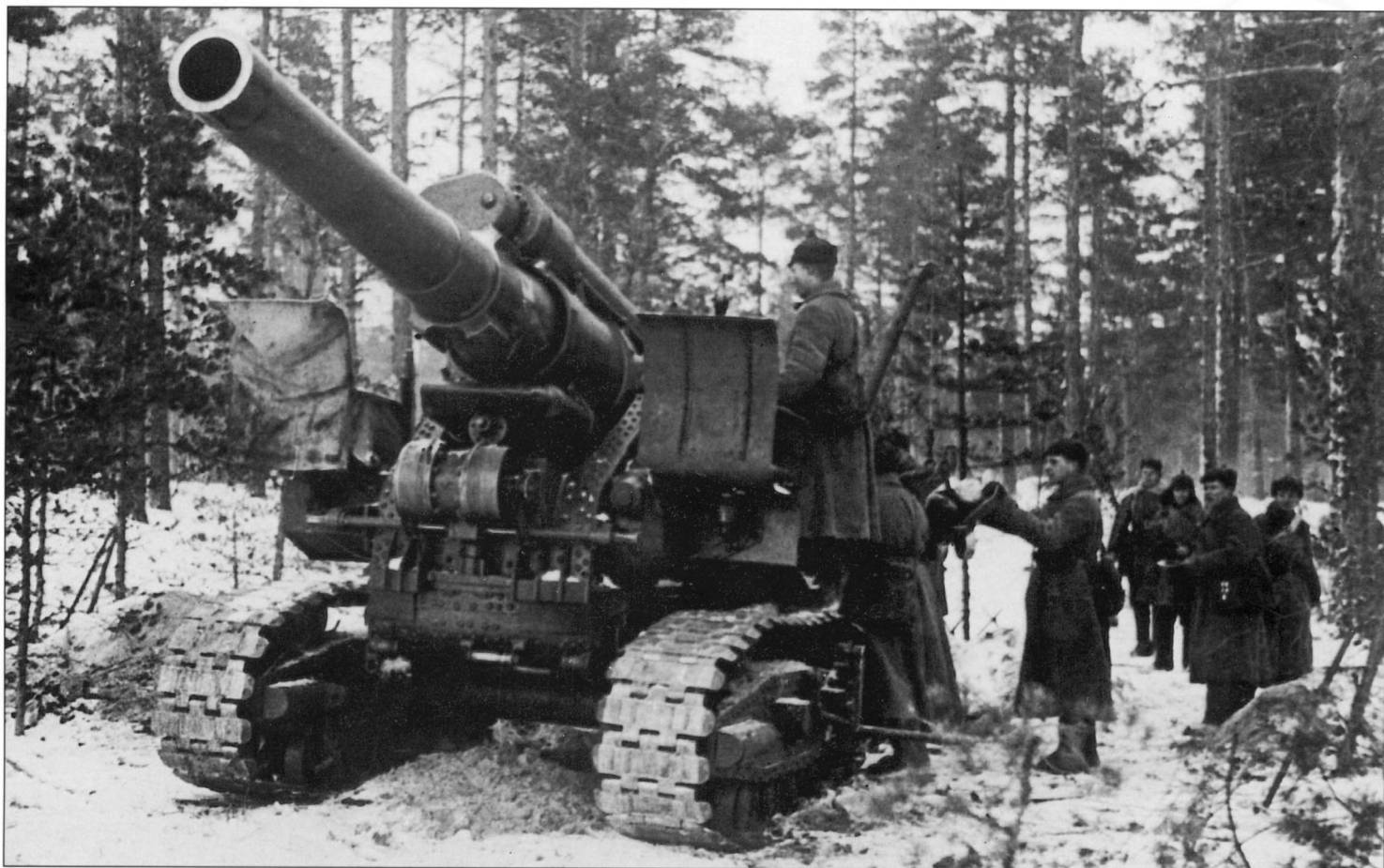
The Soviet equivalent of the French Kanone 485(f) gun was this 203mm B-4 howitzer, which was first produced in 1931. The most powerful gun used by the Red Army, it was attached to a special fully tracked vehicle, which carried a 15-man crew, tools and ammunition, and this pair was towed by powerful tractor. Due to shortages in production, the special tractor was often replaced by another — the S-65, for example. The lighter version of the gun was equipped with wheels, while the heavier version remained static.
