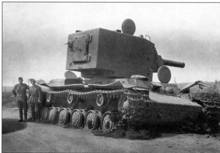
Another KV-2 tank. This one was abandoned after being damaged in combat. The heavy tanks, especially the KV-2s, were an unpleasant surprise for the Germans. For many weeks staff officers did not believe the reports received from front-line units that they had encountered tanks armed with 152mm guns, armored with 75-100mm plates and weighing about 50 tons. The heaviest German tank at the time was armed with 7.5cm gun and weighed about 20 tons.
