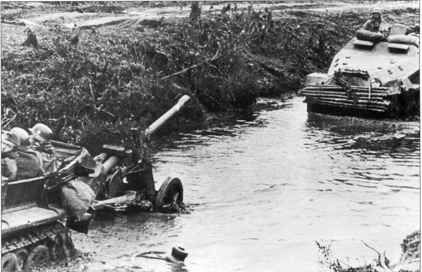
Vehicles of 1.Panzer-Division move through a stream in autumn of 1941. At left is a Sd.Kfz. 10 towing a 5cm PAK 38 anti-tank gun, while at right is a Sd.Kfz. 251/1 Ausf. B half-track. During the struggles for Moscow, this division belonged to XLI Ar.Kp. of Pz.Gr.3 and fought on the northern flank. Despite the lack of Pz.Gr.40, whose supplies had been cut off by Hitler's order, the division used the PAK 38 very successfully to repulse Soviet armored counterattacks until the beginning of December.
