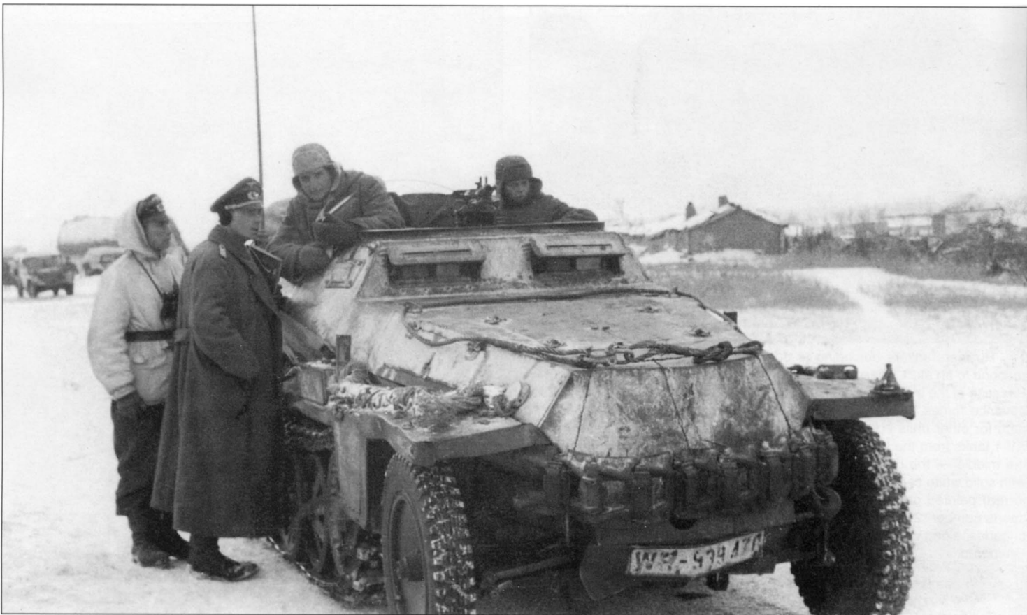
This Sd.Kfz. 250 from 22.Panzer-Division was photographed somewhere in Russia in the winter of 1942. The emblem of the division is painted on the right side of the frontal plate, and the license number is "WH 939476". Note how the towline is affixed to the engine deck.
