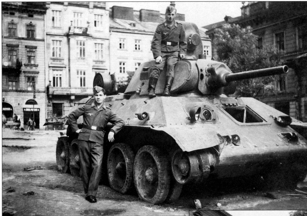
A souvenir photo from a "trip" to Lvov in July 1941 taken by Luftwaffe personnel, showing two of them and a knocked-out T-34 Model 1940 from 4th Mechanized Corps. Clearly visible in this photo is the ventilation on the turret hatch and an extra transmission lashed to the engine deck. Also abandoned on another street was at least one T-34 from the same unit with a similar transmission on the rear deck.
