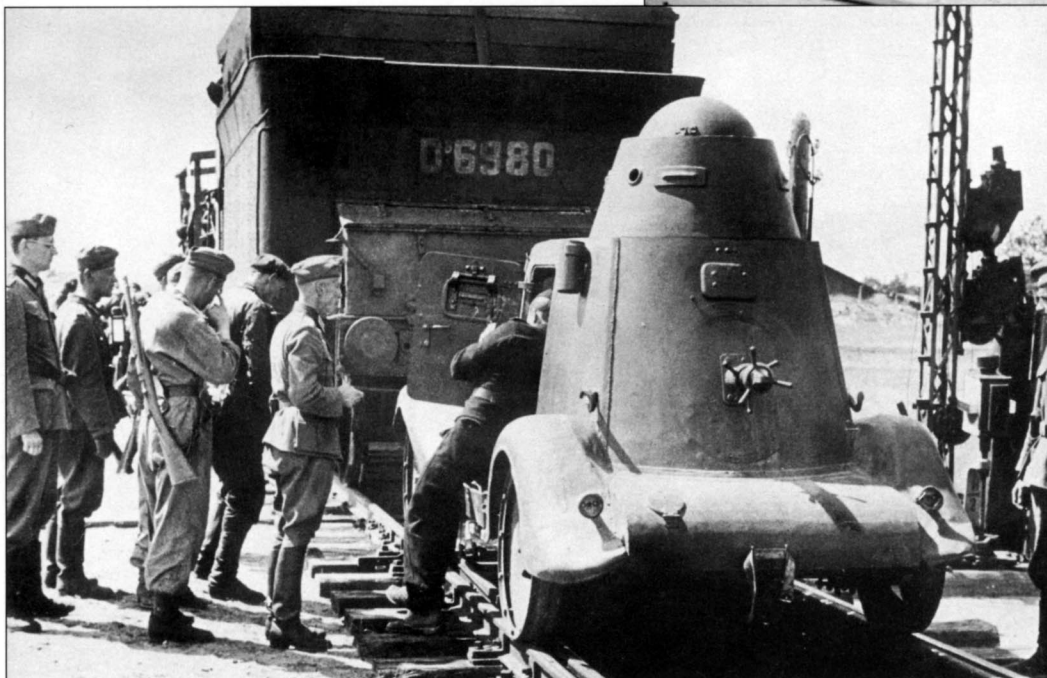
A few dozen BA-20 armored cars were modified to the BA-20 ZhD railway version and adopted for use by railway protection forces. Here we see one of the captured vehicles being inspected by the Germans, who named this type of vehicle the Pz.Sp.Wg. BA-20 2(r).
