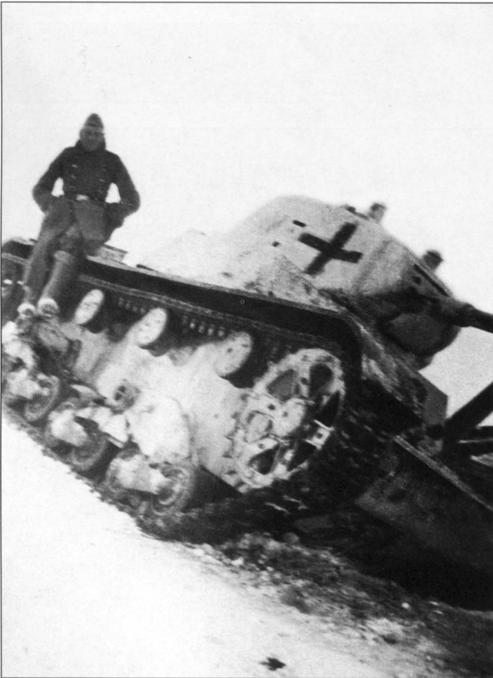
Another victim of the winter fighting — a Soviet T-26 Model 1939 captured by the Germans and then abandoned during a march due to mechanical breakdown or bad weather. The tank wears a solid coat of white camouflage and the black national cross on the front part of the turret. A similar cross was probably applied to the rear, too. Note that the tank has no additional markings. This may indicate that it was a supplementary tank in a unit.
