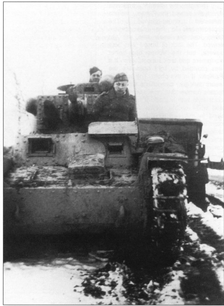
Another shot of a Pz.Kpfw. 38(t) from the same unit traveling down a Russian country road. This photo gives a good indication of the size of the tank, which was too small by German standards, making it quite uncomfortable for the crew. Note that all surfaces on the front of the tank are covered with a solid coat of mud.
