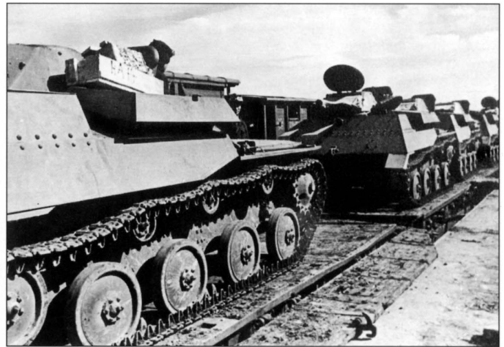
From the beginning of the war the Soviets sent to the front lines hundreds of trains carrying vehicles for the fighting troops. This scene shows the transport of T-40 amphibious tanks armed with 12.7mm machine guns. These vehicles were used by the reconnaissance troops of some divisions in place of the T-37/38 tanks.
