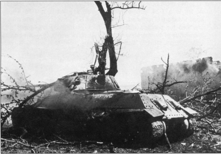
This up-armored T-34 Model 1942 was modified with additional armor by Plant No. 27. The pieces of added turret armor are easily seen in this photo. This type of modification was not popular among higher ranks of technocrats and politicians, who forced mass production of the T-34 as much as possible. They were more interested in more, rather than better, T-34s.
