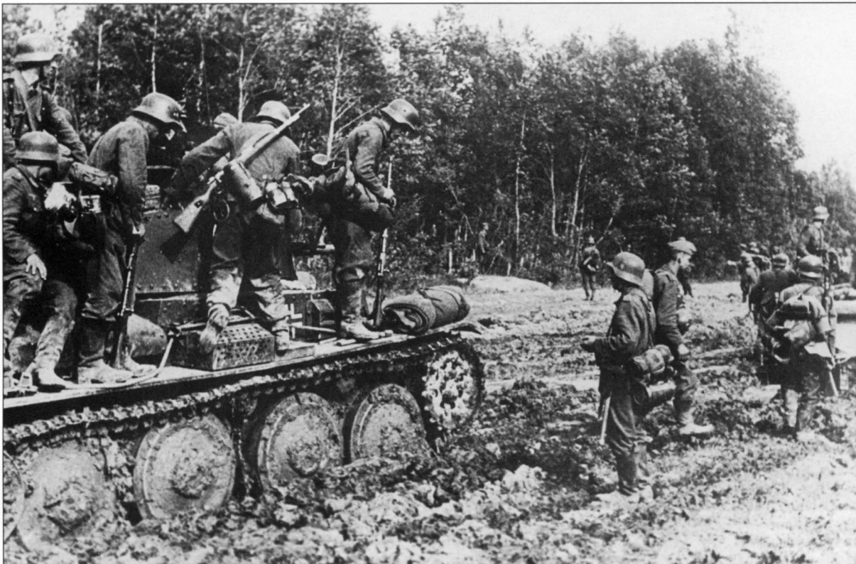
More battlefield litter that was left in the path of the advancing Germans. The tank was hit in the first road wheel (notice the hole) and the construction of the chassis was altered in this place. The road wheel is higher now, at a height even with the front idler. Note the small unit markings on the mud-covered turret. More important is the fact that the horse drawn wagon in the background is loaded with boxes of ammunition. This reflects the condition of the Red Army during most of the war. Soviet industry turned out tens of thousands of tanks and guns, but only a few light trucks, which had to be replaced by slow, small transport vehicles that were much weaker than tanks and more vulnerable to enemy fire.
