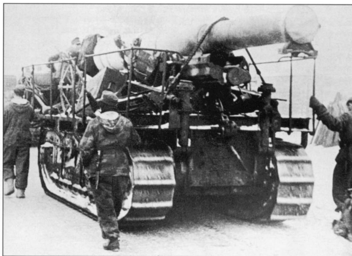
In 1942 the 194mm Kanone 485(f), the old French self-propelled gun produced in the mid-1930s, was sent into action in the northern sector of the Eastern Front for use in the siege of Leningrad. The vehicle is probably painted with French camouflage.
