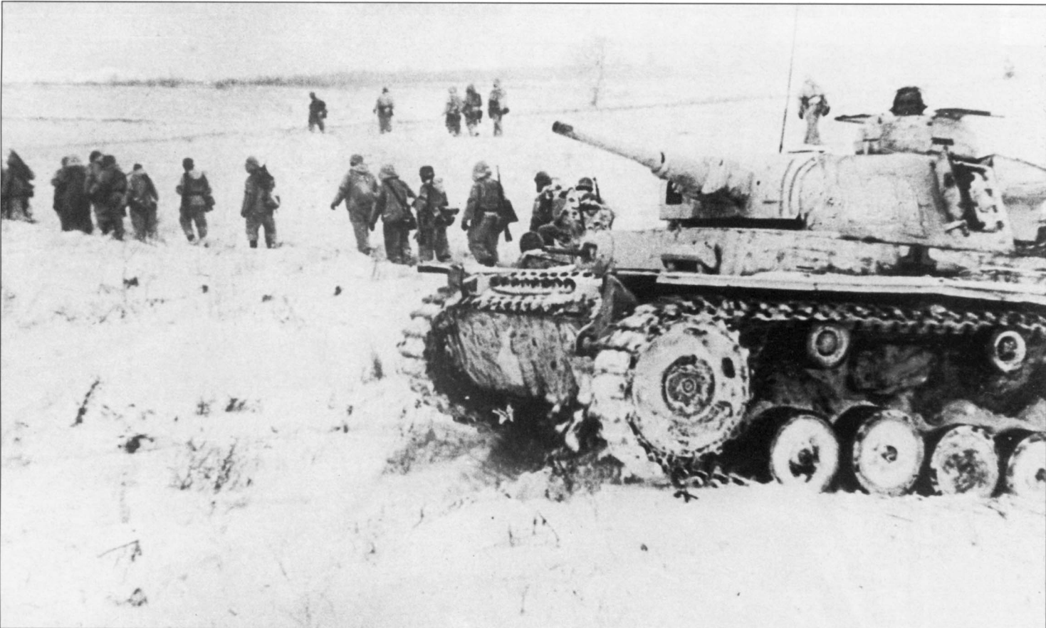
Germans troops fan out across the wide steppes of southern Russia during the winter fighting of 1942/43. In the foreground is a Pz.Kpfw. III Ausf. J with a heavy coat of white winter camouflage. Note the national cross painted on the side of the superstructure — its white outline is much darker than the white camouflage. During the great battle of this winter season from November 1942 to February 1943, which took place between the Caucasus, Stalingrad and Kharkov, the Soviets lost almost 4,500 tanks, while the total losses suffered by the Panzerwaffe on all fronts were: around 2,600 tanks, about 320 StuGs, and about 230 self-propelled guns. Most of them — almost 1,700 of these vehicles — were lost in the Stalingrad conflict.
