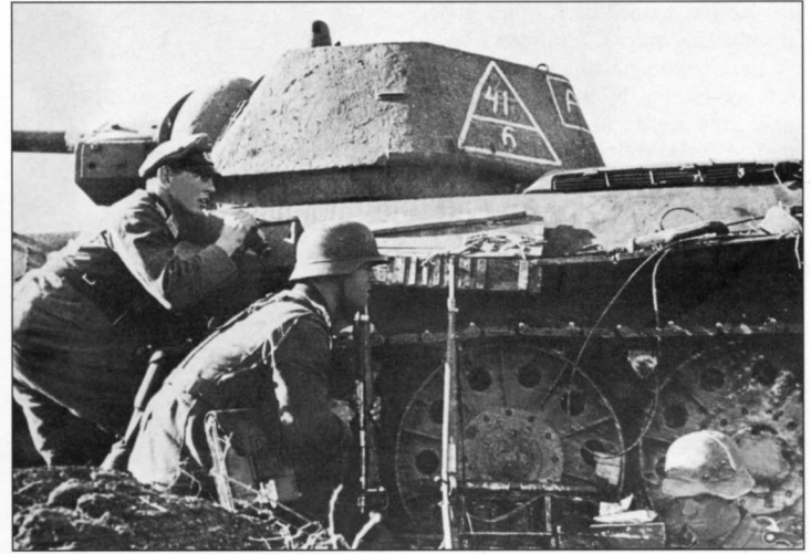
A T-34 Model 1943 with its hexagonal turret covered with unit markings typical of the 1942-1943 period is used as cover at an advanced position occupied by German infantry. Note that the triangle with the "41/6" code was painted over previous markings that are still just barely visible. The first T-34 Model 1943 with the new version of turret was introduced at the end of the summer of 1942 and immediately sent to the front in large numbers.
