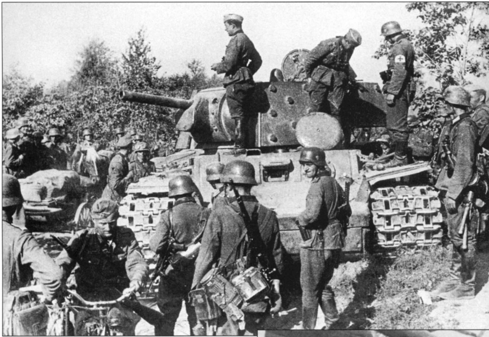
Modern Soviet KV-1 tanks that were abandoned along the roads of the Baltic states made a great impression on the German soldiers. They had never before seen such giants, so they all wanted to closely examine these vehicles, as is evidenced by this photo. Here at least a couple of dozen soldiers are admiring a KV-1E Model 1941 heavy tank. Note the appliqué armor bolted to the turret and the short F-32 gun.
