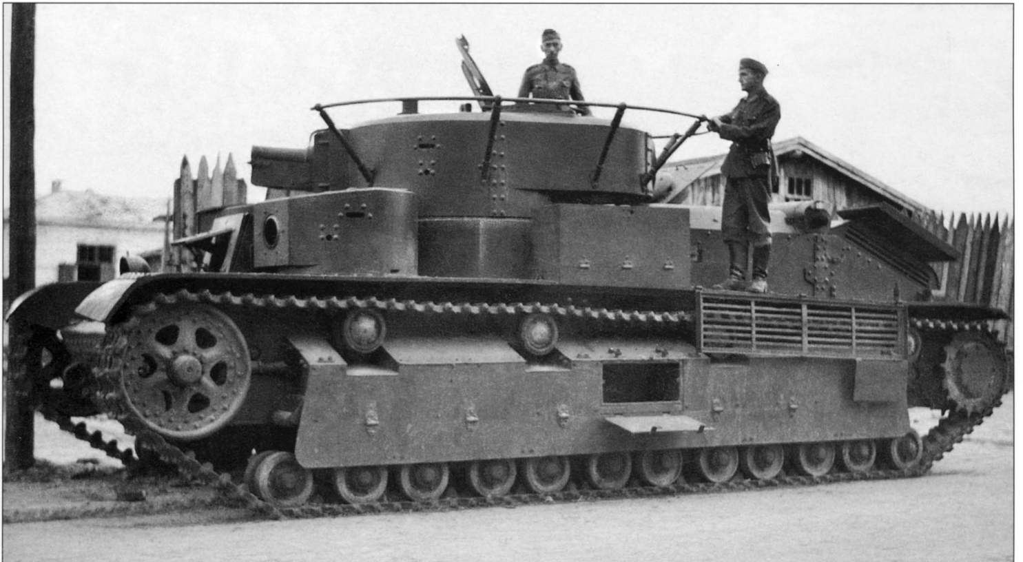
The Soviet medium tank of the 1930s, the T-28, was big, slow and had thin armor. There were 490 of these tanks produced between 1932 and 1939, and about 400 of them were in service at the beginning of Operation "Barbarossa", mainly in the 3rd, 5th, 8th, 10th, and 15th Tank Divisions. This is a command version of the T-28, apparently abandoned due to a mechanical breakdown or fuel shortage. Note the short-barreled KT-28 76.2mm gun.
