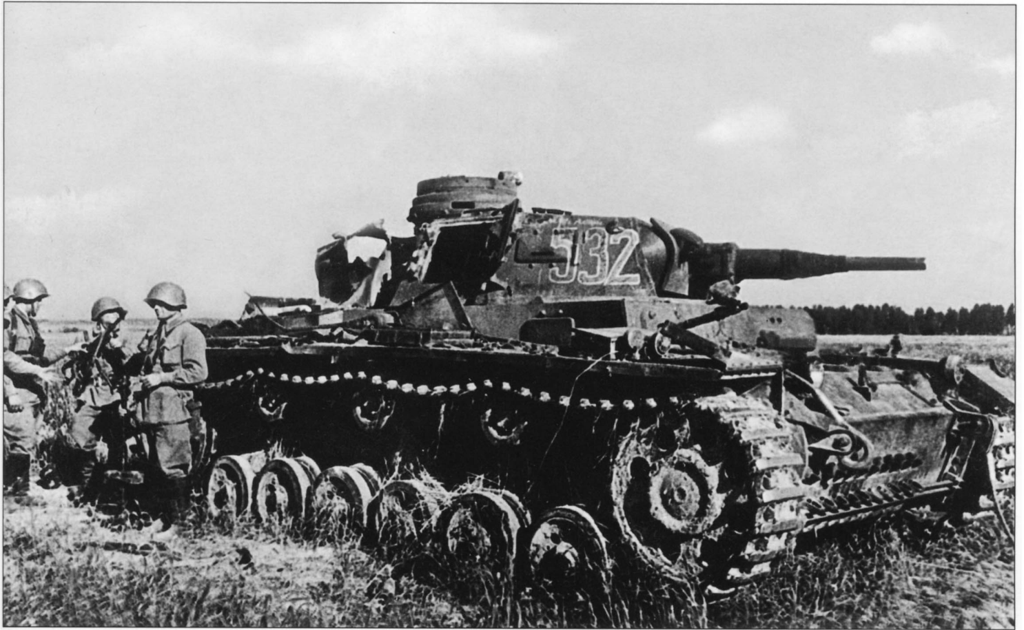
The same Pz.Kpfw. III tank photographed from the other side. This vehicle has a smaller tactical number "532" painted in red with a white outline. Note the damage to the stowage box — it shows where a round tore through then ripped off part of the door of the turret's hatch.
