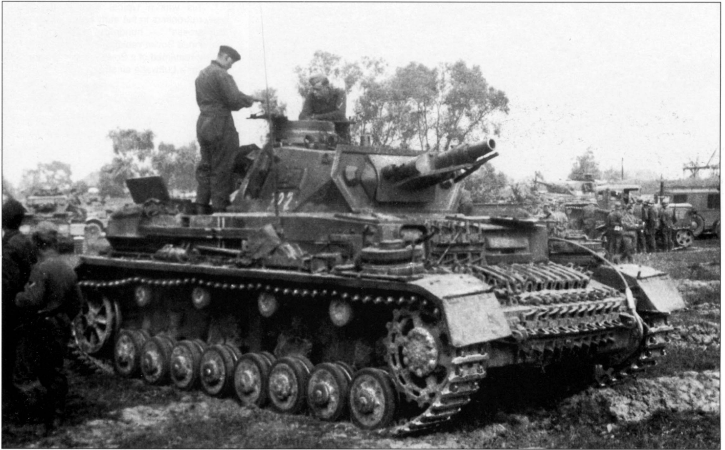
A Pz.Kpfw. IV Ausf. D in the so-called "U-bootpanzer" (Tauchpanzer) configuration, which permitted the tank to submerge in water up to 15 meters (16.5 yards) deep. These Tauchpanzer IVs were originally developed for the preparation of Operation "Sea Lion", the invasion of England, but were eventually used to cross the River Bug in June 1941 during Operation "Barbarossa". Note the frame around the turret front; this is the mounting frame for the waterproof fabric cover. The Tauchpanzers were mainly used by 18.Panzer-Division of Guderian's Panzergruppe 2.
