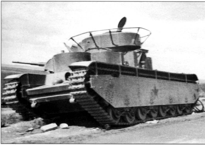
A T-35 from the 1934-1937 production series, which is equipped with a frame antenna, lies abandoned in a ditch. Note the Soviet red star on the side of the armor.
