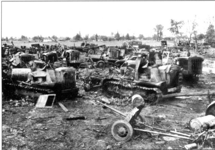
The field concentration of vehicles belonging to an anti-tank unit was photographed following an air strike. All visible tractors are the ChTZ-65 "Stalinet" artillery tractor, which was designed on the base of the agricultural tractors, like American "International TD", for example. Factories could produce them for both military and civil duty without any troubles, but this civilian machine was not popular with the military crews. The guns are the two main types at that time: the 45mm model 1937 (designed on the base of the German 3.7cm PAK 36/37 gun) and the 107mm model 1910/30 and model 1940.
