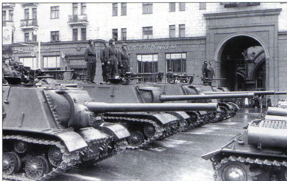
The imposing sight of companies of heavy assault guns greeted Russian spectators during the June 1945 Victory Day parade in Moscow. Here is a line up of ISU-122 assault guns on the streets leading into Red Square. In the foreground is the initial ISU-122, while behind it is an ISU-122S.
