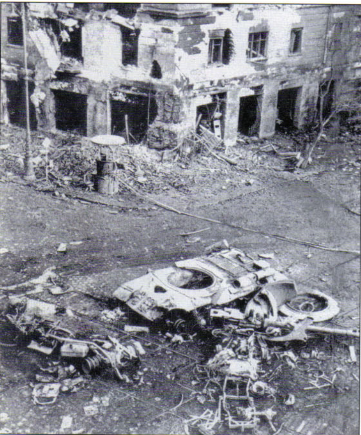
The IS-3 saw major combat action only a few times in Soviet service. This is an IS-3 knocked out during the bitter fighting against Hungarian insurgents in Budapest and probably belonged to the heavy tank/assault gun regiment of the 33rd Guards Mechanized Division. It has suffered from an internal ammunition fire which has completely lifted off its turret. (US Army Ordnance Museum, APG)
