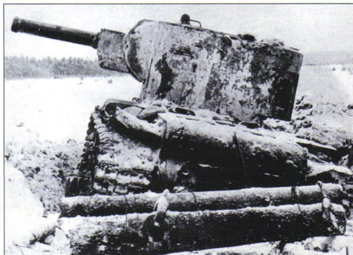
Very few KV-2 tanks survived the summer 1941 fighting. This is a rare example of a KV-2 Model 1940 that was still operational during the fighting in the winter of 1941-42, with white winter camouflage. It has become bogged down and the crew has attempted to extract by pulling unditching beams underneath it, without success.
