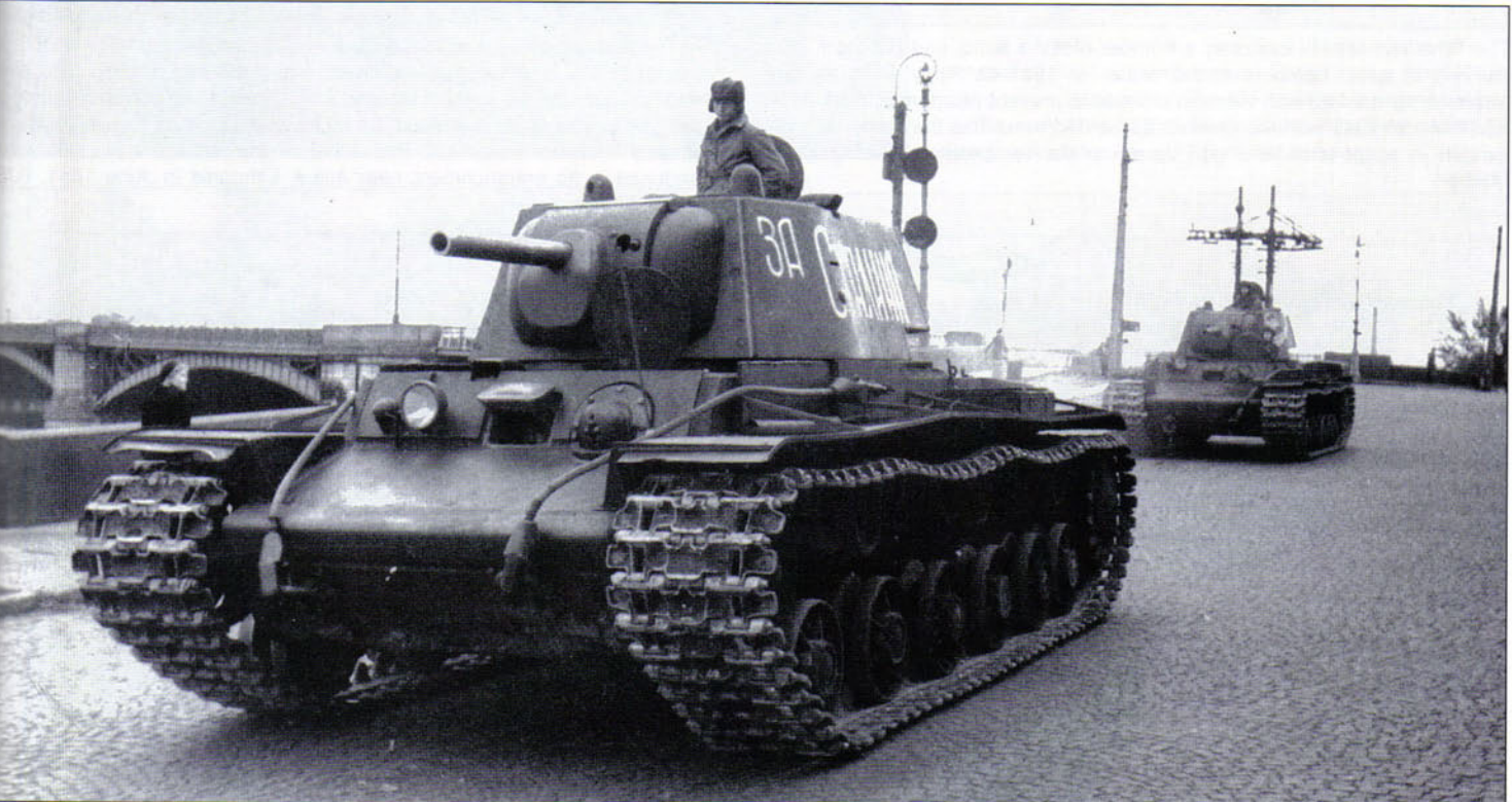
A clearer view of the KV-1 Model 1941 seen in the upper photo. This tank carries the slogan "Za Stalina!" (For Stalin!) on its turret side. This also has the new uparmored turret, as well as appliqué armor on the bow, superstructure front and on the hull sides.
