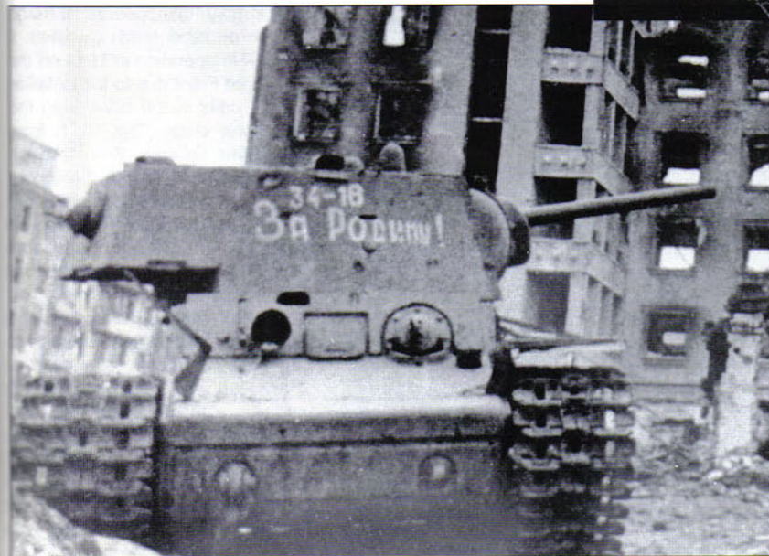
A clear view of a KV-1 Model 1941 with the uparmored welded turret. As will be noted, the turret side plate continues straight back instead of curving under the turret overhang. This vehicle is fitted with the new ZIS-5 76.2mm gun and has standard hull and turret appliqué armor. The rectangular armor patch under the side pistol port was probably to repair battle damage.
