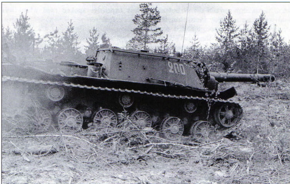
The most important sub-variant of the KV tank series was the SU-152 assault gun. These vehicles, manned by tank troops, were used to provide direct fire support of infantry and armored formations. This SU-152, probably of the 1539th Heavy SP Artillery Regiment of the 3rd Shock Army, 2nd Baltic Front was commanded by Lt. S. F. Berezin. (Soloviev)
