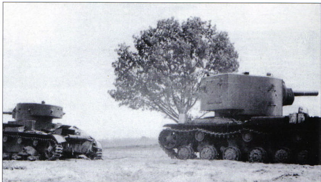
The companion vehicle to the KV-1 was the KV-2, originally called the "large turret KV". This version was armed with a 152mm howitzer and was intended to provide fire support when attacking reinforced concrete bunkers of the type encountered in Finland. So far as is known, only four of this early production version were built. This tank of the 5th Tank Division was abandoned in its entrenchment near Alitus, Lithuania in June 1941. (US National Archives)
