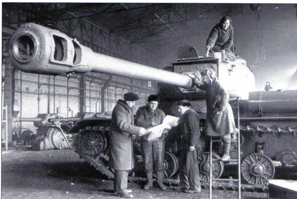
By August 1944, production at Chelyabinsk was beginning to shift over to the improved IS-2m heavy tank. This used a new front hull casting and a wider gun mantlet. Here a tank undergoes final inspection and painting in early 1945. In the background are gun assemblies for the ISU-152 heavy assault gun.
