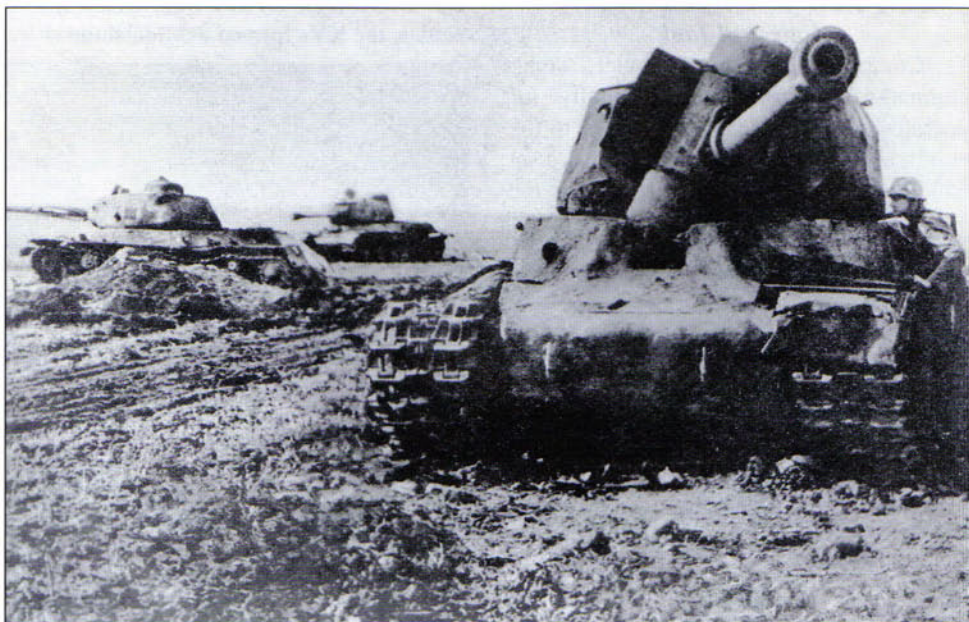
A German soldier inspects a knocked out IS-2. Although the IS-2 was largely impervious to the Panther and Tiger frontally except at close ranges, it was still vulnerable on its thinner sides. The tank in the foreground probably suffered an internal ammunition fire, as the front turret mantlet casting has been separated at the joint from the rest of the casting.
