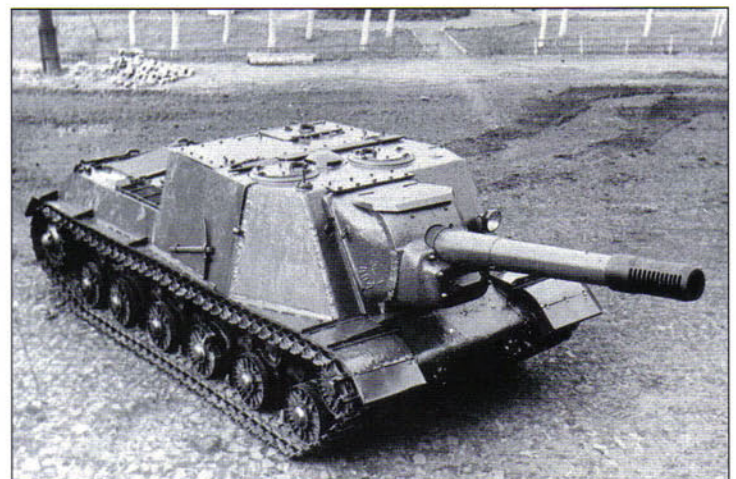
In the autumn of 1943, the Chelyabinsk designers began to adapt the SU-152 assault gun to the IS tank hull. The result was the ISU-152 assault gun. This is the original prototype of the vehicle and it is quite clear that there were few changes between the prototype and series production vehicles.
