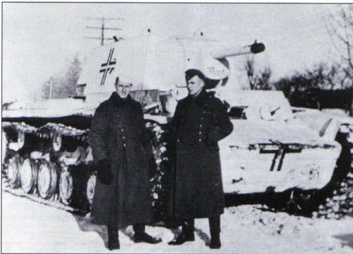
The Wehrmacht captured a number of KV-1 tanks and put them into service in small numbers in the winter of 1941-42. They were always prominently marked with German crosses to prevent misidentification. This KV-1 Model 1941 with the uparmored welded turret has the name "Marta" written in script under the gun barrel on the recuperator housing. (Lee Archer)
