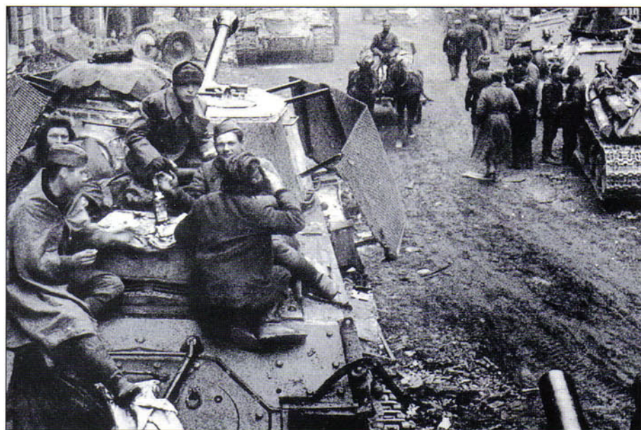
Although not of best quality, this is a rare view of an IS-2m fitted with stand-off screen armor on its turret during the Berlin operation. While some of the anti-Panzerfaust screens were made from looted bed-springs, many were made by local Red Army mobile workshops as appears to be the case here.
