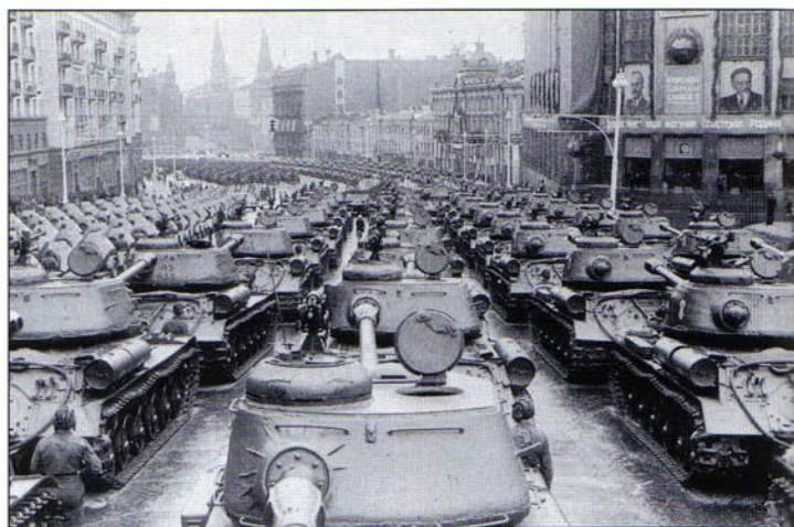
The streets leading into Red Square are crammed with armored vehicles as the Victory Day parade begins in Moscow in June 1945. The casting on the rear of the turret of the IS-2m in the foreground shows the effect of wear on the sand casting molds with traces of the steel marker rods showing. These are late production IS-2m tanks with the 12.7mm DShK heavy machine gun mounted on the commander's cupola. To the left of the photo are a large number of BA-64B armored cars.
