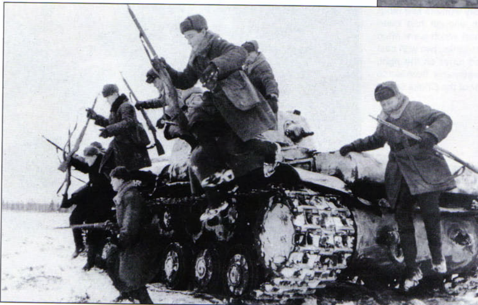
A tank assault squad leaps from a KV-1 Model 1941 during exercises in the winter of 1942. The Red Army lacked armored infantry vehicles, and so used the expedient of having its infantry ride into combat on the backs of its tanks. This is why Soviet tanks tended to have far more hand-holds welded to their tanks than in other armies.
