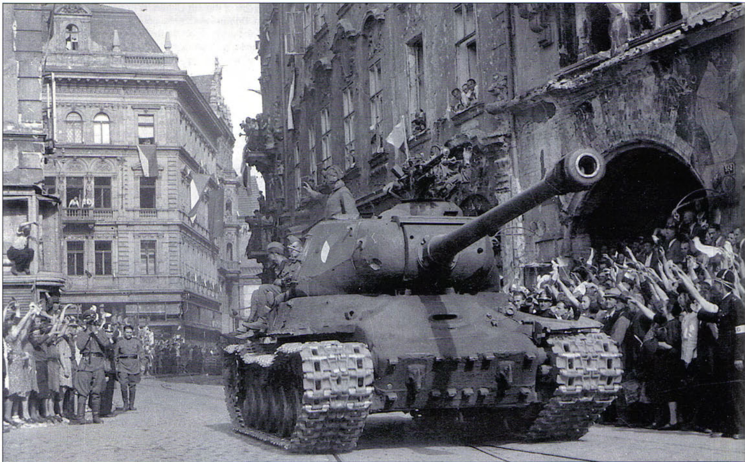
A view of a IS-2m of the Czechoslovak 1st Tank Brigade in the Old Town section of Prague in May 1945. This is a late production IS-2m fitted with the external 12.7mm DShK heavy machine gun on the commander's cupola, a feature only seen towards the end of the war.
