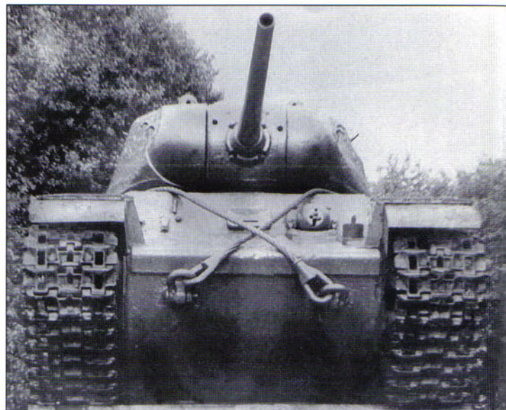
Some KV-85 heavy tanks retained the hull machine gun position as seen here. The KV-85 was used to equip a number of Guards heavy tank regiments in October-November 1943 including the 7th, 11th, 15th and 29th Guards Heavy Tank Regiments. Each regiment normally had a strength of 21 KV-85 tanks.
