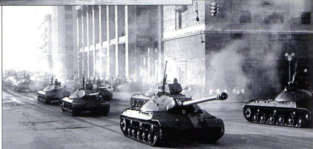
The IS-3 became a staple of Moscow parades after 1946. This is during one of their 1946 parades through Red Square, on Tanker's Day in September 1946 with the Kremlin evident in the background. These are 1946 production tanks, evident from the side stowage bin covers on the hull side.
