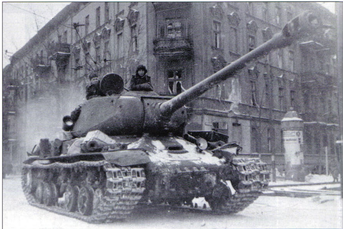
Another IS-2m of the 34th Guards Heavy Tank Regiment in Poznan on 23 February 1945. This tank has already seen some action as its fourth roadwheel station is missing a wheel, from mine damage or a worn-out wheel bearing.
