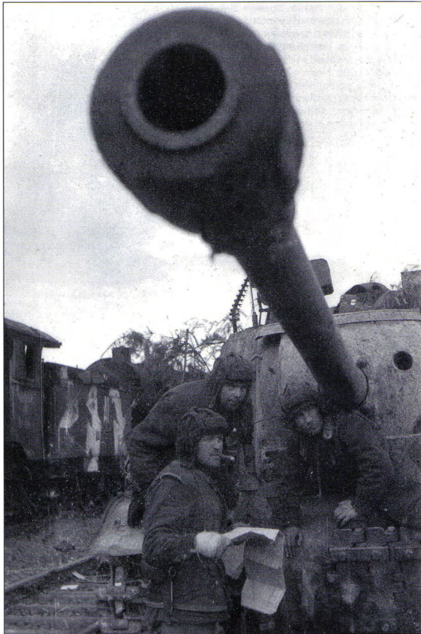
The crew of an ISU-122S commanded by Jr. Lt. Petrov (with the cigar) prepare their mission during fighting by the 3rd Byelorussian Front against the German Third Panzer Army on the Zemland (Samland) peninsula in East Prussia in January 1945. The ISU-122S, also called the ISU-122-2, was an improvement on the basic ISU-122 with the improved D-25S gun. There were no fewer than eight ISU regiments taking part in this campaign with the 3rd Byelorussian Front including the 373rd, 395th with the 5th Army, the 343rd and 345th with the 28th Army, the 337th with the 31st Army and 354th, 348th and 350th Guards Heavy SP Artillery Regiments under frontal command. Indeed, the high value attached to these vehicles meant that they were actually produced in larger numbers than the basic IS-2 heavy tank.
