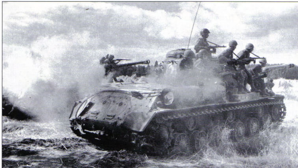
An IS-2 carries a tank assault team forward during the fighting in the summer of 1944. This is a spring 1944 production vehicle, lacking the rear travel lock, but having the new pattern hand-holds.
