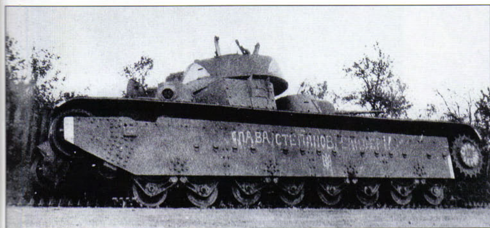
A total of 48 T-35 heavy tanks were operational with the Red Army at the beginning of the war on 22 June 1941 with the 67th and 68th Tank Regiments of the 34th Tank Division, 8th Mechanized Corps in Ukraine. Of these, only 5 were lost in combat, the remainder were abandoned due to mechanical breakdowns. This is the standard T-35 Model 1935 identifiable by its vertical turret sides. (James Crow)
