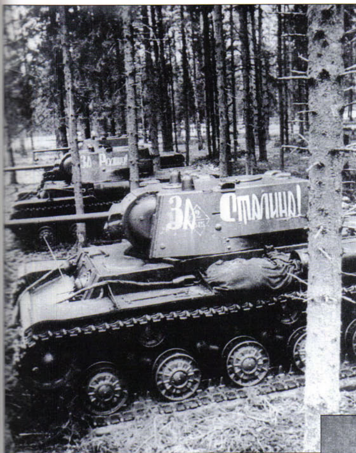
A platoon of tanks from the 116th Tank Brigade in May 1942 on the Western Front. This unit is particularly well known as it was photographed heavily during its training period in the spring of 1942. The vehicle nearest the camera is a KV-1 Model 1941 and carries the slogan "Za Stalina!" (For Stalin). The 2 in the tactical marking probably indicates the 324th Tank Battalion. The KV-1 Model 1941 with cast turret carries the slogan "Za Rodinu!" (For the Homeland). The nearer KV is a mixture of early and late features, mounting the newer ZIS-5 76.2mm gun and hull appliqué armor, but still using the older pattern welded turret, and early pattern roadwheels.
