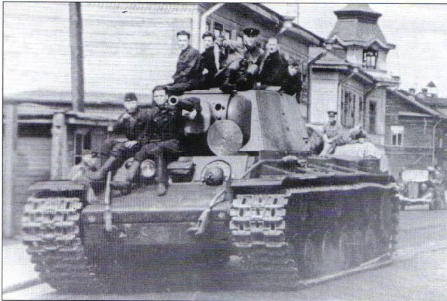
A KV-1 Model 1941 with uparmored welded turret going into combat in the suburbs of Leningrad in the late summer or early fall of 1941. The F-32 continued to be mounted in the KV-1 tank for some time after more effective ZIS-5 76.2mm gun was already being fitted in the T-34 medium tank.
