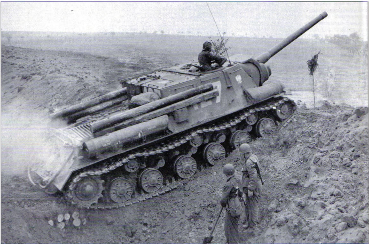
The Polish Army also kept the ISU-122 in service well into the 1960s. Here a vehicle crosses a fascine bridge laid by engineer troops to breach an anti-tank ditch during field exercises. (Janusz Magnuski)
