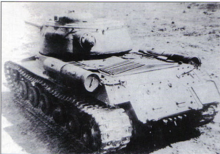
A rear view of the IS-85 prototype at Chelyabinsk in November 1944. Many of the features of this tank stayed the same with the early production IS-2 such as the lack of a rear travel lock.
