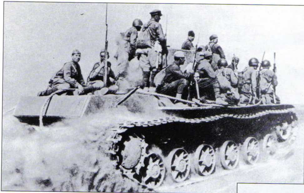
A KV-1 Model 1941 moves into action in the summer of 1942 with a tank assault (tankoviy desant) team on board. This gives a very clear view of the altered rear hull of the KV-1 common on some 1942 production vehicles where the rounded panel gave way to a simpler squared off shape to permit the use of thicker armor plate.
