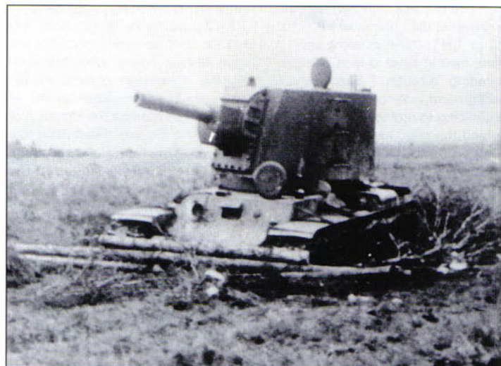
The companion vehicle to the KV-1 was the KV-2, originally called the "large turret KV". This version was armed with a 152mm howitzer and was intended to provide fire support when attacking reinforced concrete bunkers of the type encountered in Finland. So far as is known, only four of this early production version were built. This tank of the 5th Tank Division was abandoned in its entrenchment near Alitus, Lithuania in June 1941. (US National Archives)
