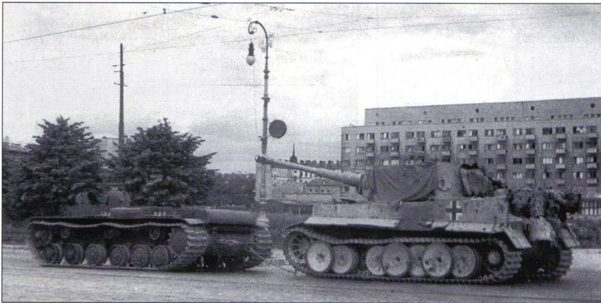
After being retired as battle tanks, some KVs were put to use as recovery vehicles, called KV-T or KV-1T (Tyagach: tractor). Here, a KV tows a recovered German Tiger I heavy tank across Revolution Square in the Petrogradskiy section of Leningrad in 1944.
