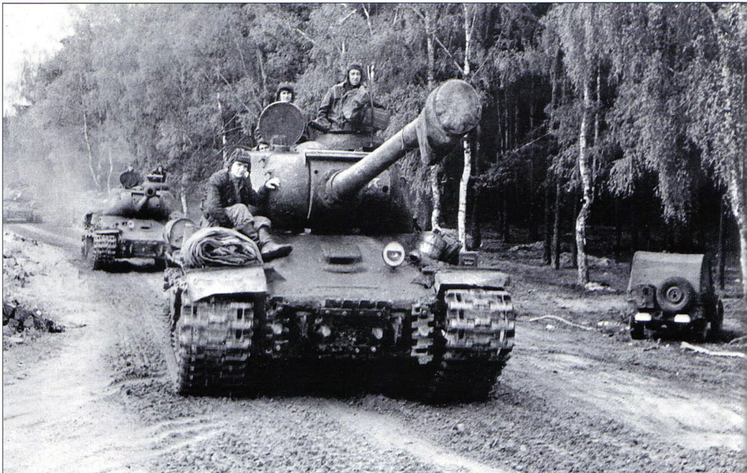
An IS-2m company moves up outside of Berlin in May 1945, with a Lend Lease jeep evident to the right. There is a small white star as a tactical marking on the mantlet, and the front headlight has been partially painted out for night driving.
