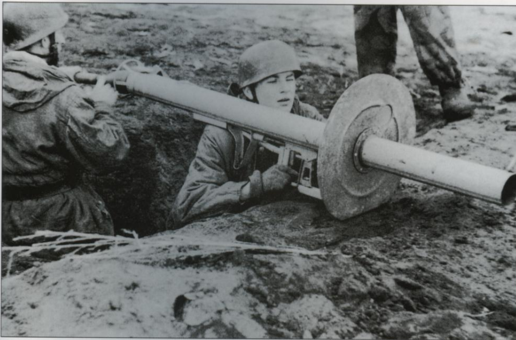
A photograph showing Fallschirmjäger troops training in the use of the 8.8cm Raketenpanzerbüchse 54 (RPzB 54), or 'Panzerschreck' as it was often called. The design was based on the American bazooka, examples of which were captured in Tunisia in 1943. The first model, the RPzB 43, did not have a protective shield and the operator had to wear protective clothing. This appears to be an early, crude attempt as the final production version had a stamped rectangular shield. The range was only 220 yards but the rocket could penetrate up to 8" of armor. Both paratroopers are wearing the reversible winter suit, one with the splinter pattern camouflage side out while the other appears to be mouse gray.
