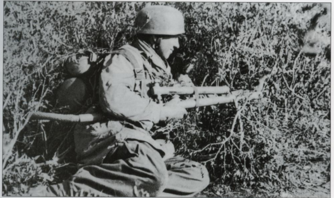
A paratrooper armed with the portable Flammenwerfer 41 flame-thrower. The upper cylinder carried the nitrogen propellant and the lower cylinder carried the fuel. A special protective suit was provided but was not often seen outside the training ground because it was cumbersome to use. This Fallschirmjäger wears only his olive green second model jump smock and jump trousers with the gravity knife pocket visible above the right knee.
