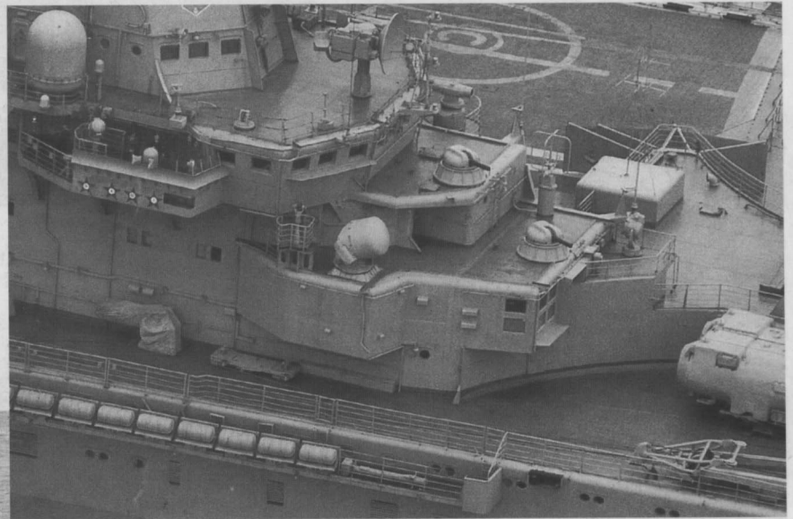
Starboard side amidships showing the Top Sail radar (in front of the mast) and Top Steer immediately behind it. One level down are the Head Light radars which are used in conjunction with the SA-N-3 Goblet SAM. The 'balls' in the centre of the island are Side Globe electronic warfare radomes.
