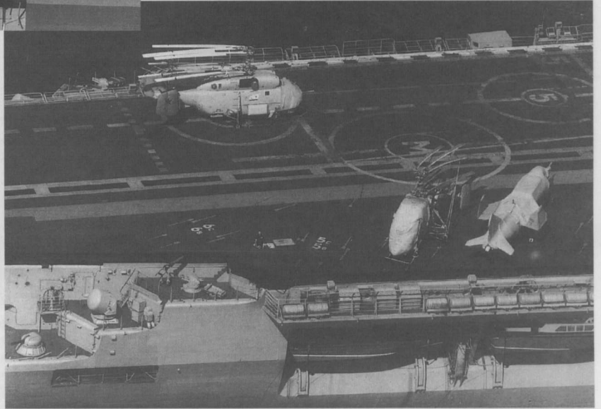
The Kiev's flight deck at the stern of the vessel. A Ka-27 Helix helicopter occupies launch position number "6" on the port side of the deck. At the bottom left corner of the picture is an AK-630 6-barrel Gatling gun and its fire control radar.
