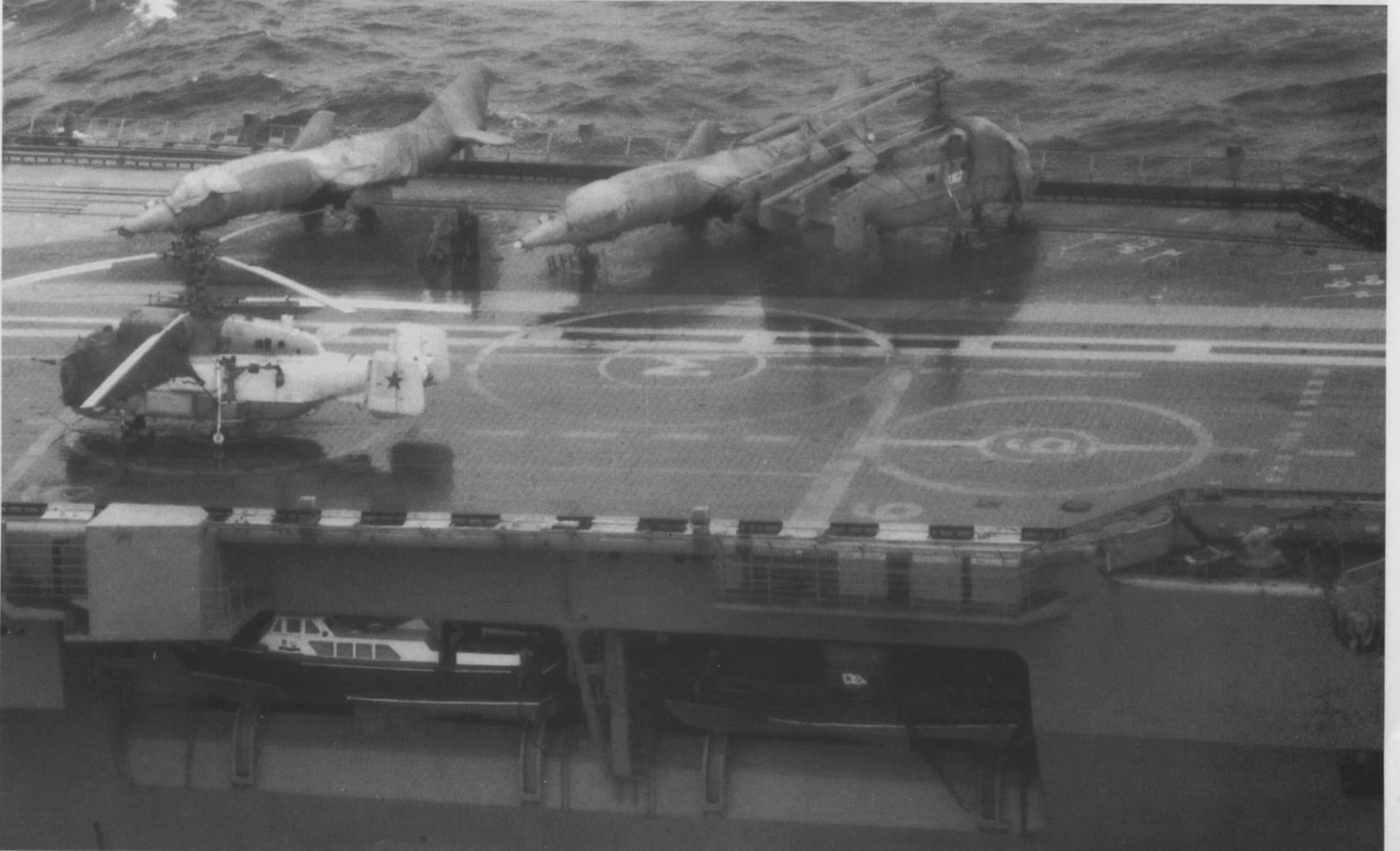
Rear flight deck detail on a wet day. The Helix, although still in its canvas 'night-cap', has sets of rotor blades extended. In the rear are two Forgers and a Hormone helicopter.
