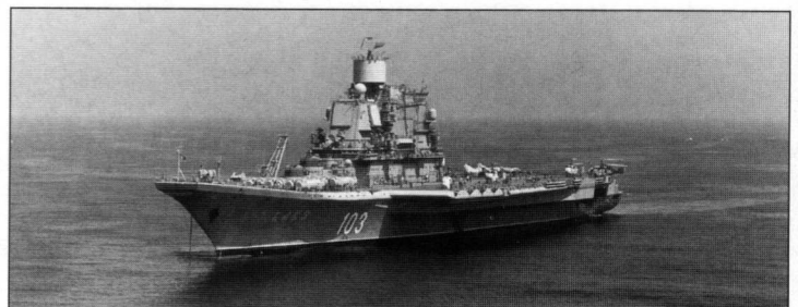
Lower: Three-quarter port shot of the Admiral Gorshkov showing the change to the bow at the waterline, the elimination of the port forward gun sponson and the obvious electronic changes.
