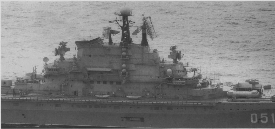
The Kiev's island showing electronic and weapon systems. Immediately to the left of the "0" in "051" is a slightly darker toned panel which covers the torpedo launchers.
