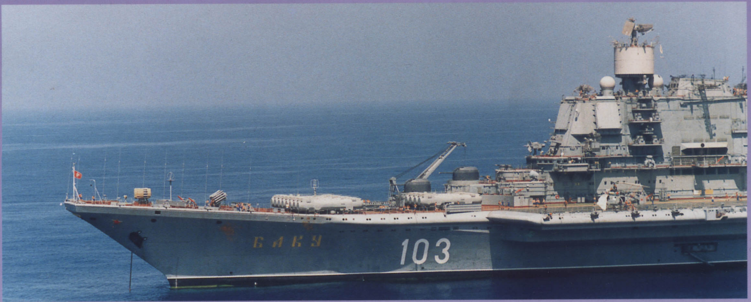
Forward port view of the Admiral Gorshkov. Differences in this section include: replacement of the RBU-6000 with the RBU-12000, replacement of the SUW-N-1 position with flush mounted SA-N-9 SAM, increased SS-N-12 complement, and two 100mm single gun mounts.
