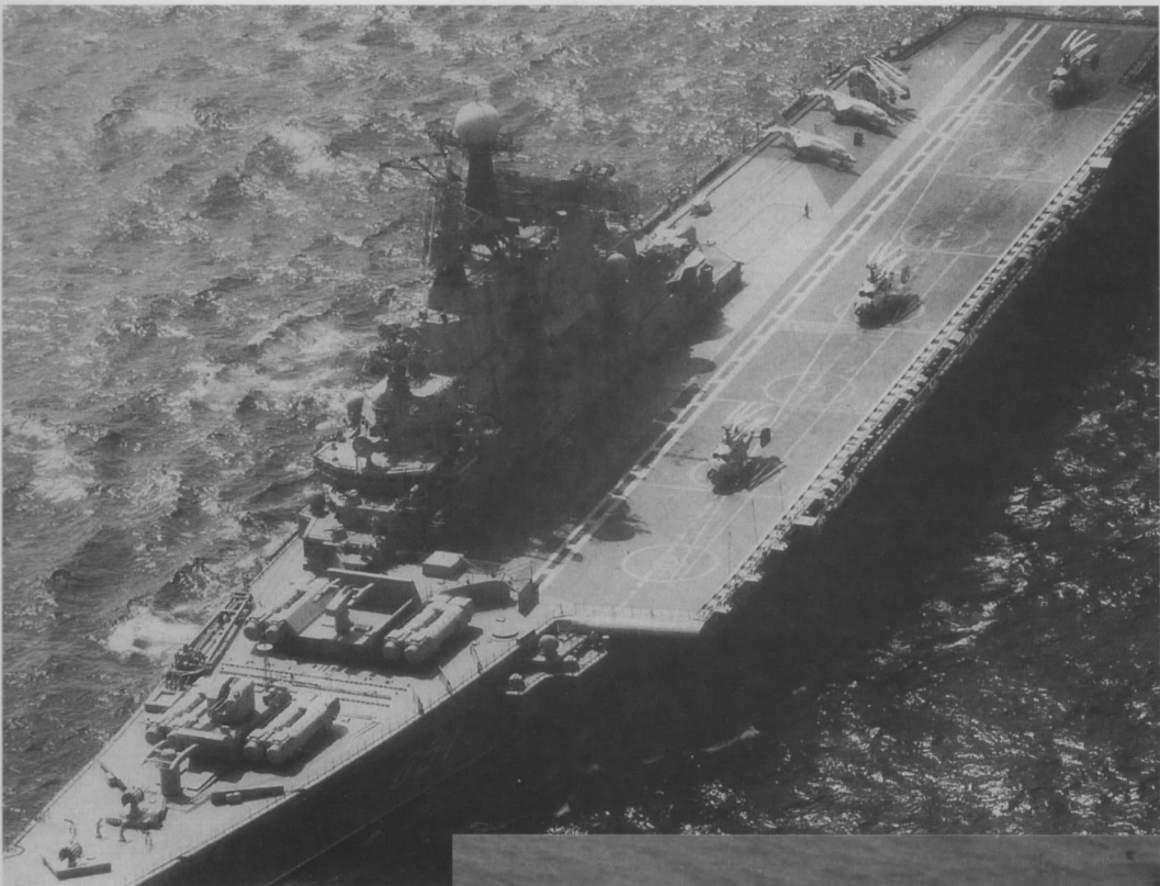
The Kiev showing its large island located on the starboard side. A comparison between Kiev class and U.S. carriers will show the absence of any deck launching or recovery equipment. Both the Helix and Forger are used in a VTOL mode only. The crewman walking forward of the Forger is just leaving the rear aircraft elevator.
