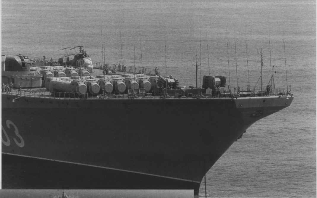
The Admiral Gorshkov's bow with her very impressive missile battery. The SS-N-12 has no reload capability, unlike the three earlier vessels which have eight missiles and eight reloads.
