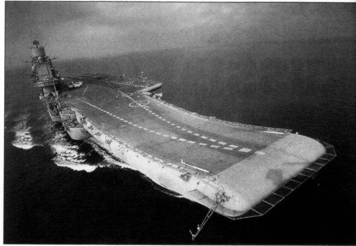
The ski-jump of the Admiral Kuznetsov is shown to advantage in this shot. It may have been intended to support the deployment of the Yak-141 Freestyle, as this aspect does not benefit aircraft without vectored thrust engines. (Sergey Skrynnikov)
