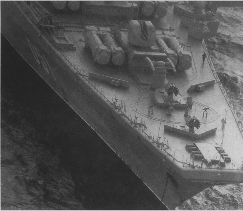
Close-up of Kiev's bow showing the Trap Door radar for SS-N-12 (in the retracted position), two RBU-6000 rocket launchers, SUW-N-1 missile launcher and twin 76.2mm guns between pairs of SS-N-12 Sandbox launchers. Also clearly visible are the tracks for the reloading dollies for the RBU-6000s.
