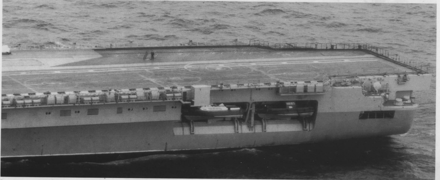
A photographic stroll down the port side of the Kiev. All fixed wing aircraft and helicopters have been stowed below deck. Note how the small launches are stored in their respective spaces under the deck at the stern, and how they are launched by sliding them down the tracks.
