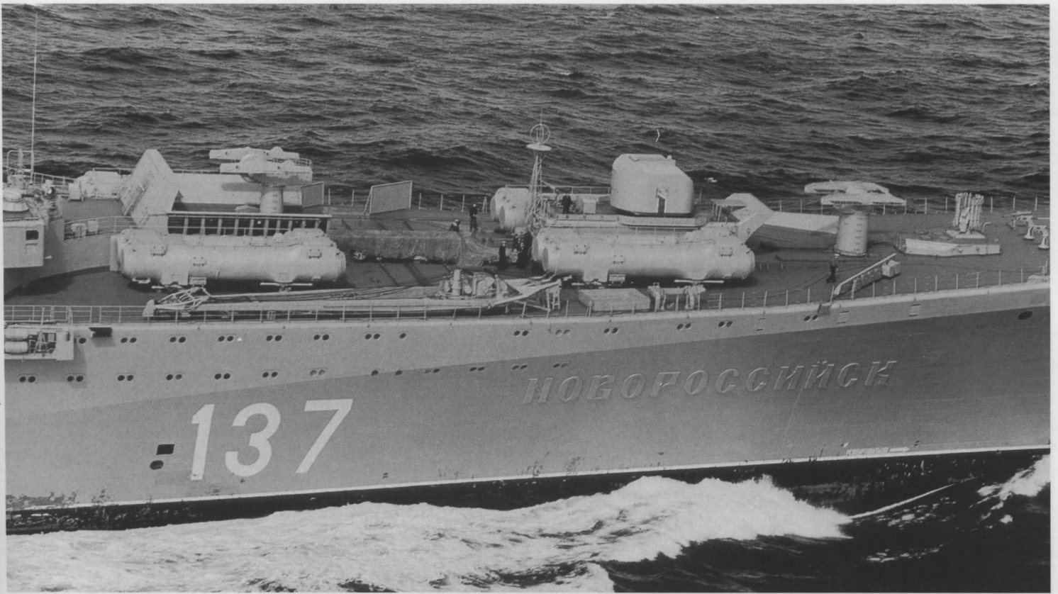
The business end of the Novorossiysk. The size of the SS-N-12 surface-to-surface missile launchers is best appreciated by comparing their mass to the diminutive sailors standing next to them.
