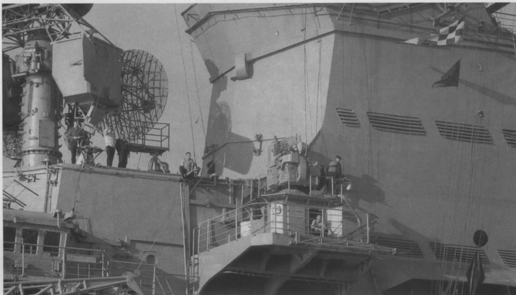
This photo shows some of the fire control radars located on the Kiev's island. At left is the Head Light system; in the center is one of two Pop Group systems. Of the Kiev class vessels, only the Kiev itself and the Minsk are equipped with Pop Group radar.
