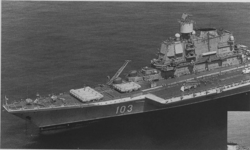
This aft island view shows two Sky Watch panels. Compare the clean look of this vessel with the other Kiev vessels. The SA-N-9 launchers can just be seen at the bottom of the picture directly under the figures. The helicopters are a Helix and a Hormone.
