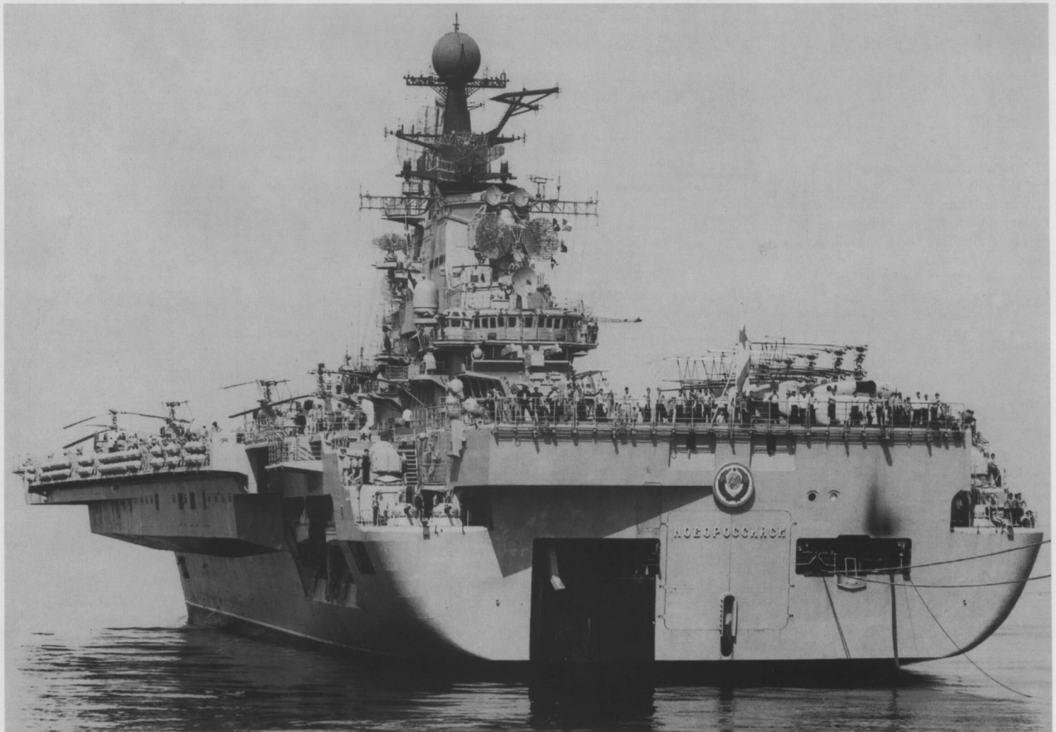
The Novorossiysk from the stern port quarter showing the VDS doors, the port-side boat launchers and a deck-full of happy sailors. Also visible are the four stern-mounted AK-630 ADMG's and the Helix helicopters on deck, some with their rotor blades folded back and secured.
