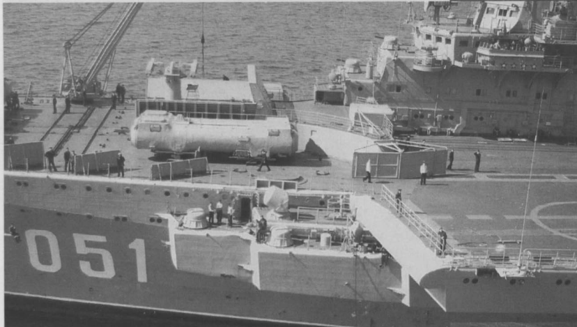
Close-up of the foredeck detail including the twin AK-630 and their associated radars mounted forward of and below the flight deck. Note the size of the wind baffles (at left) in relation to the men standing next to them.
