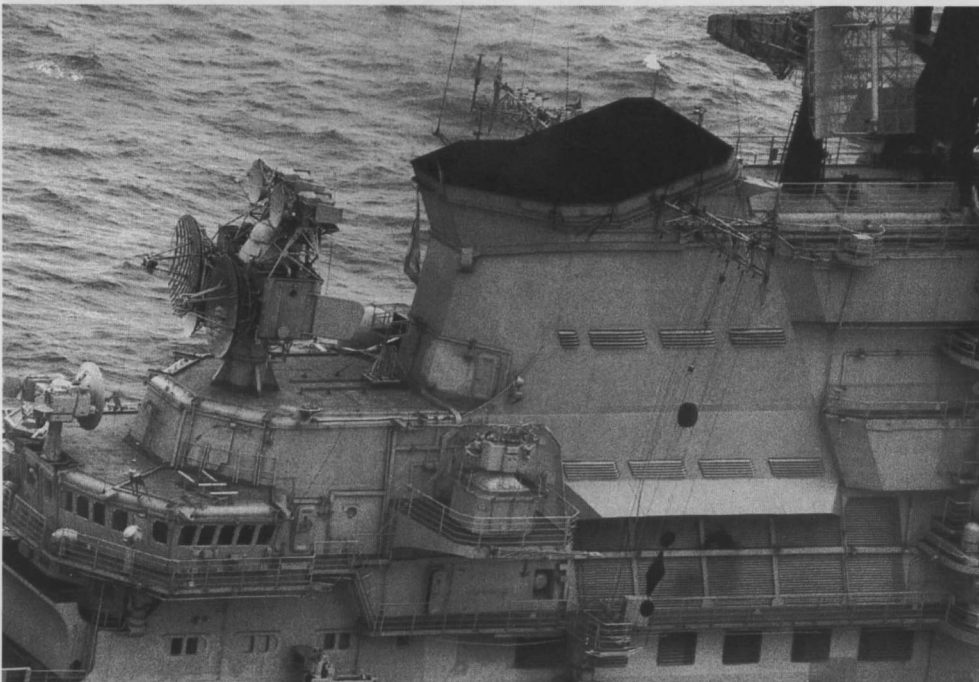
Climbing the radome ladder: (from bottom to top) Tee Plinth (electro-optical), two (horizontal) Bell Thump jammers, two (vertical) Side Globe EW radomes, two (horizontal) Bell Bash jammers, two more (vertical) Side Globes and, finally, Rum Tub ESM antennae.
