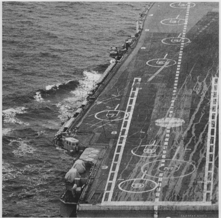
Stern area of the Kuznetsov's deck and rear weapon positions. To the rear of the two SA-N-11 mounts is the RBU-12000. To the front are the SA-N-9 missile silos. Half way along the deck are two AK-630 close-in defence weapons.
