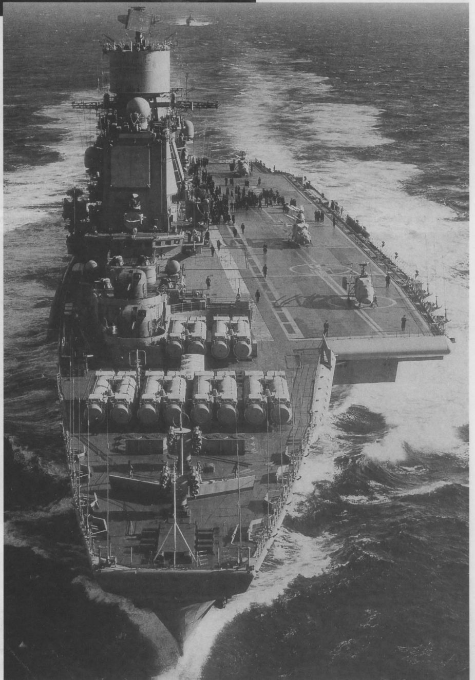
Weapon systems on the bow: Trap Door radar (retracted), two RBU-12000 ASW launchers, twelve flush-mounted vertical launch SA-N-9 launchers, four pairs of SS-N-12 launchers, two more pairs of SS-N-12 launchers, two 100mm guns and the re-configured AK-630 guns (now four) mounted in tandem pairs.
