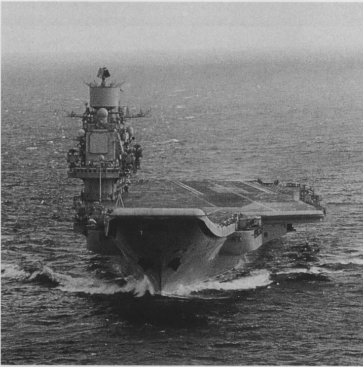
This view of the Admiral Kuznetsov from directly ahead shows the two forward weapon areas and some of the detail on the island. The flight deck, which measures 999 ft x 229.7 ft (304.5m x 70m), is well displayed here.
