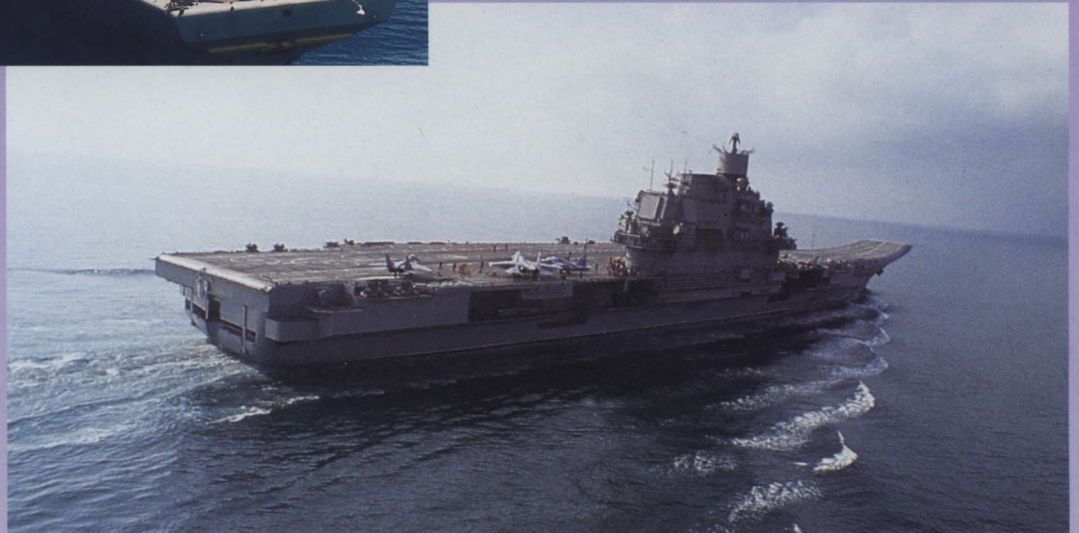
A distant view of the first true Russian aircraft carrier, the Admiral Kuznetsov (originally Leonid Brezhnev, then Tbilisi). Navalized Su-27K, along with other Russian ship-based aircraft such as the Su-25T and the MiG-29K, undergo flight tests from its deck. (Sergey Skrynnikov)
