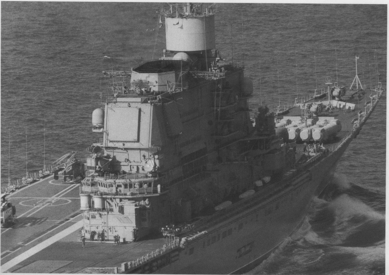
This aft island view shows two Sky Watch panels. Compare the clean look of this vessel with the other Kiev vessels. The SA-N-9 launchers can just be seen at the bottom of the picture directly under the figures. The helicopters are a Helix and a Hormone.
