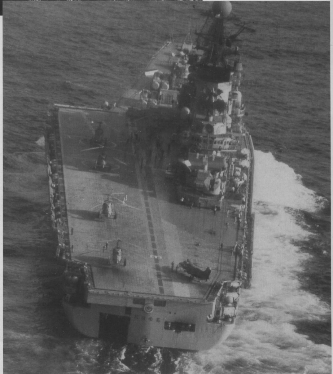
Stern view of the Kiev underway with four Helix preparing to launch. The small dark rectangle to the right is the opening for the stern mooring lines.
