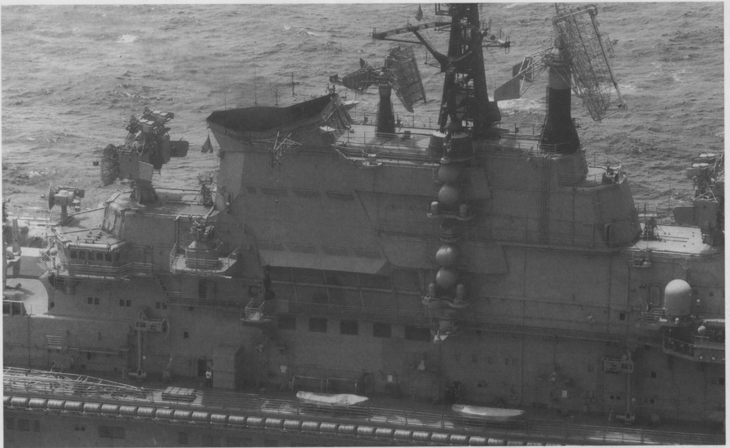
Starboard side amidships showing the Top Sail radar (in front of the mast) and Top Steer immediately behind it. One level down are the Head Light radars which are used in conjunction with the SA-N-3 Goblet SAM. The 'balls' in the centre of the island are Side Globe electronic warfare radomes.
