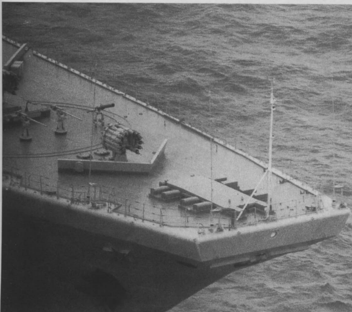
Forward of the RBU-6000 (a twelve-barreled rocket depth charge launcher) is the panel covering the Trap Door radar which is used for missile tracking and control for the SS-N-12 Sandbox.
