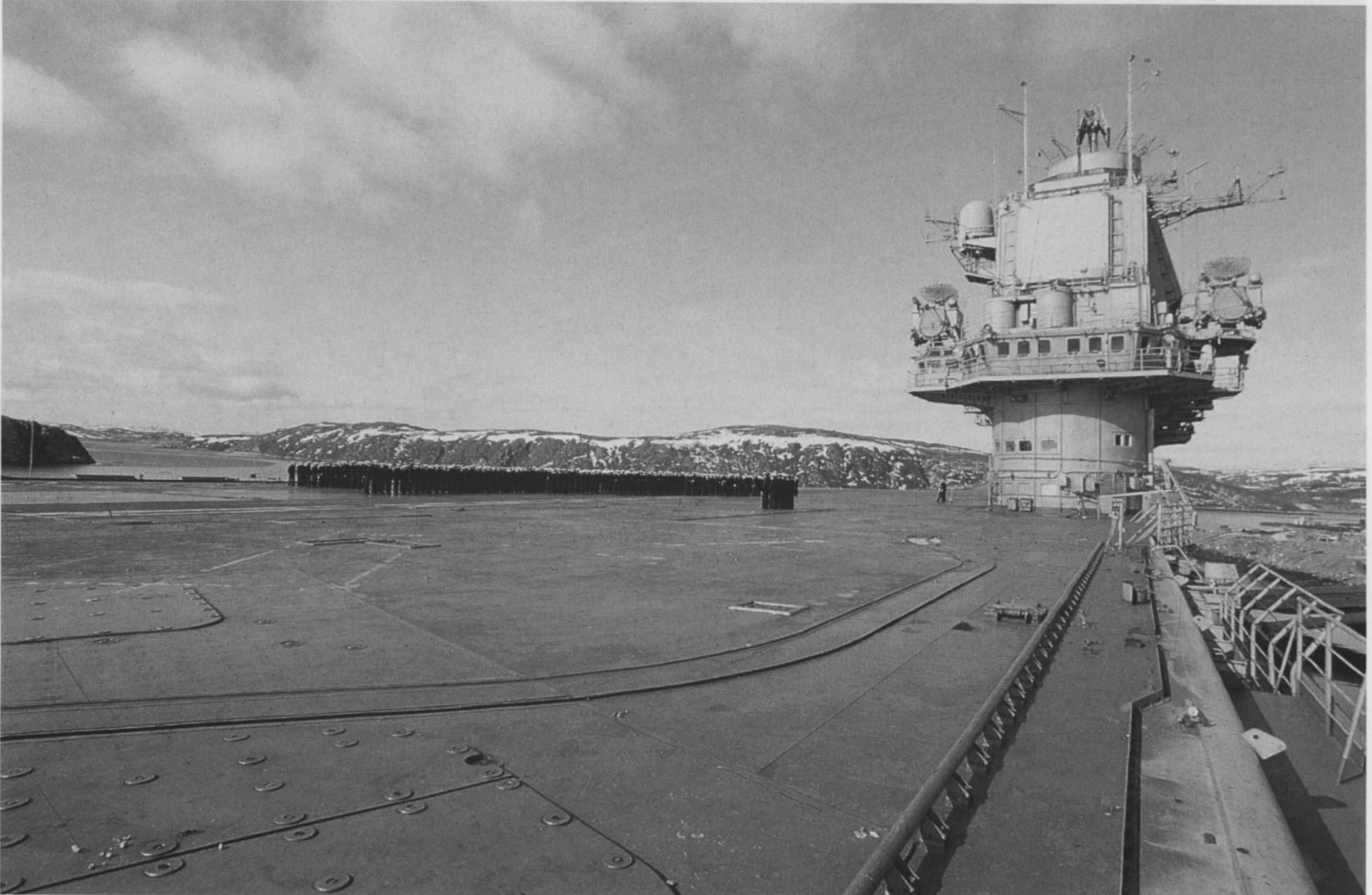
Unlike its busy Western counterparts, the Admiral Kuznetsov's deck is mostly used as giant parade ground for Russian seamen rather than for carrier landing operations. Note the Sky Watch planar phased array and the Cross Sword radars. (Pavel Gerasimov)
