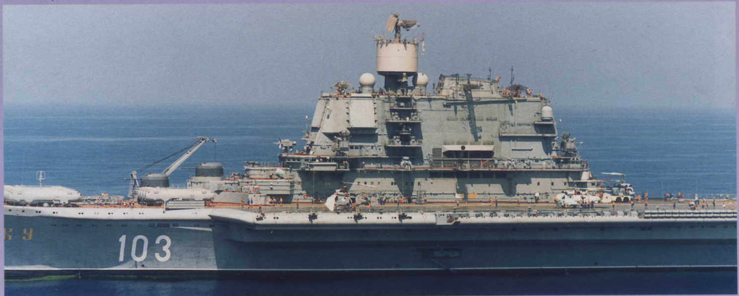
The Admiral Gorshkov's center section showing (from the top) Plate Steer radar, Cake Stand radar (resembling a large tub!), Low Ball SATCOM radomes (fore and aft of the main mast) and a flat Sky Watch 3-D planar phased array radar plate (immediately beneath the foremost Low Ball radome).
