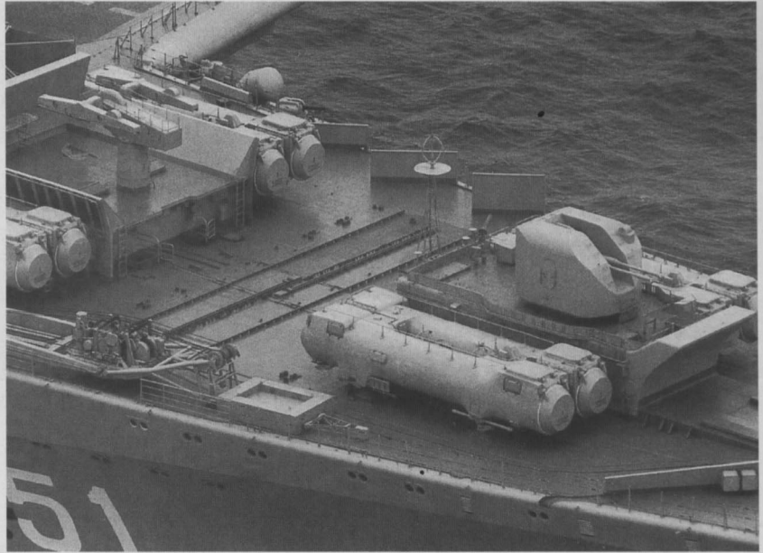
This close-up shows three of the Kiev's prominent weapon systems. Sandwiched between SS-N-12 Sandbox cruise missile launchers (range of 300 nautical miles) are (to the right) twin 76.2mm guns and (to the left) twin SA-N-3 Goblet anti-aircraft missile launchers (maximum range 55km).
