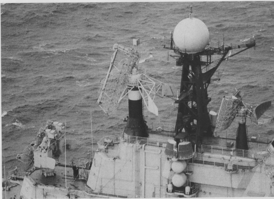
A view of Novorossiysk's forward island showing her electronic set. Seen here are (L to R) Head Light radar (fire control for the SA-N-3), Top Sail (3-D Air Search), Top Knot radar (TACAN) and Top Steer (3-D Air Search).
