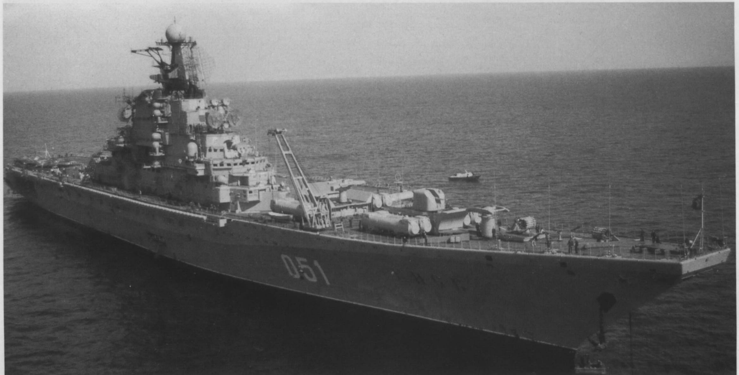
Starboard fore quarter showing the bulk of the weapon systems mounted there. The forward crane is erect, the starboard anchor is clear and there are ship's boats in the water.
