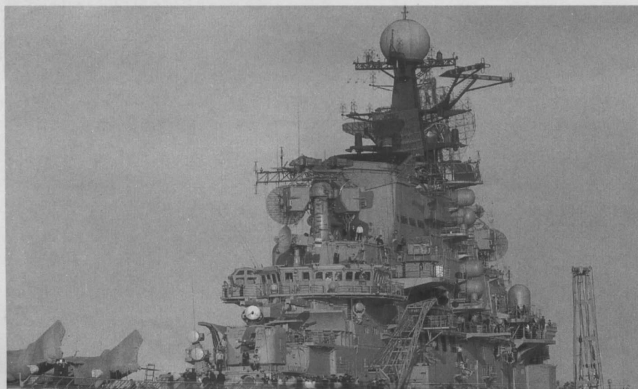
Interesting shot of the Kiev's starboard rear quarter showing (in the corner cut-out) a pair of AK-630 and their Bass Tilt radar and, forward of them, the (now empty) launch positions. Forward of the launch position, and extending to mid-island are would-be Soviet trapeze artists cleverly masquerading as painters.
