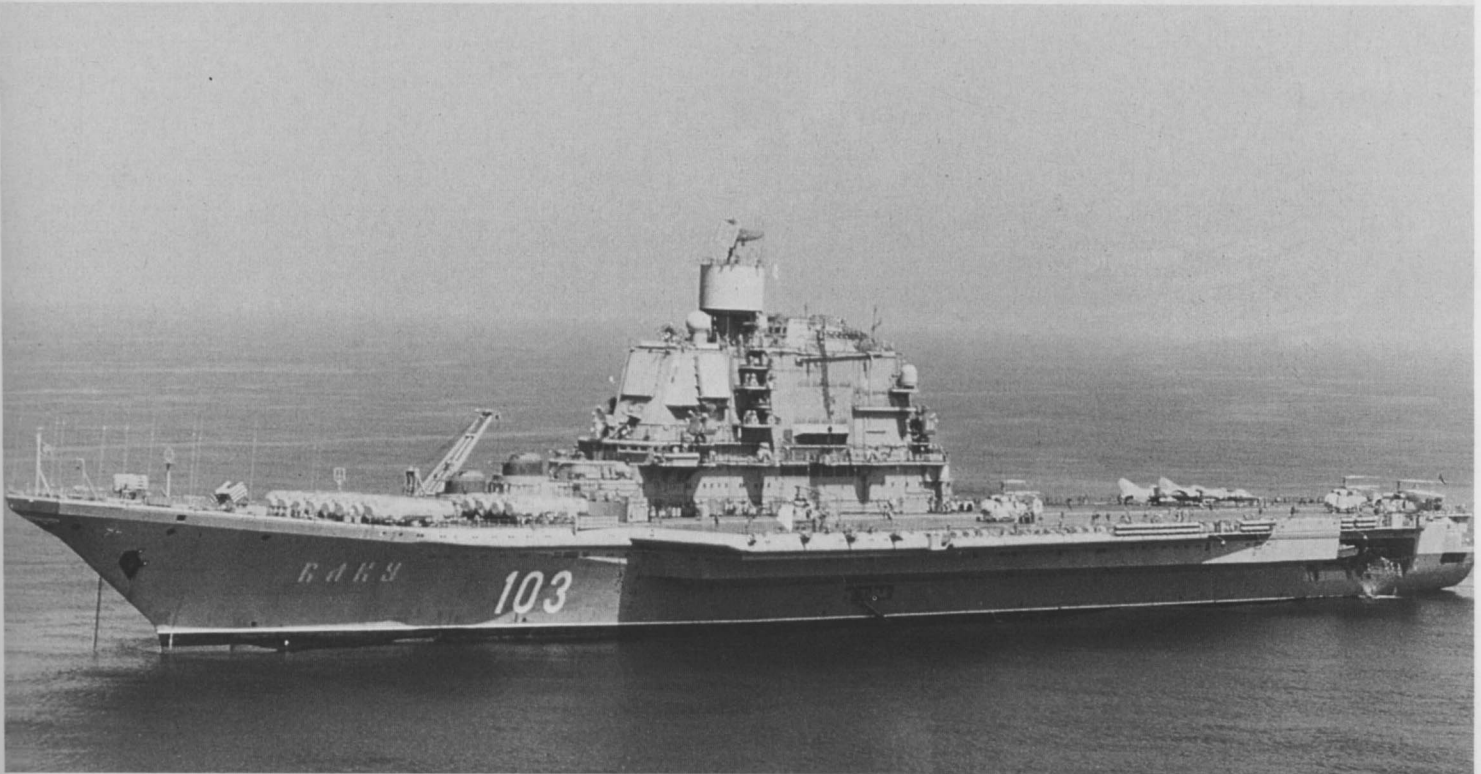
The Admiral Gorshkov (formerly the Baku, as the Cyrillic name on the hull reads) sitting at anchor. The difference in the superstructure between the other Kiev class vessels and this one is apparent by the briefest study of the electronic equipment with which it is equipped.
