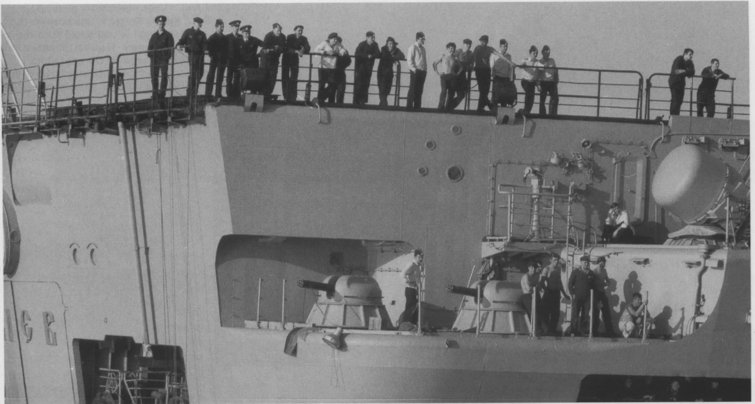
In this close-up view of the two rear starboard AK-630 30mm Gatling gun and their Bass Tilt radar, it is possible to see the six barrels of the rotating guns. The size of the guns and their turrets can be determined by comparing them to the sailor that is leaning against the one at right.
