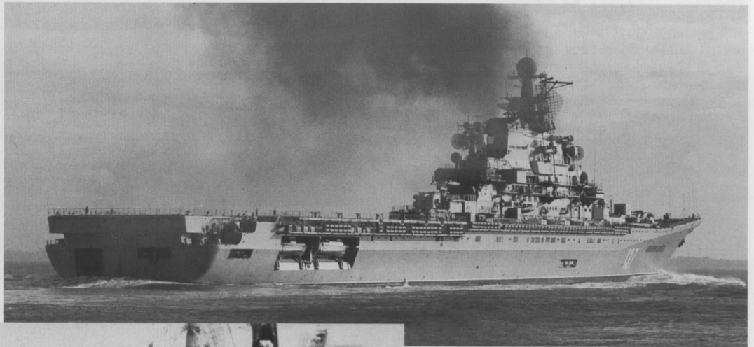
The Novorossiysk from the starboard-side stern. In this view the stern mooring port, boat launchers (one empty) and the collapsible life rafts are all visible. The Helix helicopters are not as small as normally thought, as is evident by a comparison with the crew members standing next to them.
