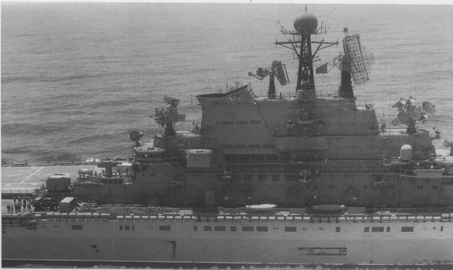
The Novorossiysk's island showing another difference with Kiev - the lack of Side Globe EW balls. In addition, as there are no SA-N-4 Gecko launchers (which would appear as a small circular plate on the starboard side next to the 76.2mm gun, right where the Gaz-66 truck is parked), there is no Pop Group radar mounted below and forward of the Head Light radar. (See earlier Kiev shots for comparison). Note that the aft aircraft elevator is lowered.
