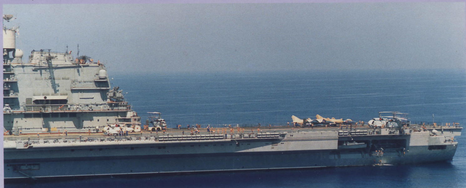
Rear island and deck view of the Admiral Gorshkov. The 76.2mm gun, the SA-N-3 launcher, the flush mounted SA-N-4 launcher and all their associated electronic fittings are not here; the only weapon system to be found is the vertical launchers of the SA-N-9 and its Cross Sword radar.
