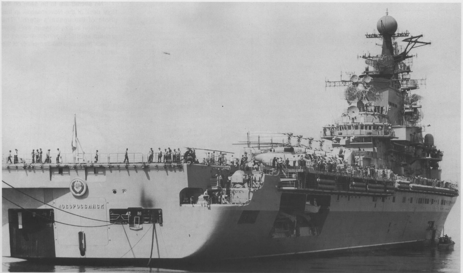
The Novorossiysk from the starboard-side stern. In this view the stern mooring port, boat launchers (one empty) and the collapsible life rafts are all visible. The Helix helicopters are not as small as normally thought, as is evident by a comparison with the crew members standing next to them.
