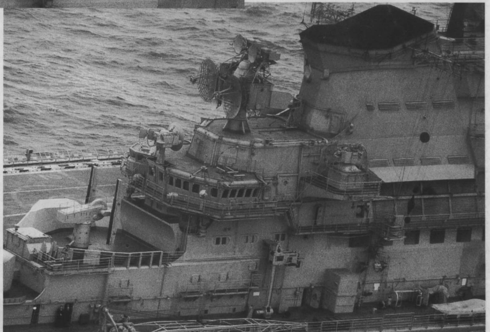
Forward of the funnel is Top Steer, an S-band 3-D system used for air control. Even with the funnel rear and down one level is the Pop Group radar which is used to control the SA-N-4 Gecko SAM.
