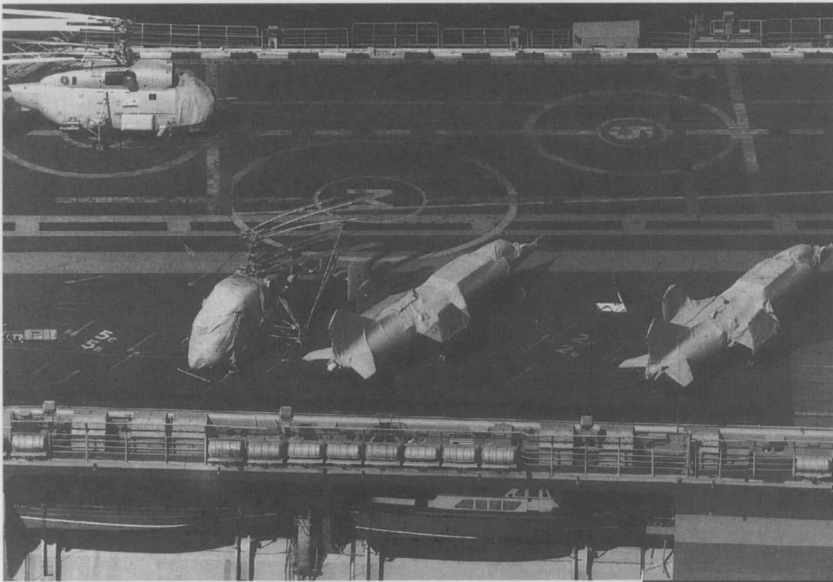
Flight deck details including a Helix helicopter on the flight deck and a Hormone and two Forgers to the starboard of the safety line. The Forgers are completely wrapped in tarping. The two ship's launches are mounted under the deck (bottom).
