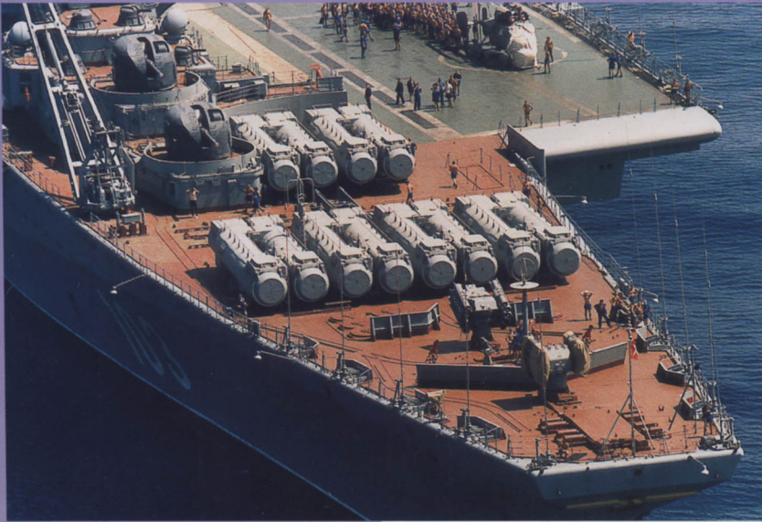
Forward weapon positions of the Admiral Gorshkov. Note the absence of the weapon sponson, the single wind deflector and the Hormone helicopter. Each of the 100mm gun barrel caps has a little red star on it. Note also that the leading edge of the flight deck has been extended and is rounded.
