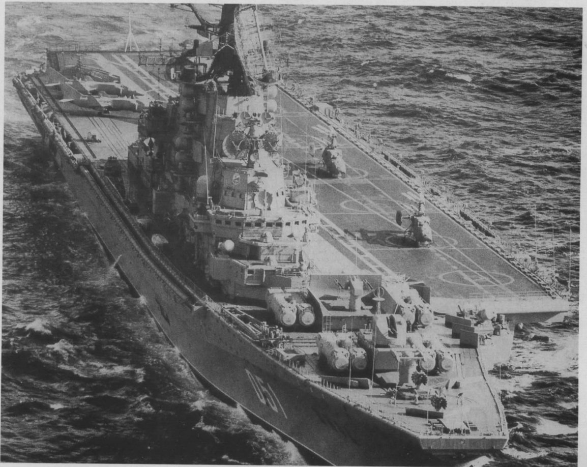
Three Helix on the flight deck being readied for flight. This view also clearly shows the AK-630 30mm six-barrel Gatling anti-aircraft guns (one in the lower right corner of the picture and the other two immediately behind the left pair of Sandbox missile launchers).
