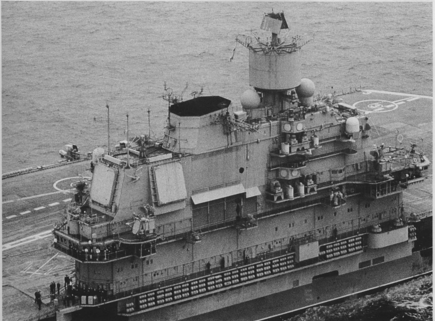
Overall view of the starboard side of the island. Topping the mast are the Plate Steer array atop the Cake Stand. The Big Ball SATCOM domes and the Sky Watch phased array are also shown.
