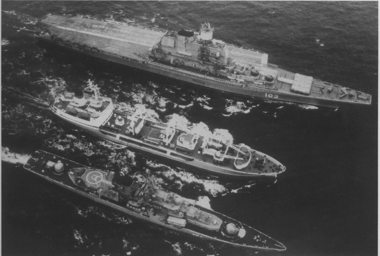
The Admiral Gorshkov and a Sovremenniy class destroyer taking on fuel from a Boris Chilikin class fleet replenishment vessel. The Sovremenniy is an anti-ship vessel which has adequate anti-air, but minimal ASW, capability.
