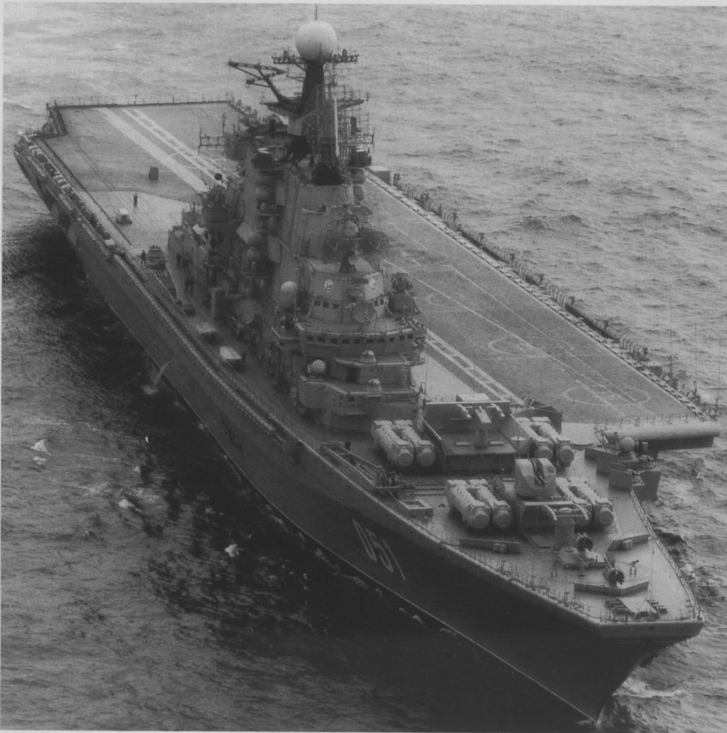
The Kiev 'clean' with no air visible on deck. Weapon systems on the bow (from bow aft) include: F-6000 (x2), SUW-N-1 launcher, 76.2mm gun mount sandwiched between two pairs of SS-N-3 Sandbox surface-to-surface cruise missiles, and SA-N-3 Goblet missile launcher between another pair of Sandbox launchers.
