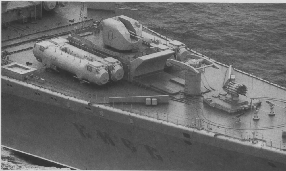
Forward of the 76.2mm gun is the twin SUW-N-1 launcher. This weapon is an unguided solid fuel rocket similar to the FROG-7 (Free Rocket Over Ground) used by the Soviet Army.
