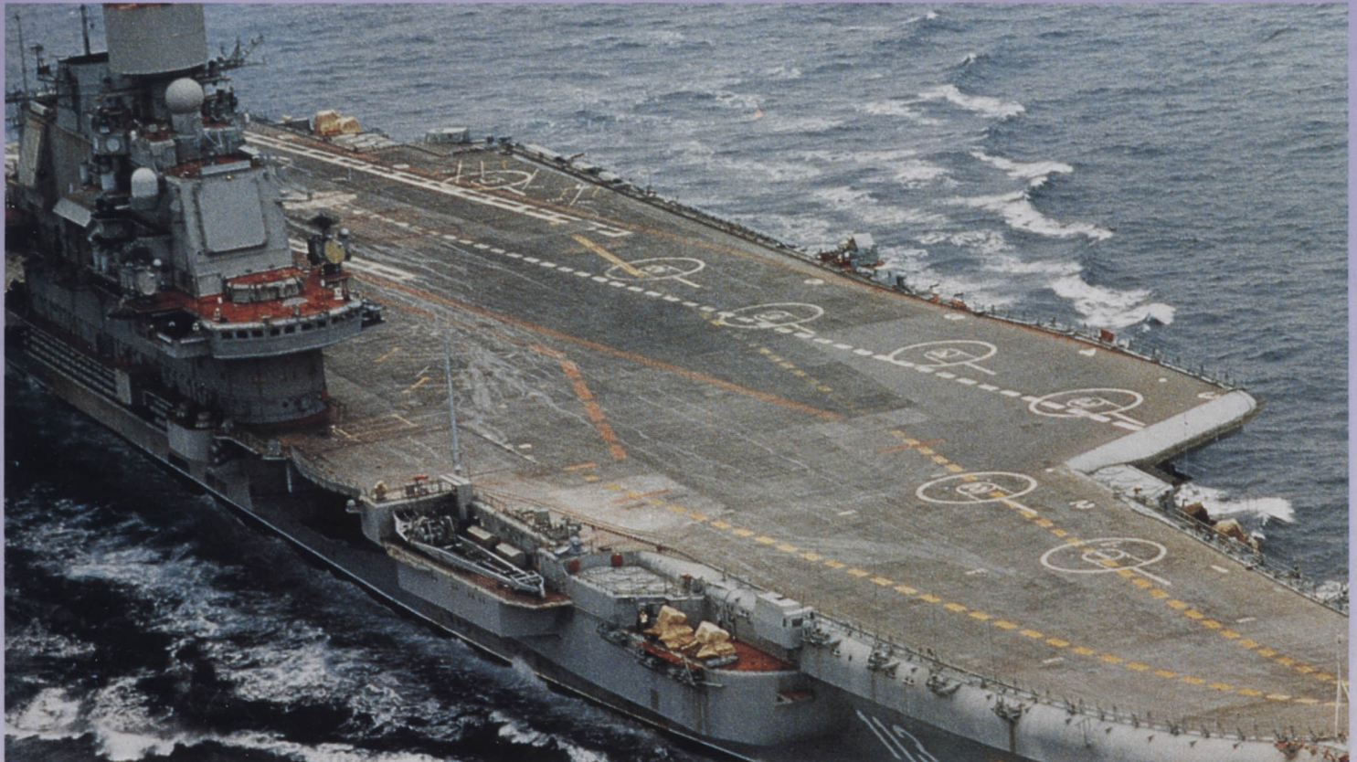
Fore deck of the Admiral Kuznetsov showing the SA-N-11 with canvas weather covers, SA-N-9 missile silo covers, 20-metre crane and island details. The Cross Sword radars are visible on either side of the Sky Watch array.
