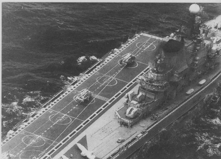
Overhead view of the flight deck area showing deck markings, Helix helicopters with rotors folded and the rear crane in the stowed position.
