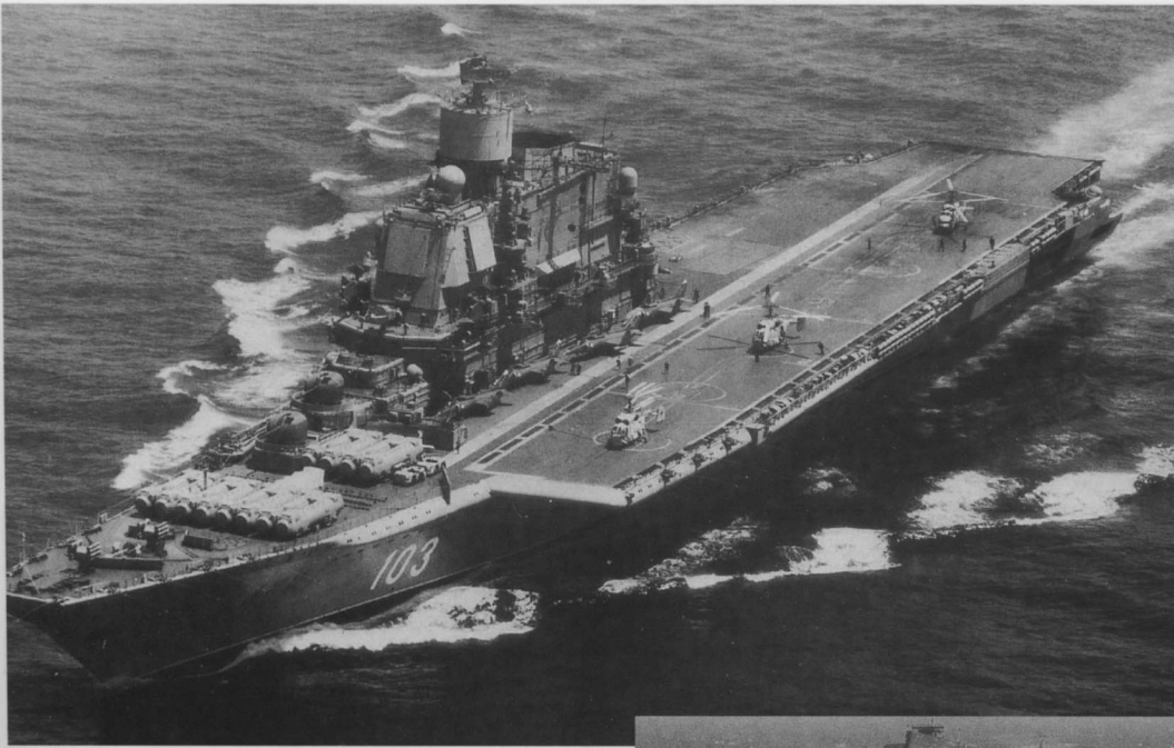
This shot clearly shows the new array of the SS-N-12 launchers, the new guns and the absence of the port bow gun sponson. There is also only a single wind deflector forward of the flight deck.
