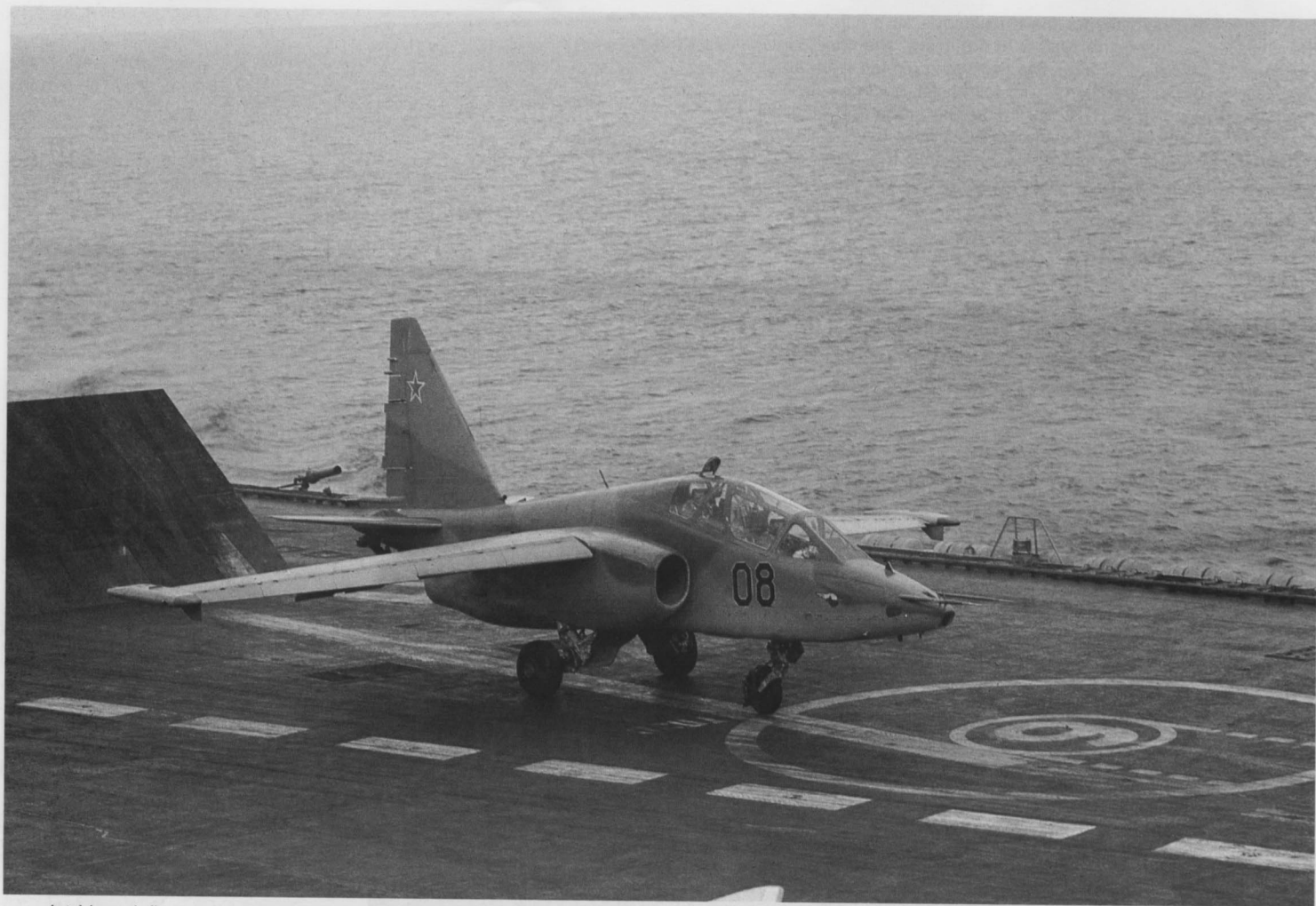
Jet blast deflector shields are raised behind a Su-25T Frogfoot while it runs up its engines. The engine exhausts are deflected by these shields measuring 8m by 4m. The presence of such shields are essential for the safety of the flight deck crew. (Sergey Skrynnikov)
