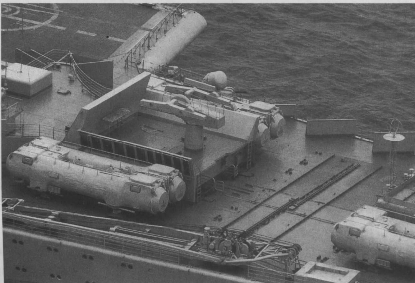
Close-up of the twin SA-N-3 Goblet launchers. Note the blast shields and the three vertical panels to the right of the photo which are wind baffles for the leading edge of the flight deck.
