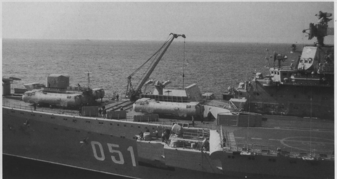
A variety of work is being performed in this photo of the Kiev, some of it involving the use of the forward crane. Of particular interest in this shot is the way the SA-N-3 Goblet launcher has been pointed to the side.
