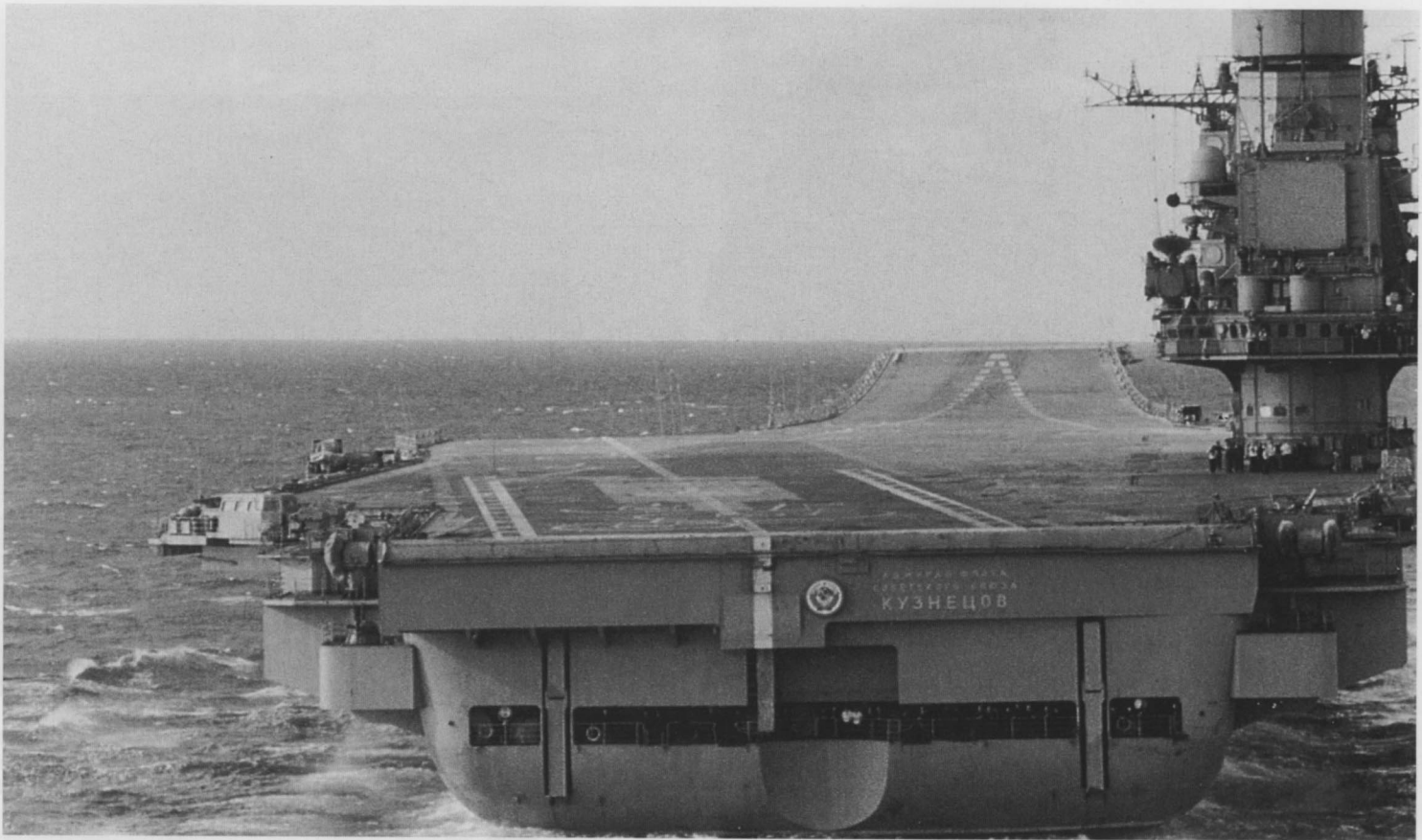
Close-up of the stern of the Kuznetsov. The small size of the island is apparent in this view. Weapon systems seen on the port side stern are: AK-630, RBU-12000 and two SA-N-11.
