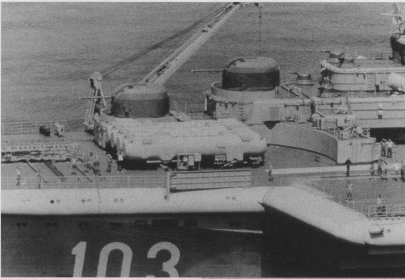
Close-up of SS-N-12 Sandbox launchers and two 100mm gun mounts. The 100mm gun has a range of about 9 miles (15,000m) and is controlled by Kite Screech radar. SS-N-12 is an advanced version of the SS-N-3 Shaddock which uses the Trap Door radar, recessed in the forecastle on the Kiev class ships.
