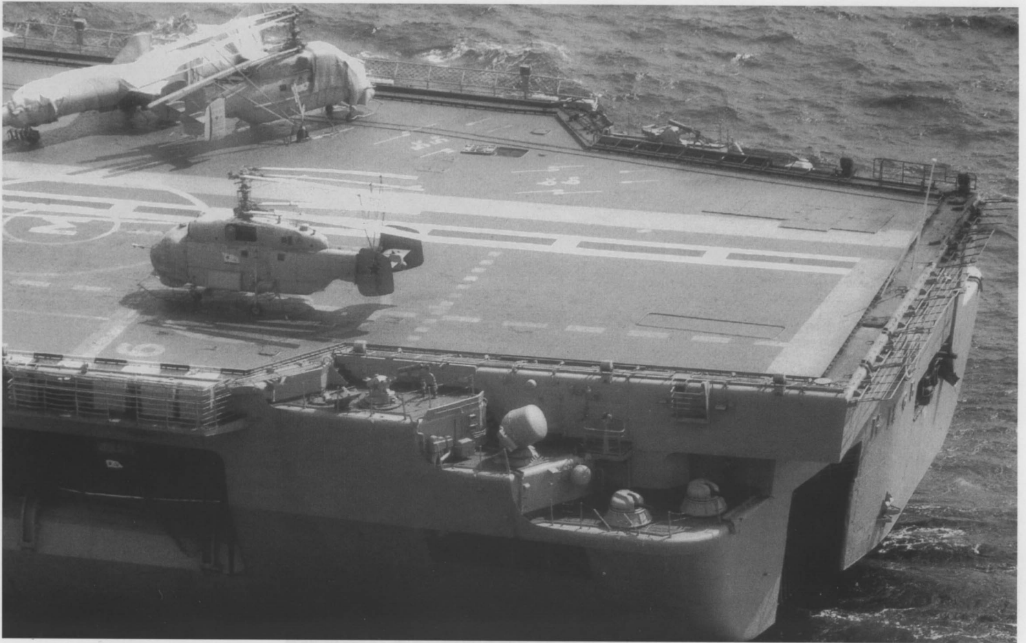
Details of the rear flight deck. The variety of painted markings on the deck are noteworthy. Also interesting is the railing fitted along the edge of the rear of the flight deck at the stern of the ship. It can be folded down to accommodate the activity of aircraft and then restored to an upright position.
