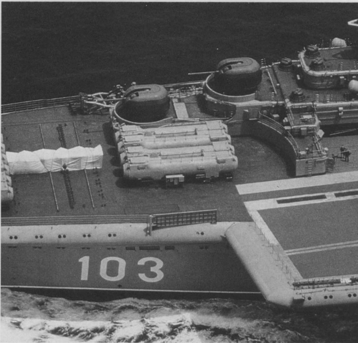
The two single 100mm gun mounts and four of the SS-N-12 Sandbox missile launchers located on the foredeck of the Admiral Gorshkov comprise the main subject of this photo of number "103". Also clearly shown is the extended leading edge of the flight deck.
