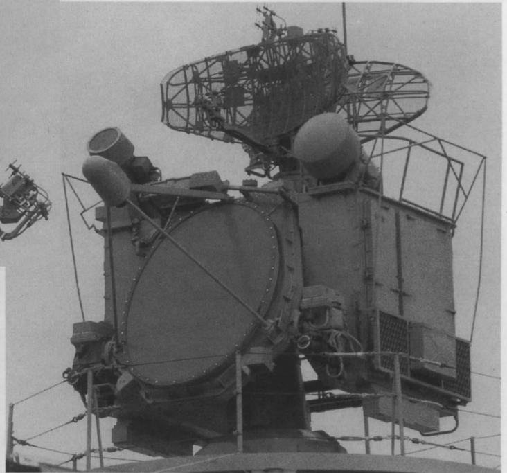
Cross Sword radar, used for fire control of the SA-N-9 SAM, as seen on the Admiral Gorshkov and the Admiral-of-the-Fleet Kuznetsov. This radar represents the latest in Russian technology and did not have an easy birth. Numerous problem areas delayed its introduction, and it is still not known if it will perform as intended.
