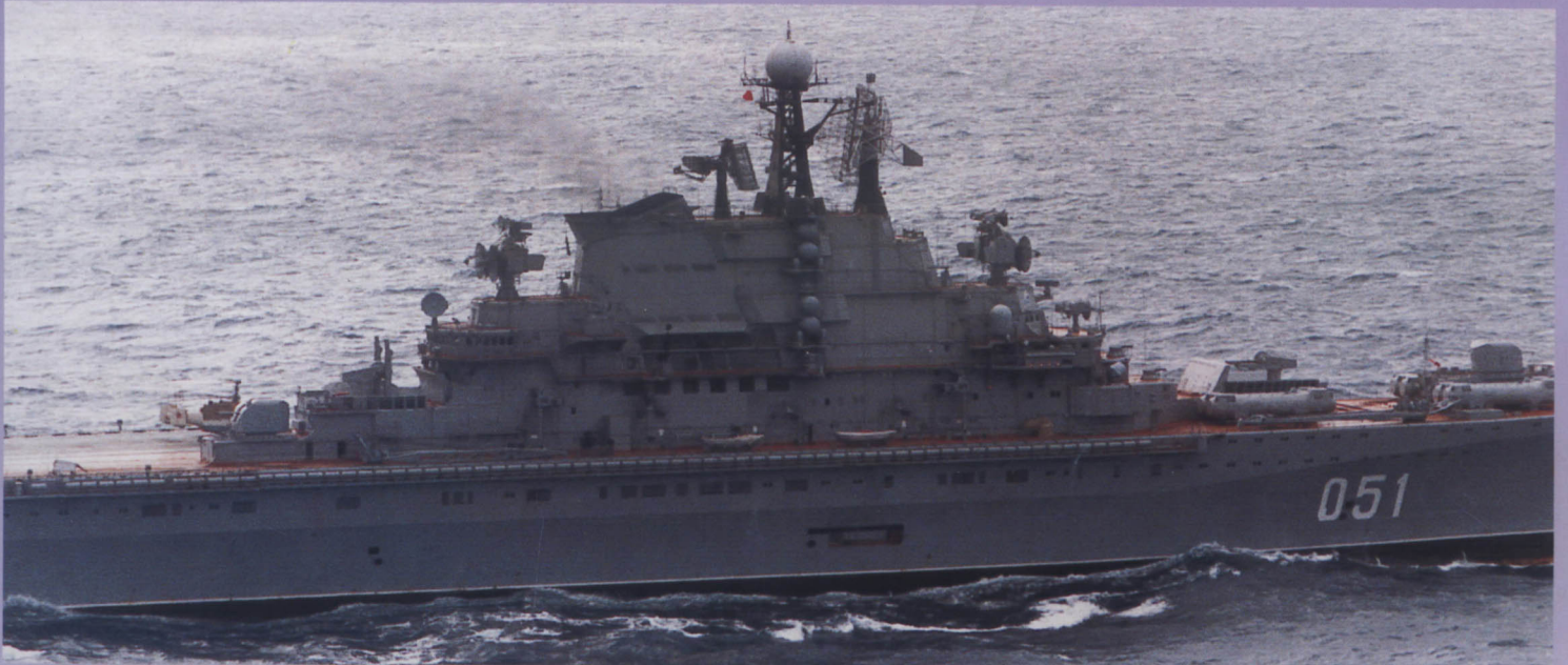
A walk up the starboard side of Kiev showing the relatively clean stern and the heavy grouping of weapon systems on the bow. Just to the left of the number "051" is the door covering the 533mm torpedo launchers.
