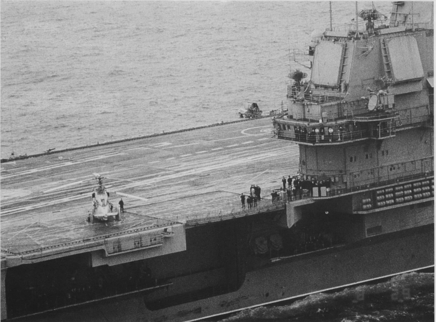
Flight deck aft of the island showing a Helix, the SA-N-9 silo and electronic fit on the island. The Cross Sword fire control radar is clearly visible.
