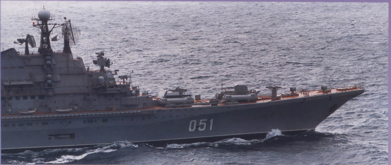
A walk up the starboard side of Kiev showing the relatively clean stern and the heavy grouping of weapon systems on the bow. Just to the left of the number "051" is the door covering the 533mm torpedo launchers.
