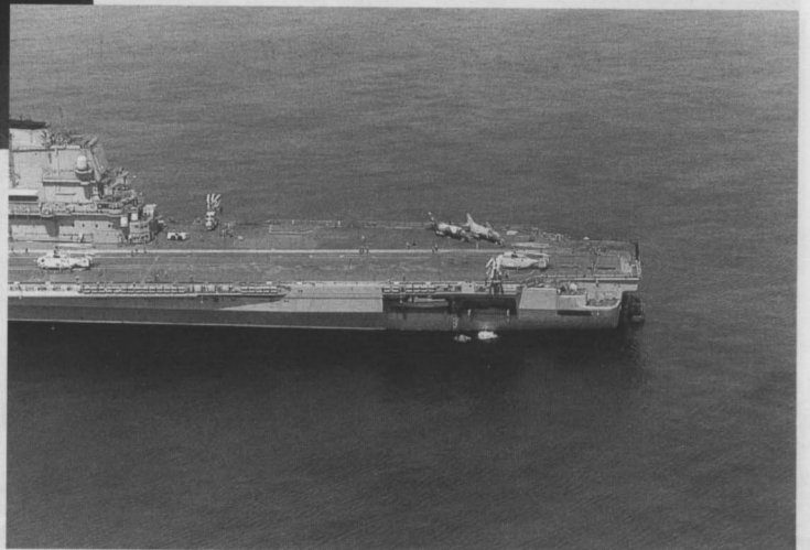
Overall shot of the Admiral Gorshkov's stern showing the increased deck area aft of the island provided by the removal of the gun turret and SAM launcher.
