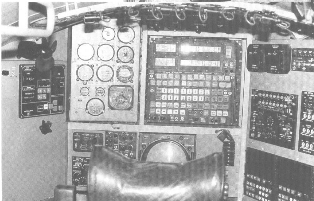
The navigator station is located in the rear part of the hermetic compartment which forms the crew's cabin. The navigator faces the rear of the aircraft. (Piotr Butowski)
