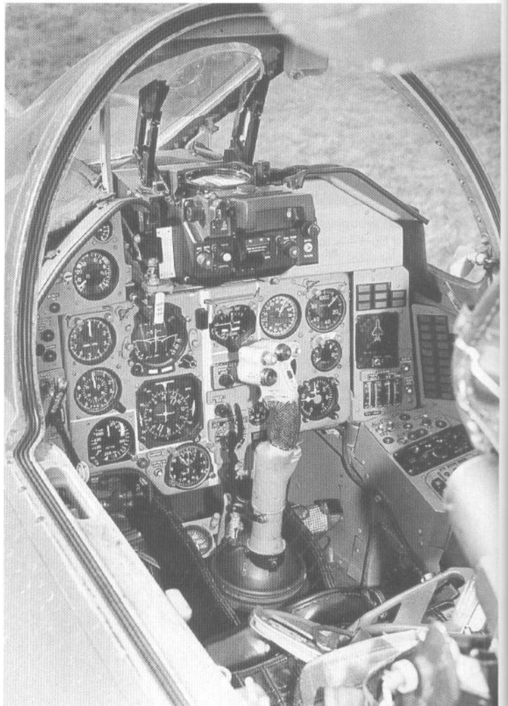
The pilot's cockpit in "humpback" versions of the Su-17 (the cockpit of Su-22M4K is in the picture) is much wider and more comfortable than in previous versions. (Piotr Butowski)
