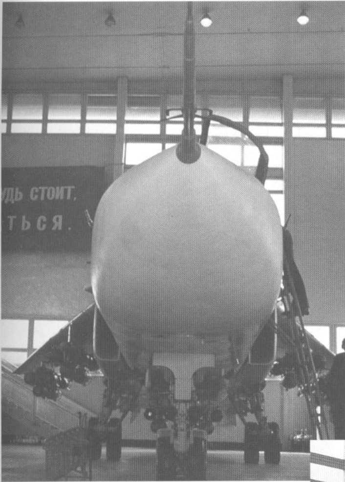
A Kh-58 (AS-11 Kilter) anti-radiation missile under the Su-24MK Fencer-D. (Piotr Butowski)
