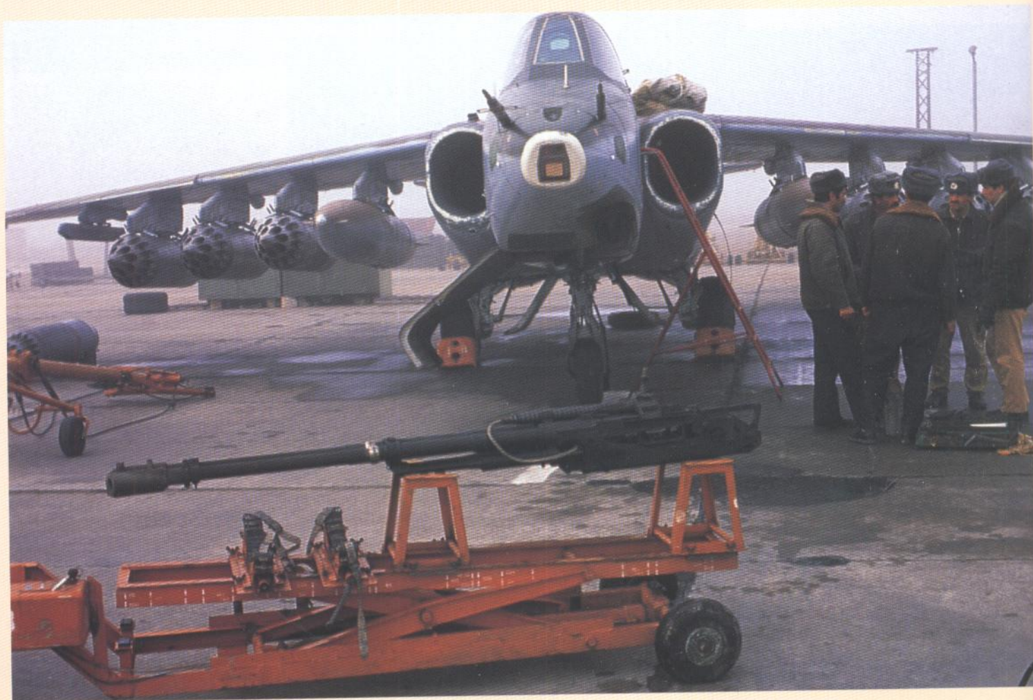
A twin-barrel 30mm cannon dismantled from the fuselage of a Su-25. (Piotr Butowski)
