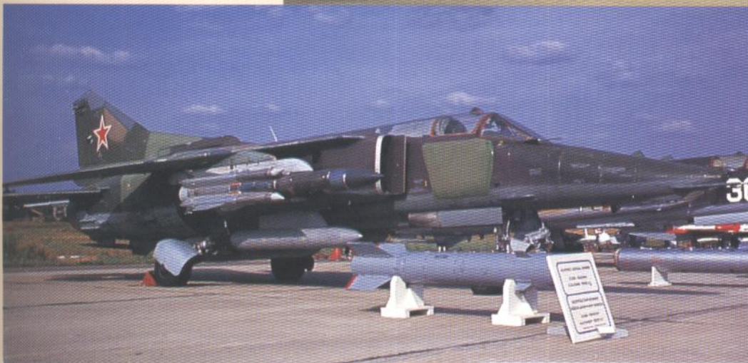
MiG-27K armed with a Kh-31P anti-radiation missile. (Protr Butowski)
