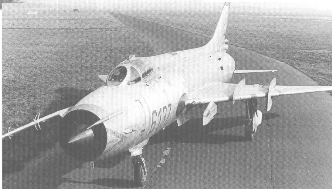
The Su-7 Fitter-A aircraft has been chosen by Sukhoi's team as the basis for the new design, the Su-17 Fitter-B. The wings have been redesigned into a variable geometry model with movable ends. The changes in external appearance include: the cockpit canopy opening upwards instead of sliding back, as in the Su-7; a fairing between the pilot cabin and the tailfin; and some minor changes in the arrangement of aerials. Also two big armament-carrying beams have been suspended under each wing. In 1972, two Soviet VVS regiments were equipped with the Su-17 aircraft.
