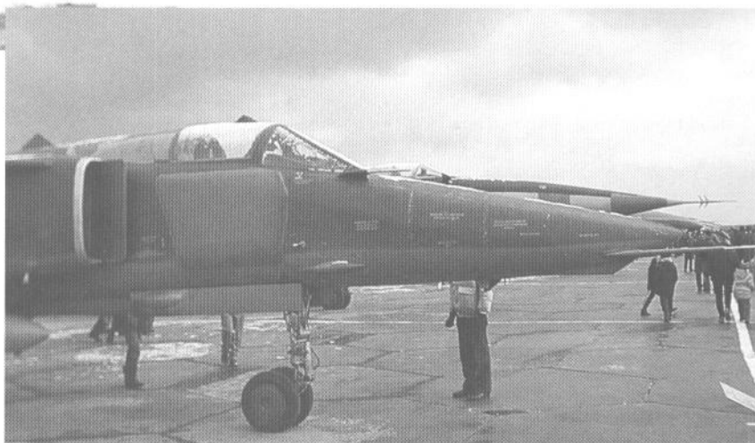
The nose of the MiG-27 aircraft with the additional armor plate clearly seen on the side of the cockpit. (Piotr Butowski)
