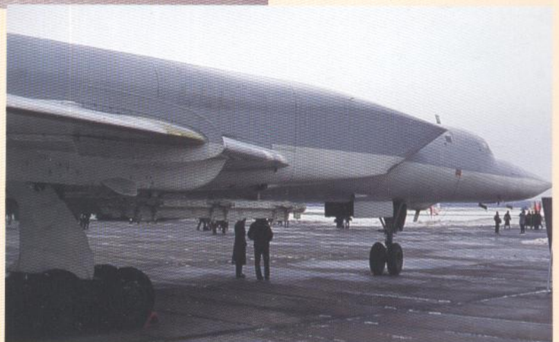
Tu-22M3 Backfire-C is equipped with new Kuznetsov NK-25 engines with increased thrust, therefore the air intakes are bigger, their form being similar as in MiG-25 Foxbat interceptor. (Piotr Butowski)
