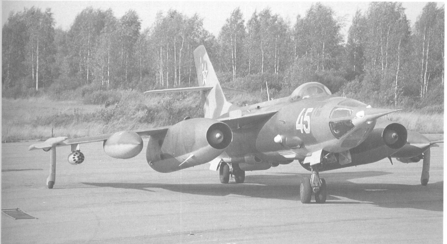
Yak-28PP Brewer-E electronic warfare aircraft. A distinguishing feature of this version is the presence of many aerials on the fuselage. (Piotr Butowski)
