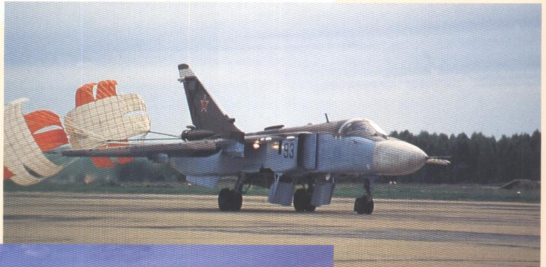
Note not only the different camouflage scheme of this Su-24M but also the opened aerodynamic brakes in front of the landing gear under the fuselage. There are also chaff/flare dispensers installed in the aerodynamic fences on the upper surface of wings. (Piotr Butowski)
