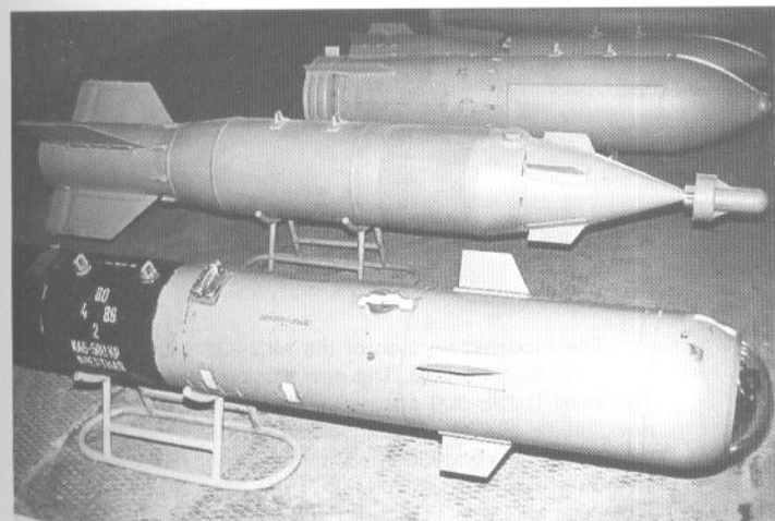
FAB-500M-62 (model 1962), a standard Russian demolition bomb (in the foreground), BetAB-500ShP bomb designed to destroy concrete fortifications and runways (next in line) as well as FAB-500ShN bomb (third in the row). (Piotr Butowski)
