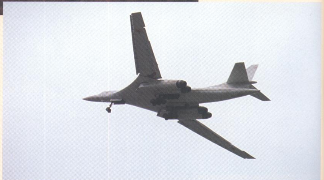
A Tu-160 prior to landing: wing sweep angle set at 20°, and landing gear, flaps and slots lowered. (Piotr Butowski)
