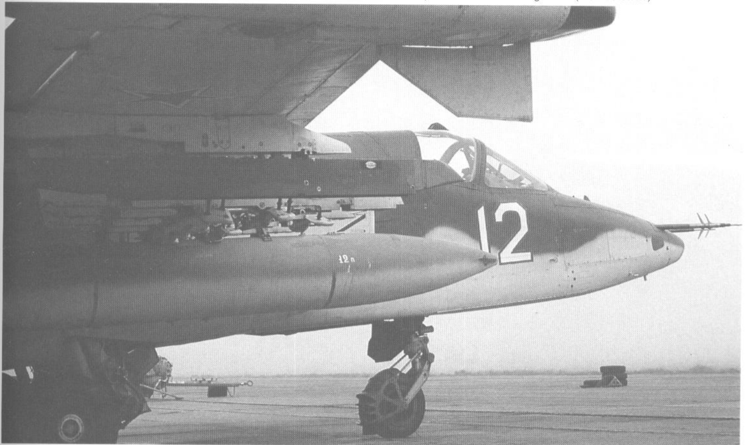
This vertical plate on the wing-tip fairing is not an aerial. It has been installed to obscure the landing floodlights and to protect the pilot's eyes from being blinded. (Piotr Butowski)
