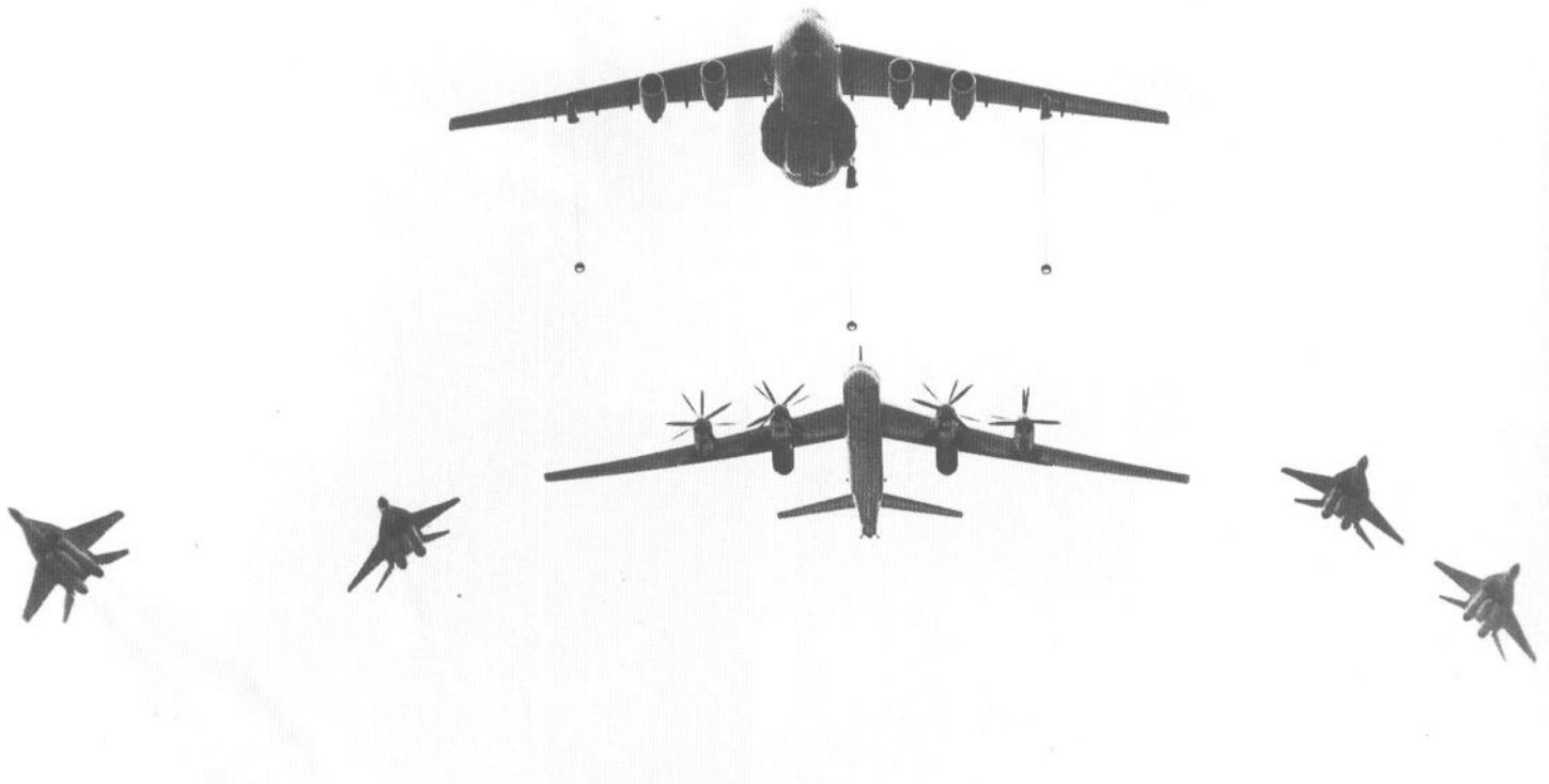
This Tu-95MS, escorted by Su-27s, is being refuelled in flight by an Il-78 Midas flying tanker. (Piotr Butowski)
