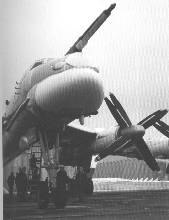
The nose of the Tu-95MS Bear-H aircraft with Short Horn navigation and bombing radar antenna. The in-flight refuelling probe is seen above. (Piotr Butowski)
