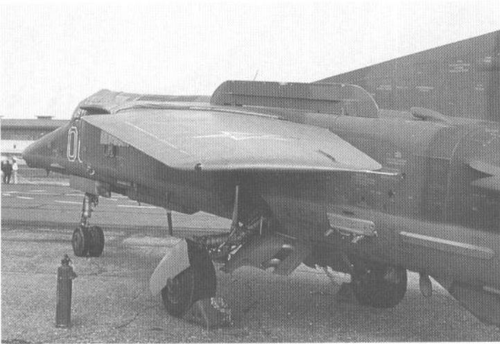
ASO-2 chaff/flare dispensers installed on the back of the MiG-27 fuselage. (Piotr Butowski)
