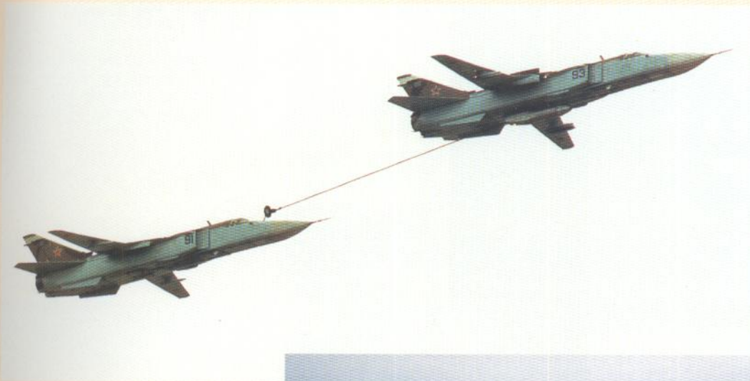
A Su-24M is refuelled in air by another of the same aircraft using the UPAZ universal refuelling device.
