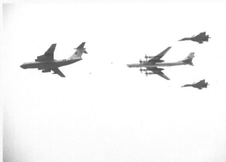
This Tu-95MS, escorted by Su-27s, is being refuelled in flight by an Il-78 Midas flying tanker. (Piotr Butowski)
