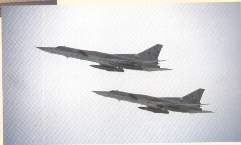
Two Tu-22M3 Backfire-C bombers. Note the different versions of Kh-22 (AS-4 Kitchen) stand-off missiles carried by both aircraft. The first one carries the anti-radar version, while the second one is equipped with missiles with programmable trajectory and an integral navigation system. (Piotr Butowski)
