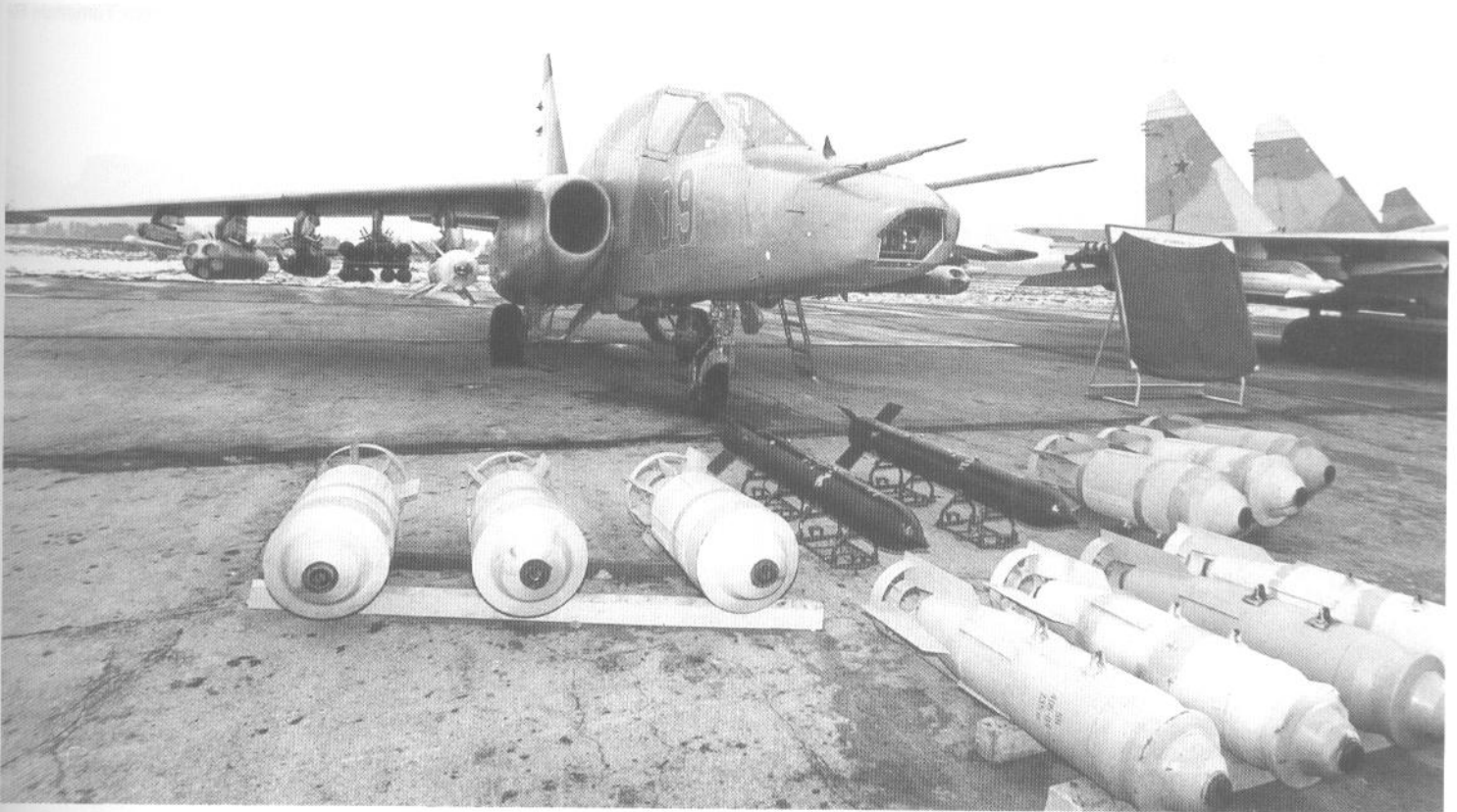
Su-25T aircraft shown during the exposition for CIS leaders in Minsk, February 1992. Free-falling bombs and unguided S-24 missiles are seen in front of the aircraft. Under the wings, looking from the fuselage, you can see: Kh-29L heavy laser guided ASM, pack with eight "Vikhr" anti-tank missiles, an Kh-25ML laser guided ASM, B-13 rocket launcher containing five S-13 unguided rockets and an R-60 defensive AAM. (Dmitri Grinyuk)
