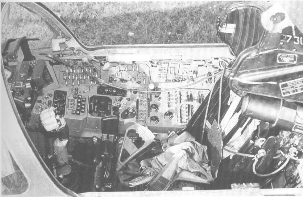
The new cockpit was equipped with the new K-36DM ejection seat, which is still standard equipment for all the contemporary Soviet aircraft. (Piotr Butowski)
