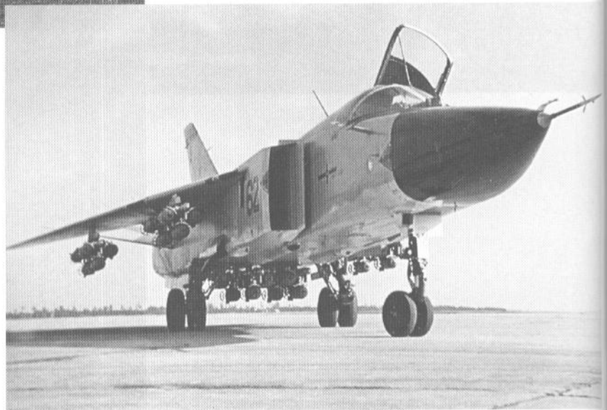
T-6-2 prototype with variable geometry wings came into being in 1970. (Sukhoi Design Bureau)
