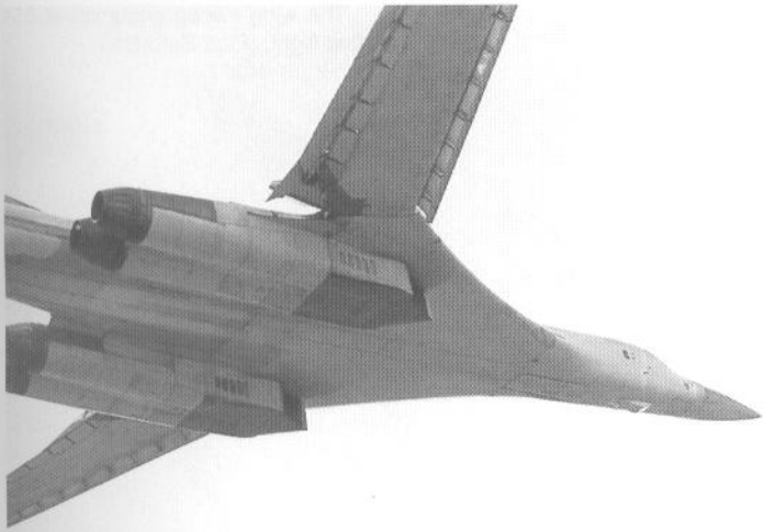
The Blackjack flying majestically at low speed. Note the high-lift devices: protruded slots and double-slot rear flaps. The Tu-160 Blackjack is the newest aircraft of the former USSR. (Piotr Butowski)
