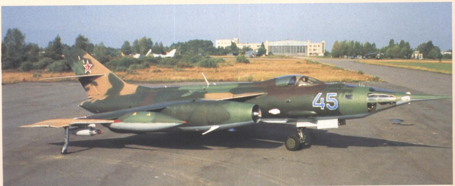
Yak-28PP. The UB-16-57 launcher under the outer wing houses sixteen S-5P chaff/flare rockets. (Piotr Butowski)
