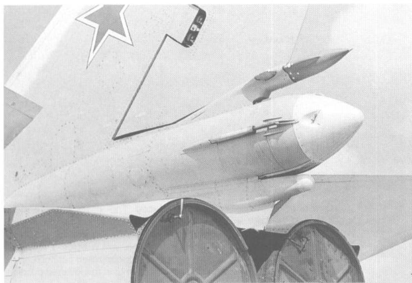
The rear section of the fuselage, with its large braking-parachute housing is typical of all versions of the Su-24, except the Fencer-A. (Piotr Butowski)
