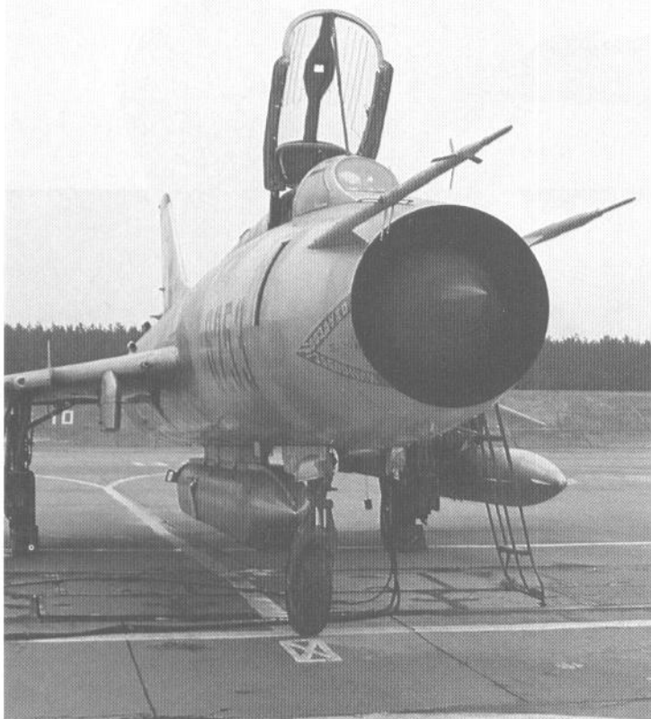
In the late 1970s, the Su-17M (Su-20) aircraft was adapted for carrying KKR-1 reconnaissance containers. (Piotr Butowski)
