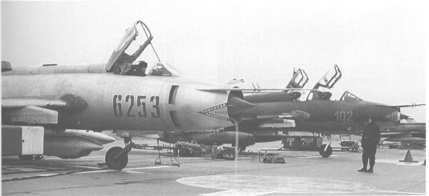
A Su-20R Fitter-C during the engine test prior to take-off on a reconnaissance flight. The thin line entering the air intake is a puddle, left after recent rain, being sucked out. (Piotr Butowski)
