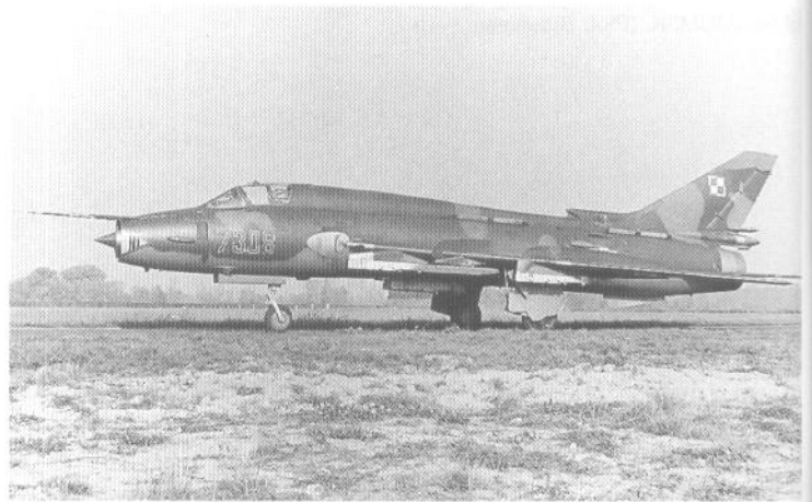
The final Fitter product, the Su-17M4 Fitter-K, manufactured serially in 1980-1990, was named the Su-22M4K for export. The photo shows a Polish Su-22M4K. The Polish Air Force uses 86 aircraft of this version and also 19 Su-22UM3K two-seaters. (Piotr Butowski)
