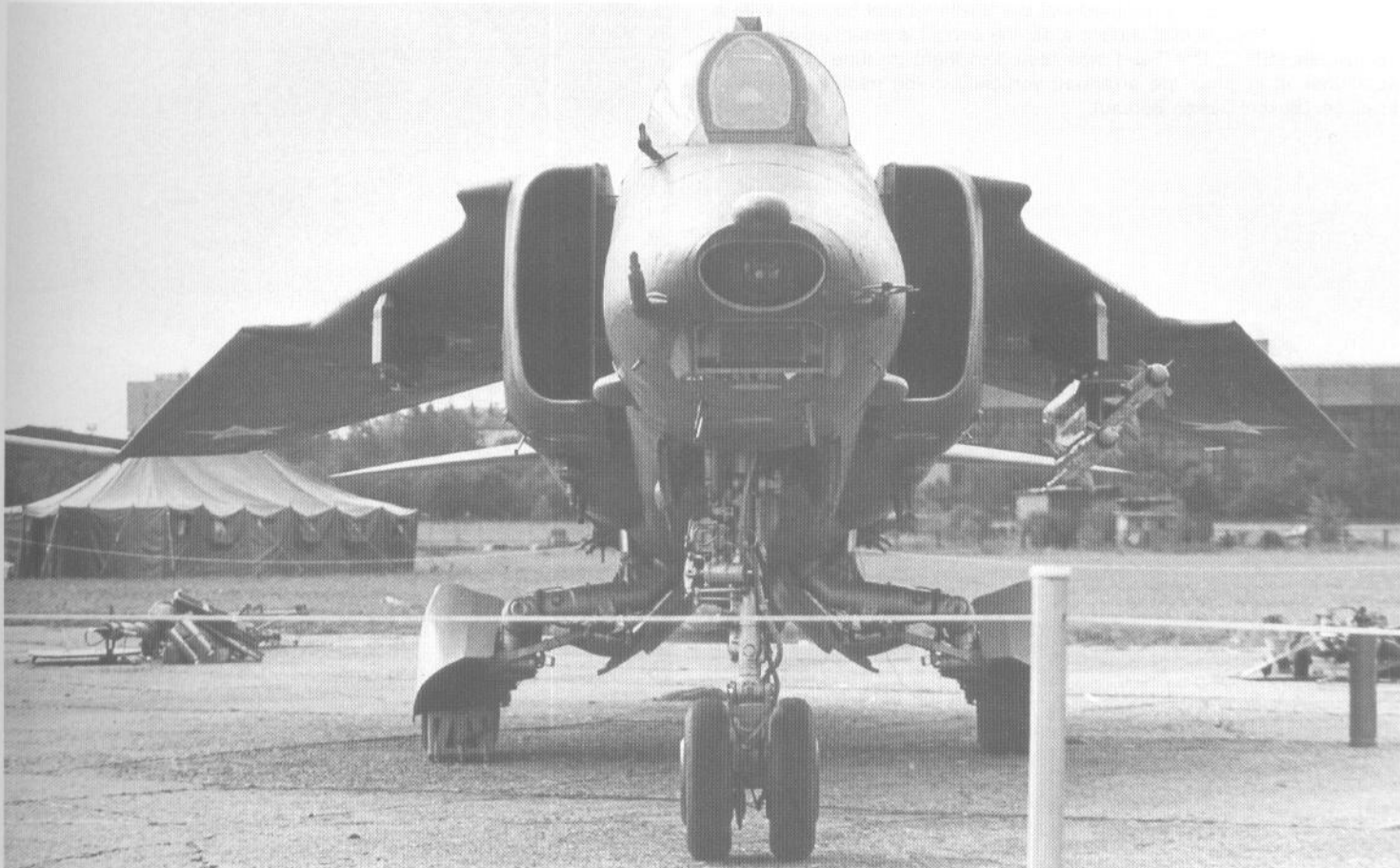
The newest modification of the MiG-27 is the MiG-27K Flogger-J with the new Kaira TV-controlled weapon system. (Piotr Butowski)
