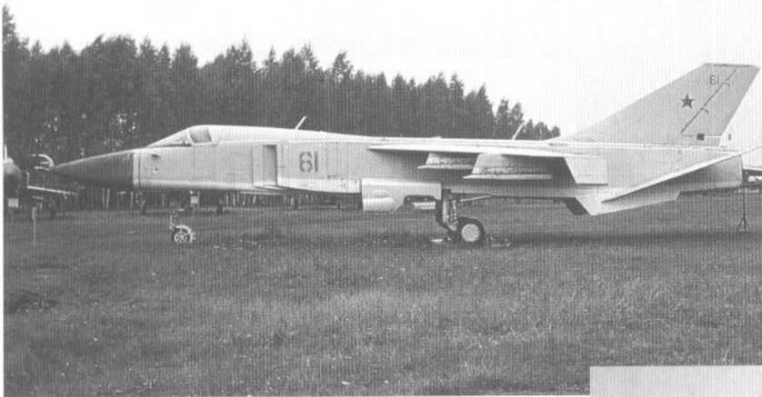
A T-6-1 aircraft displayed at the Monino museum near Moscow. During tests, the cockpit canopy was torn apart and cut off the top of the tailfin (note the tailfin is shorter than on other Su-24 aircraft). The T-6-1 was later used as a flying stand for testing the equipment and weapons. (Piotr Butowski)
