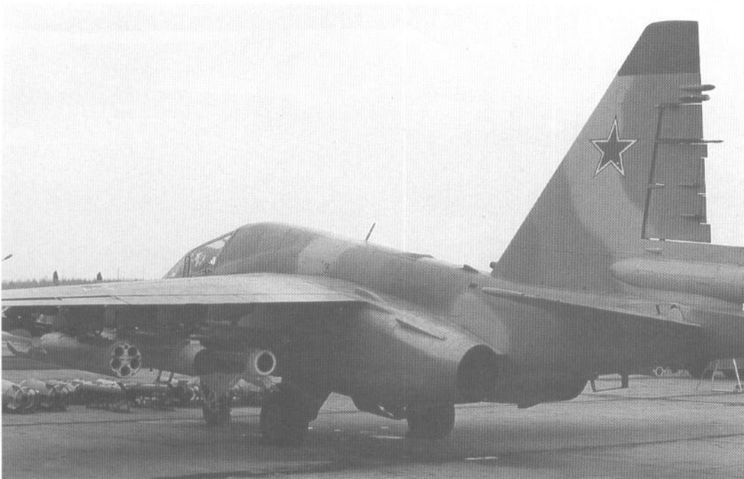
In 1992, the manufacture of the Su-25T begins. Inside the Sukhoi design bureau this version is called the Su-34; with the name Su-25TK it is offered for export. The external appearance of new Su-25T differs from the old Su-25 due to the "hump" on the fuselage behind the cockpit and the large fairing (for the 192-tube chaff/flare dispenser) on the tailfin. Inside the aircraft there is new armament: the Shkval LLTV-system ( shkval for squall) and the Mercuri FLIR pod, used for night attacks. (Dmitri Grinyuk)
