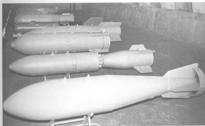
FAB-500M-62 (model 1962), a standard Russian demolition bomb (in the foreground), BetAB-500ShP bomb designed to destroy concrete fortifications and runways (next in line) as well as FAB-500ShN bomb (third in the row). (Piotr Butowski)
