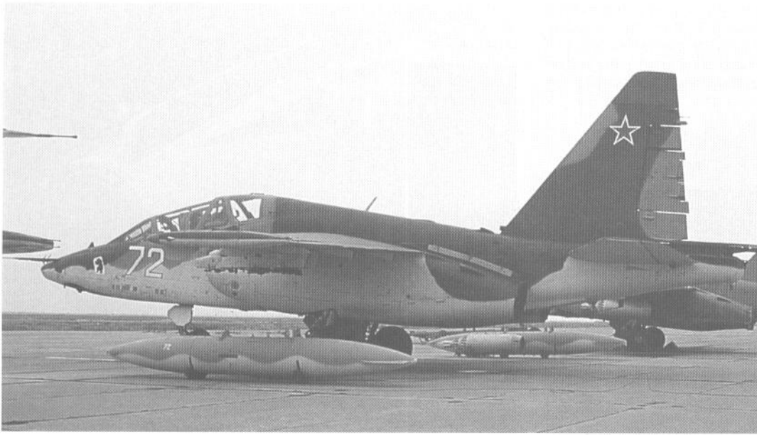
A Su-25UB. Note the auxiliary fuel tank under the aircraft wings. (Piotr Butowski)
