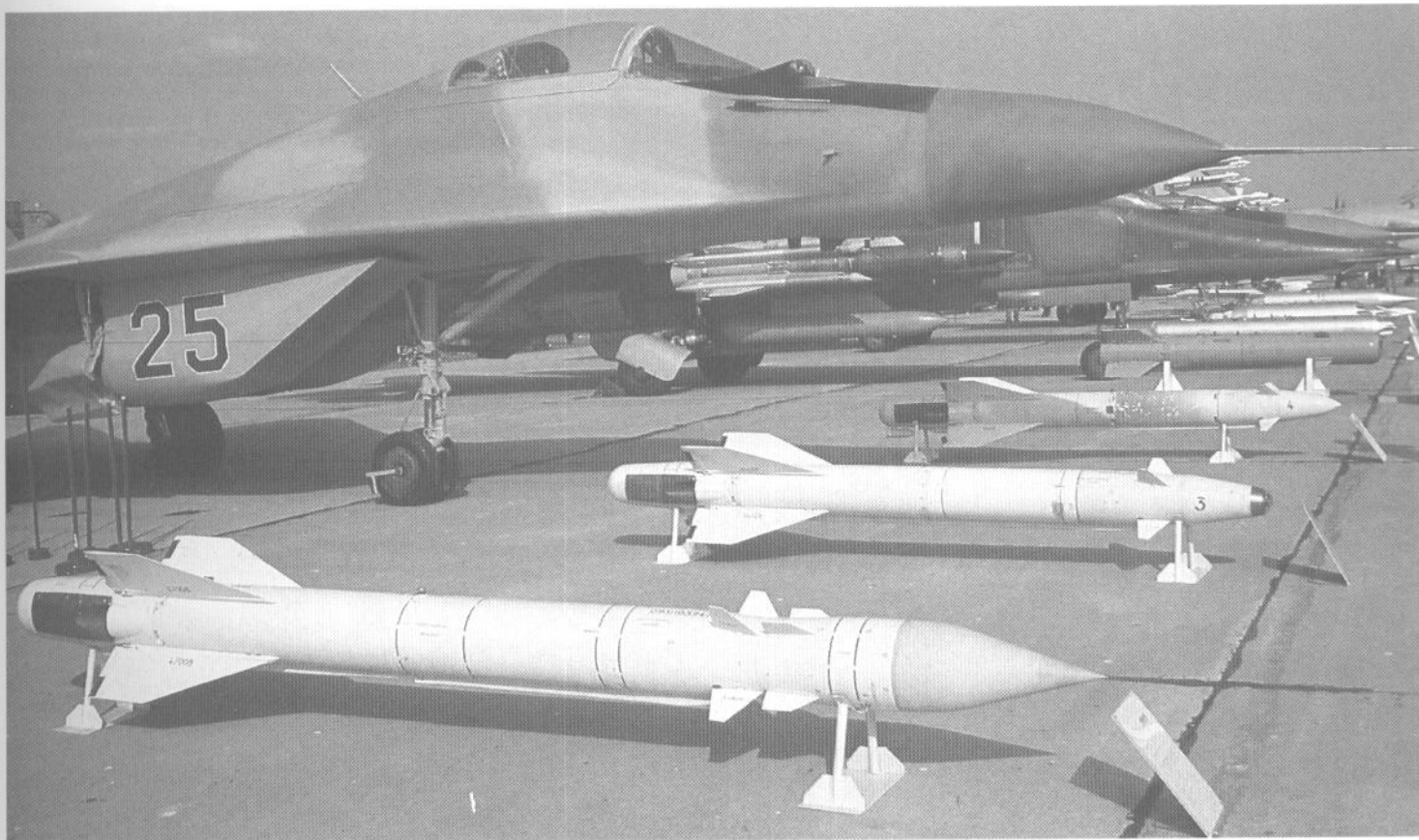
There are three versions of Kh-25 module air-to-surface missile: anti-radiation Kh-25MP (AS-12 Kegler), laser guided Kh-25ML (AS-10 Karen), as well as radio-command guided Kh-25MR (AS-10 Karen). The Kh-25 missile is a standard armament of former Soviet strike aircraft. (Piotr Butowski)
