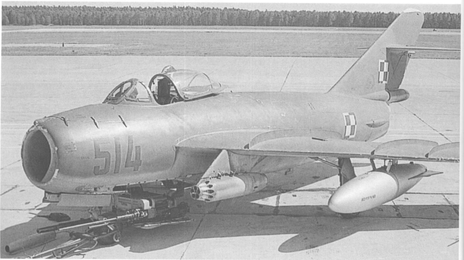
The light attack aircraft Lim-6bis was finally withdrawn from the active service in Polish Air Force in March 1992. Lim-6bis is a Polish-made version of MiG-17 Fresco, used as a light ground attack aircraft. The photo shows the pods under the inboard section of wings (absent in original MiG-17) mounted with UB-16 57mm rocket launchers. (Piotr Butowski)
