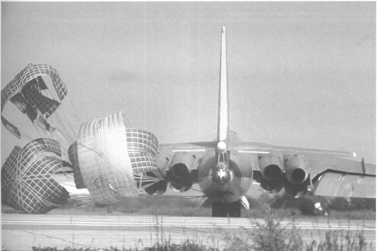
A landing 3MS-2 Bison-B with three braking parachutes released from under the fuselage. (Anatoli Andreyev).
