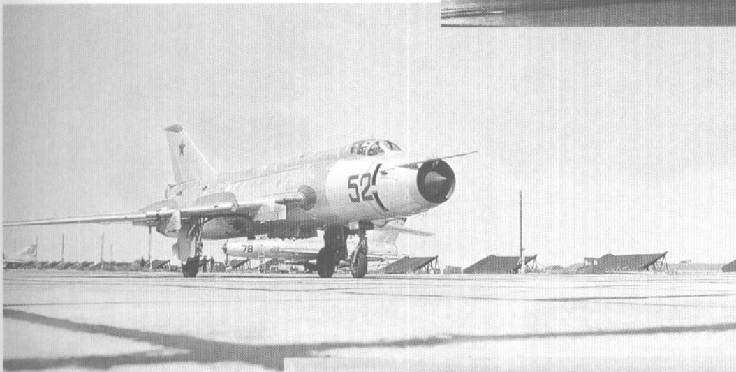
The Su-7 Fitter-A aircraft has been chosen by Sukhoi's team as the basis for the new design, the Su-17 Fitter-B. The wings have been redesigned into a variable geometry model with movable ends. The changes in external appearance include: the cockpit canopy opening upwards instead of sliding back, as in the Su-7; a fairing between the pilot cabin and the tailfin; and some minor changes in the arrangement of aerials. Also two big armament-carrying beams have been suspended under each wing. In 1972, two Soviet VVS regiments were equipped with the Su-17 aircraft.
