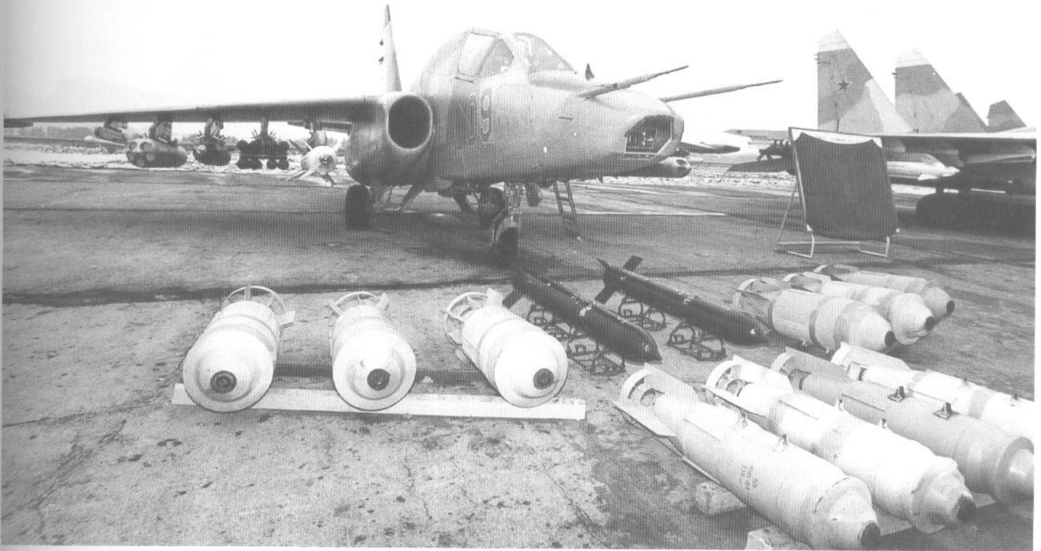
Su-25T aircraft shown during the exposition for CIS leaders in Minsk, February 1992. Free-falling bombs and unguided S-24 missiles are seen in front of the aircraft. Under the wings, looking from the fuselage, you can see: Kh-29L heavy laser guided ASM, pack with eight "Vikhr" anti-tank missiles, an Kh-25ML laser guided ASM, B-13 rocket launcher containing five S-13 unguided rockets and an R-60 defensive AAM. (Dmitri Grinyuk)
