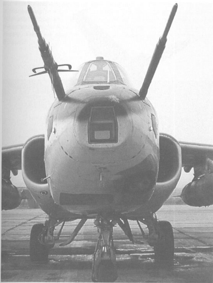
The Klion laser rangefinder and target designator's window in the nose of the Su-25 Frogfoot A. Note the twin-barrel 30mm cannon on the bottom of the front fuselage, on the port side. (Piotr Butowski)
