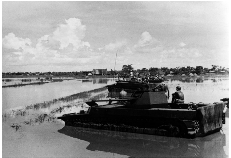
Mounting 40mm Bofors guns, Alligators of 6e GEA/1er RCC form a 'bouclage' (cordon) near Nam Dinh, 1953. A number of LVT4s were fitted at Haiphong naval arsenal with an open-topped turret mounting a Bofors for the fire-support role. These vehicles were only employed by the amphibious units of 1er RCC – note the regimental insignia well forward on the hull sides. They proved effective in the Tonkin deltas, but the increased weight and height affected their seaworthiness, so they were rarely used in amphibious coastal assaults. With no threat of air attack, the equipment of the Artillerie Antiaérienne Légère units was distributed for other purposes; 40mm Bofors guns were deployed on armoured trucks, armoured trains and LVTs. (Author's collection)
