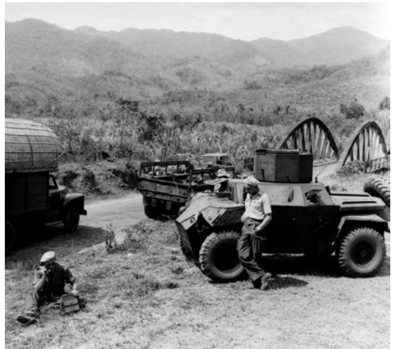
Mounting a locally fabricated machine-gun turret, a Humber Scout Car Mk II of the 5e Cuirassiers guards a bridge while protecting a convoy on the road to Dalat, southern Annam, in 1952. Typical armament was two machine guns, with the second in the hull. These turrets were made at the Saigon Naval Arsenal. The French acquired some 78 examples of the Humber scout car. Intriguingly, Humber scout cars with locally produced turrets were still used up until 1974 by Portuguese troops during the war in Angola. (Author’s collection)
