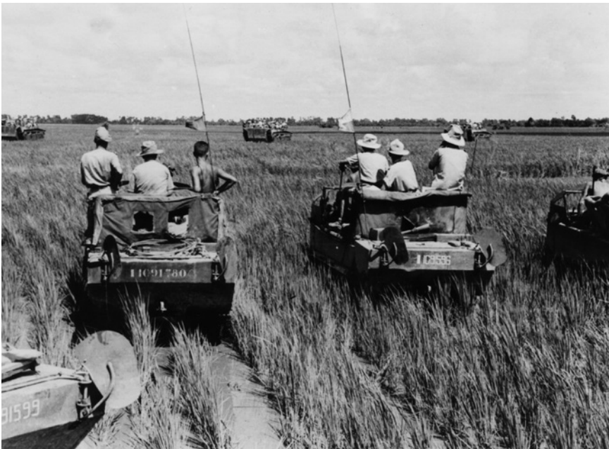
Crabes and Alligators of 2e Esc, 1er Groupe d'Escadrons/ 1er REC plough through a rice paddy in support of Legion 13e DBLE infantry near Tra Vinh deep in the Mekong Delta during the first operation with LVTs in November 1950. During operations in paddy fields and swamps the suspension of the M29C tended to become clogged with rice shoots and other vegetation that overtaxed the relatively fragile mechanism, so crews had to dismount repeatedly in order to clear the bogie wheels and tracks. (Author's collection)
