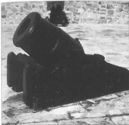
A 12-inch iron naval mortar cast in 1772 on a Gribbeauval pattern bed. (Fort Ticonderoga. Photo RC)
