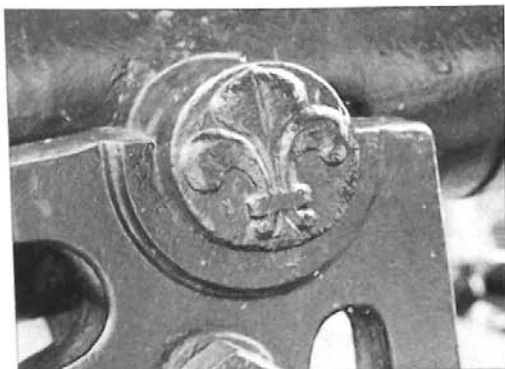
BELOW Fleur-de-lis cast into the right trunnion of the naval 18-pdr iron Model 1778 gun. According to the 1767 instructions, it was the foundry's name or marking that was to be cast in the right trunnion. However, the foundry at Indret – which cast this gun between 1781 and 1783 – obviously decided to show the lily on the left trunnion and its name on the right. A good many of Napoleon's naval guns still bore the royal lily. (Photo RC)
