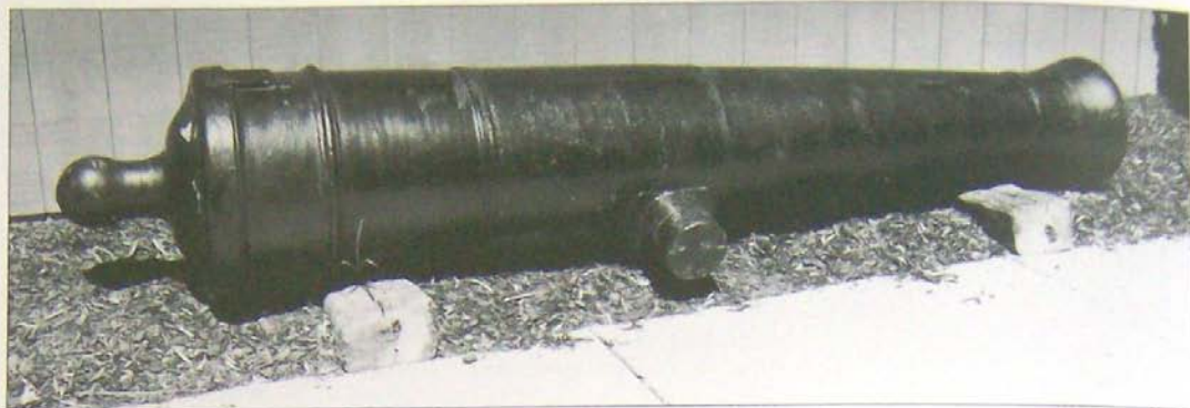
Side view of a French naval 36-pdr iron model 1786 cannon cast in Liège in 1807. (Courtesy of Scott Sheads)
