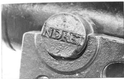
ABOVE 'INDRET' cast into the left trunnion of a naval 18-pdr iron model 1778 gun cast in 1785. According to the 1767 instructions, this trunnion was to have the initial of the master founder. The foundry at Indret cast its first guns in 1778, became a royal (or government) establishment in 1781 and remained an important gun maker during the Napoleonic era. (Photo RC)
