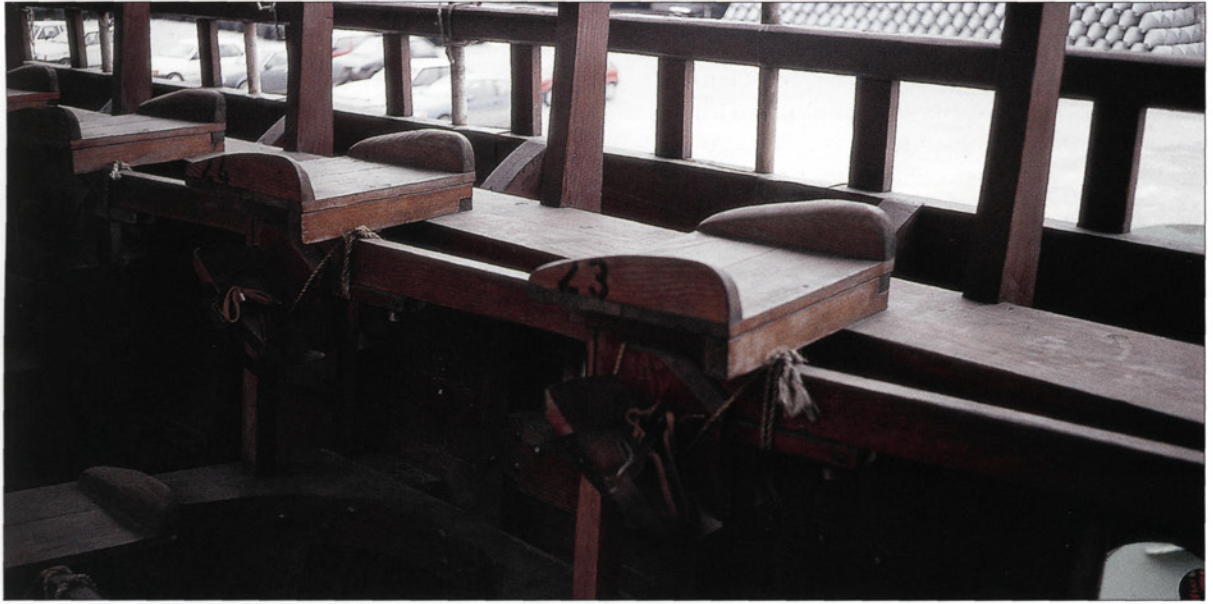
The fixed seats on Olympias . Every oarsman had a cushion – perhaps a seat pad made of sheepskin – and was doubtless assigned a regular seat on board. This would allow him to get used to the timing of the men around him and to adjust his stroke accordingly. (Author's collection)
