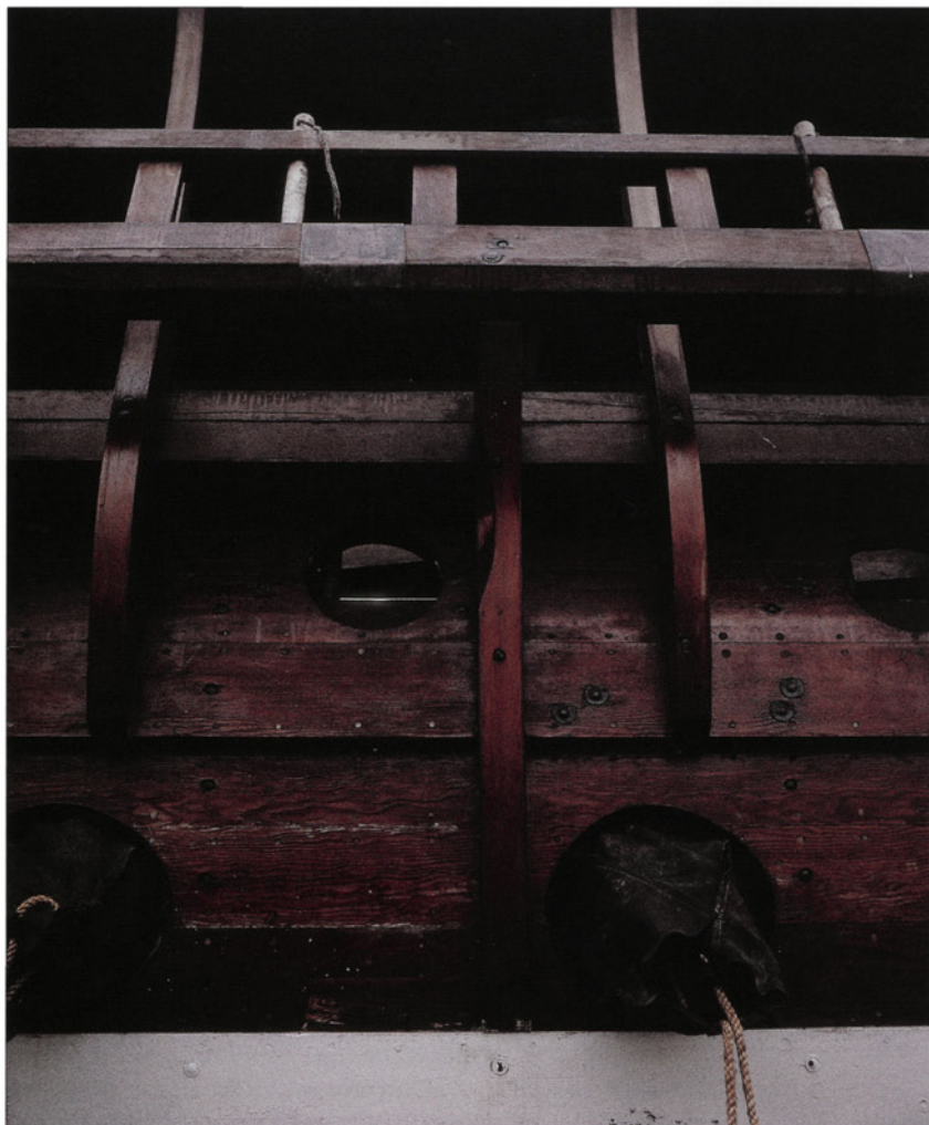
Askōmata were leather sleeves through which the thalamioi worked their oars. They were used to prevent water coming through the lower and larger row of oar-ports when the sea was choppy. Immediately above these two askōmata are two zugioi oar-ports, and above those two thranítai tholepins. (Author's collection)
