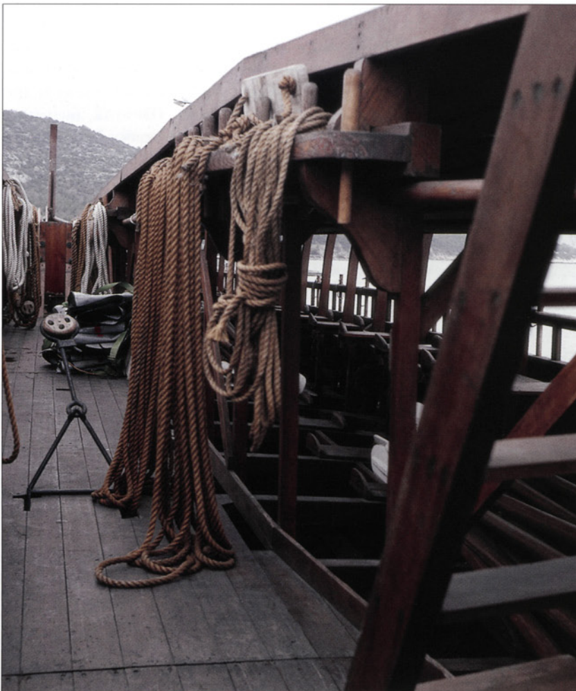
The quarterdeck ladder and gangway on Olympias . The bo'sun stood in the gangway, midway along, and called out instructions to the oarsmen. He had the help of the bow officer, while a piper kept time on a shrill double pipe. (Author's collection)
