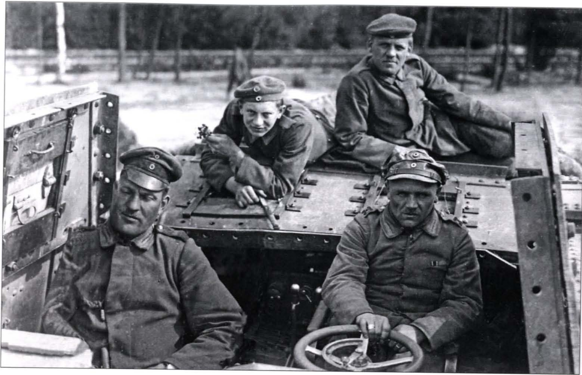
ABOVE The roof of the command cupola could be removed and the front and rear panels folded down to make it easier to drive the A7V when outside the combat area. This is the crew of Panzer 563 "Wotan" during a rail movement in July 1918. Like the rest of the final production batch, Wotan was fitted with appliqué armor on the cupola. (NARA)
