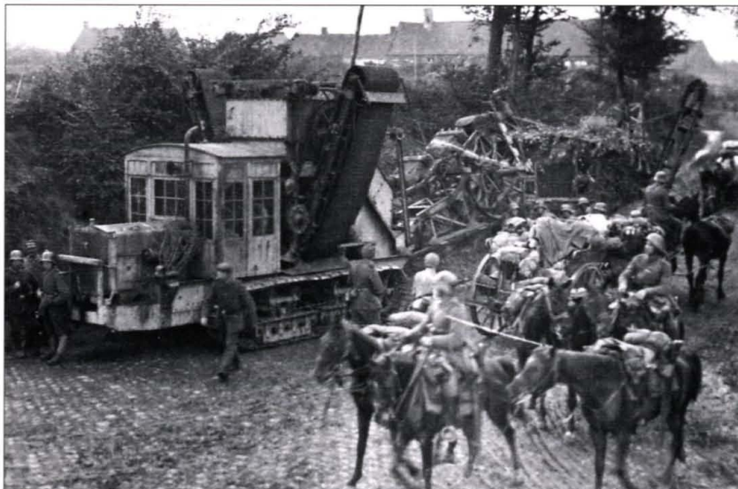
At least a single example of the A7V-Schützengrabenbagger trench-digger was completed, and it is seen here moving to the front on October 28, 1918. (NARA)
