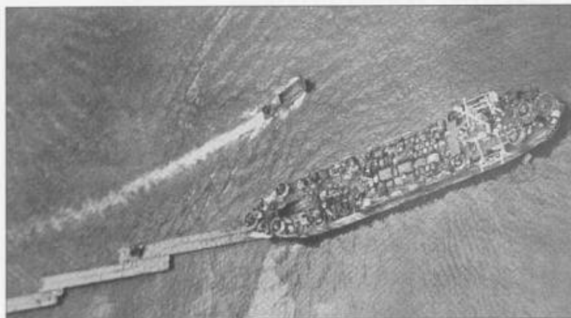
An LST, its weather deck fully loaded, is nosed up to an extended causeway at Peleliu. Four additional causeway sections are off-frame. The staggered causeway provided vehicle bypasses and helped resist lateral currents. An LCM(3) scoots past.
