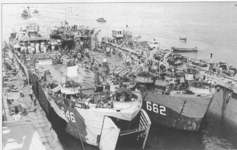
Construction details varied between LSTs, as demonstrated by LST-646 and 662 afloat in ABSD-6 (advance base section dock). LST-646 is fitted with two Welin-type davits and has a twin and two single 40mm guns on the forecastle. LST-662 has six pairs of davits and mounts a twin and four single 40mm guns plus two 20mm cannon aft of the twin 40mm. Note the movie screen (white square) aft of the forecastle on the weather deck.
