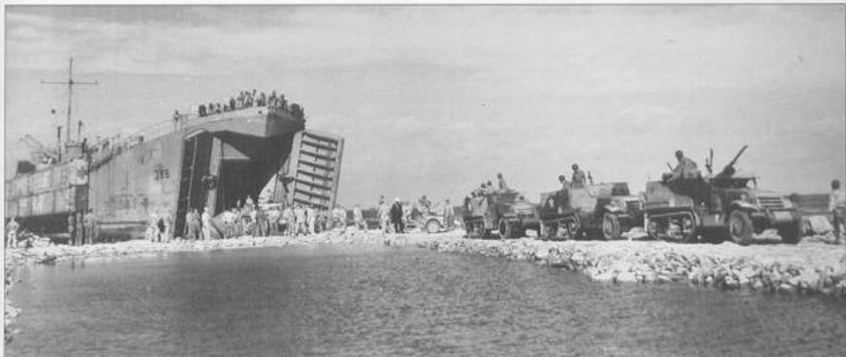
LST-396 unloads M3 halftracks across a coral causeway, making the pontoons on her sides unnecessary. She is spot-painted in an effort to protect chipped off rust spots. The pontoons were typically battered, rusted, and scarred from hard use. The hull number is in black 2ft figures.
