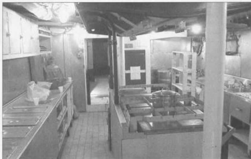
The aft-most compartment in the deckhouse is the galley. Like the wheelhouse, LST-325's galley has changed little and still boasts stainless steel appliances: steam table serving line, two grills, two ovens, large cooking and coffee kettles, dishwasher, and even an automatic potato peeler, all electric-powered.
