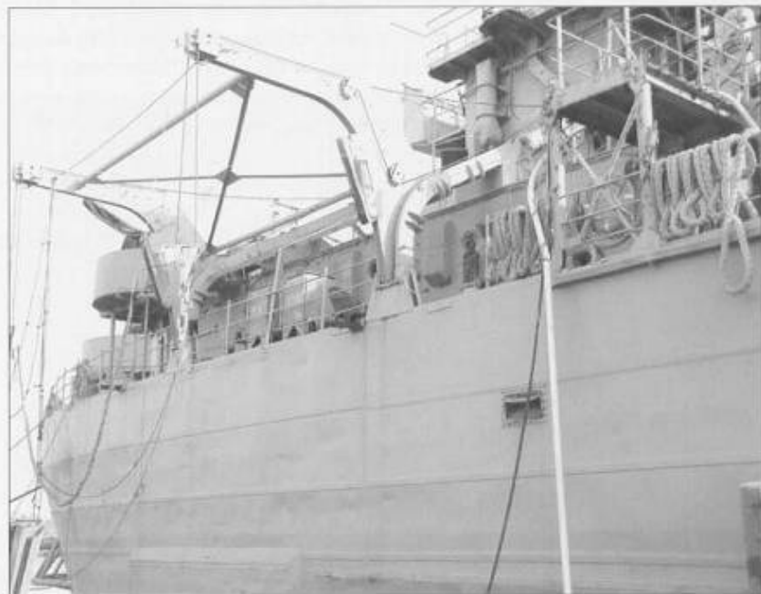
Aft starboard side of LST-325 shows the Wellin-type davits in the lowered position. The after 40mm tubs can be seen behind the davits and the end of the signal bridge in the "V" of the forward davit. The port on the hull is the main engine exhaust vent.
