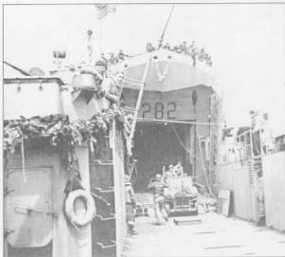
An alternate means of disembarking vehicles from an LST when pontoon causeways were not available was the employment of LCT(6)s with their stern plates removed.
