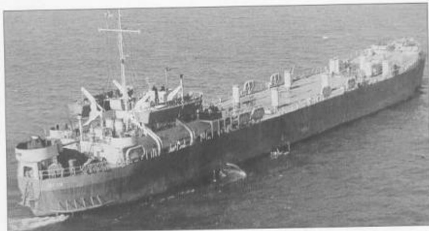
LST-172 provides a view of an uncluttered ship before additional armament was added. It is armed with a 40mm and two 20mm guns on the bow, a 20mm on each corner of the deckhouse, and a 3in gun on the stern. The two stacks aft of the bridge are the aft-most tank-deck ventilators.
