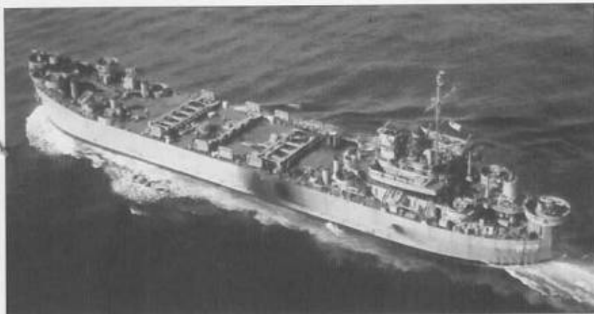
LST-882 is fitted with timber cradles to carry an LCT and is painted haze gray. The black smudge on the hull side below the deckhouse indicates the main engine exhaust vent.
