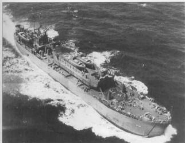
HMS LST-214 crosses the Atlantic en route to Britain with an LCT(5) carried on the weather deck. Two Army Motor Towboats, Large (MTL) are chocked inside. An LCP(L) is carried in the starboard davits.
