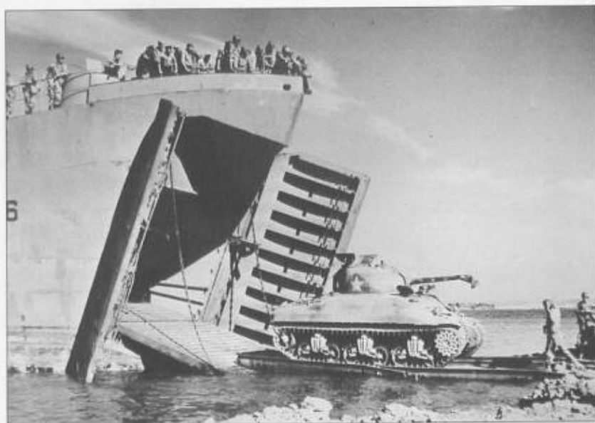
The main reason for the creation of the LST was to deliver large numbers of tanks to hostile shores. Here an M4A1 Sherman medium tank rolls off an LST over British-designed 10ft-long Vehicle Landing Ramps (VLR). The inside of the doors was normally gray, but was often repainted lead red, black, or one of the colors used for the hull camouflage.
