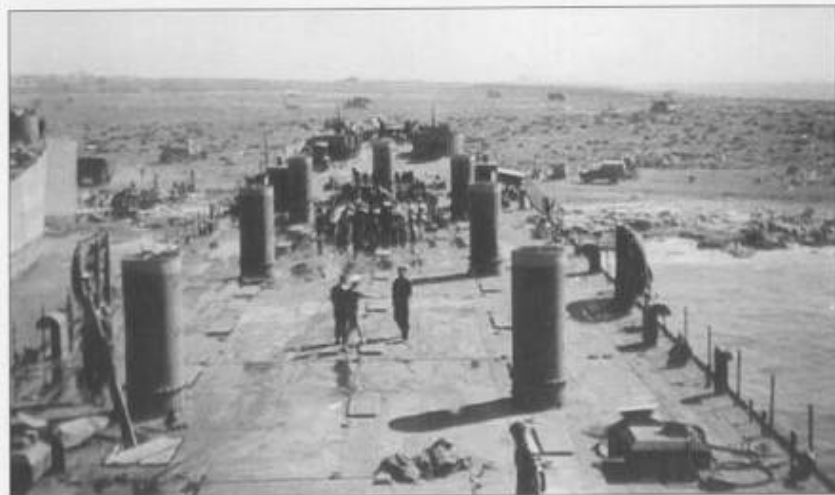
This view of the weather deck of a British-manned LST provides an idea of the parking space available. The tank-deck vent stacks could be relocated to alternate openings just forward of the deckhouse. With only two 20mm guns on the forecastle, this ship appears less cluttered than US LSTs with their multiple gun tubs clustered on the forecastle.
