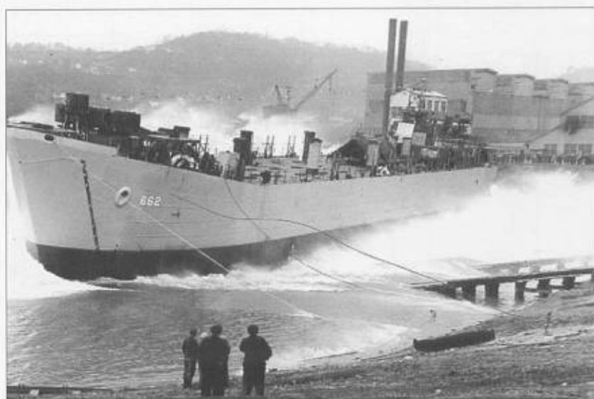
LSTs built in the river yards were launched sideways because of the shallow and narrow waterway. Here LST-662 is launched at American Bridge, Ambridge, Pennsylvania. A 328ft ship impacting broadside after sliding 20-plus miles per hour down the way was impressive.
