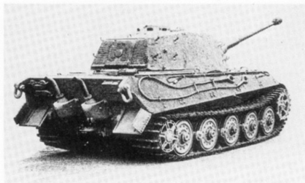
ABOVE AND BELOW From an official manual: photographs of a Tiger II ready for transportation by rail. The tracks are the narrow transport track. (Author)
