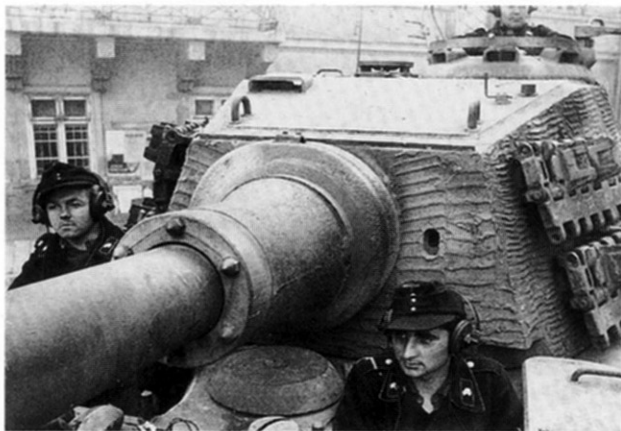
Close-up of the gun and mantlet front of a Henschel turret clearly showing the coating of
