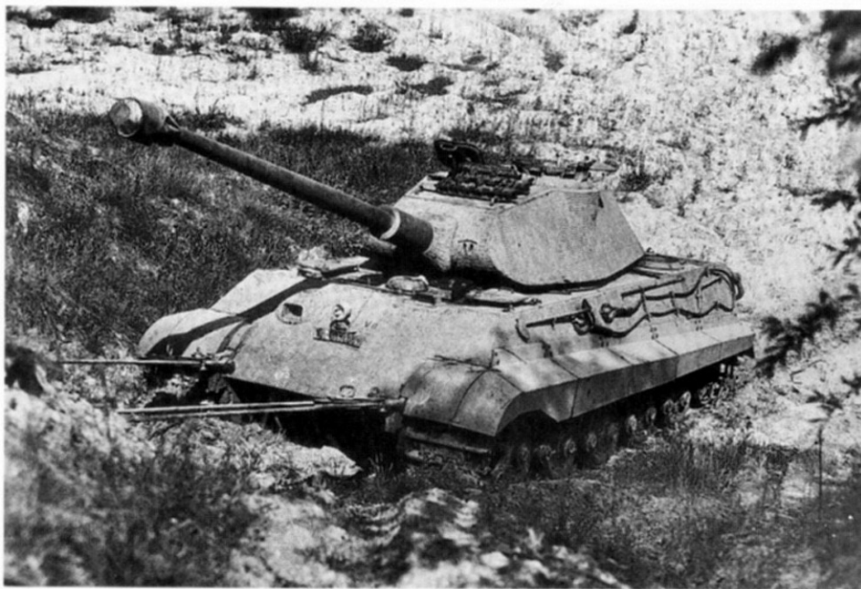
Versuchs Nr. V8 was also one of the production Tiger IIs tested by the Waffenamt. The test number 212 is on the right hand side mudguard under the shadow cast by the gun. Here we see tests on recovery methods for this new type of heavy tank. (Bundesarchiv)
