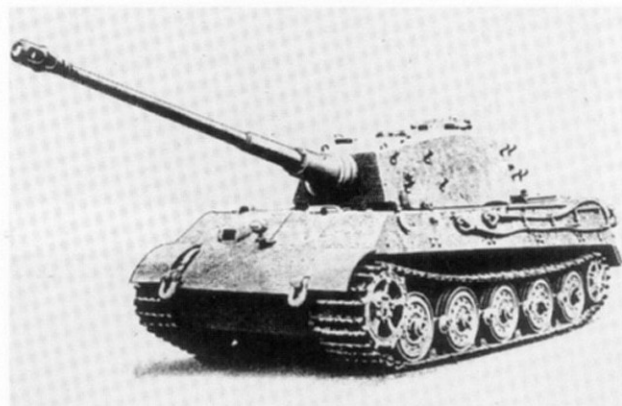
ABOVE AND BELOW From an official manual: photographs of a Tiger II ready for transportation by rail. The tracks are the narrow transport track. (Author)
