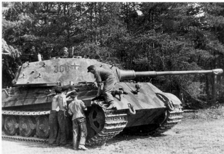
After completing the camouflage the crew fit the armoured mudguards. The call sign '300' in black, according to regulations, is still to be outlined in white. The spare track hangers show that this Tiger II was produced in July 1944. (Bundesarchiv)
