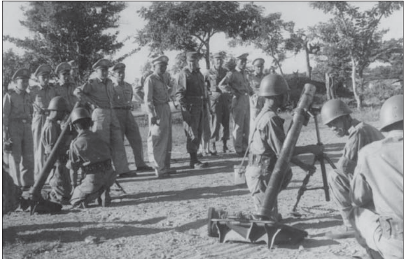
Vietnamese National Army troops demonstrate crew drill on French 81mm M1927/31 mortars. The US 81mm M1 mortar, license-built from the French model, was virtually identical but had a smaller base plate. Other heavy mortars supplied during the war included the 81mm M29 and 4.2in M2 and M30. (Courtesy Paxton Williams)
