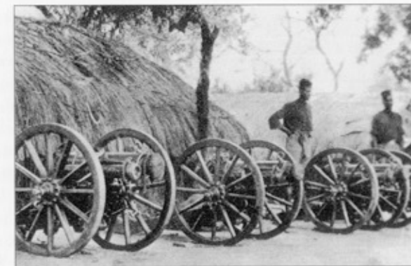
These 2.95in mountain guns of the Nigerian Artillery were employed in the campaign in East Africa. The gun weighed 827lb, and when broken down into pack-loads is reported to have been carried by porters. Nigeria contributed five infantry battalions and two artillery batteries to the West African Frontier Force in 1914. (Author's collection)
