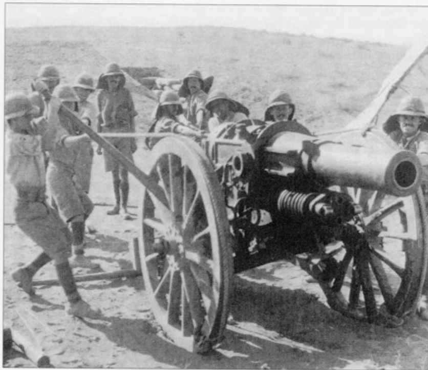
A 6in howitzer being hauled into position in Mesopotamia, 1918. This weapon – like many provided for theatres other than the Western Front – was obsolescent, with a maximum range of 5,200 yards compared to the 11,400 of the more modern mark used in France. (Author's collection)
