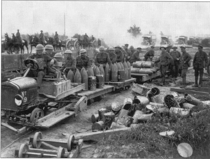
A cargo of 9.2in howitzer shells moving forward on a narrow gauge railway, 1918. The towing vehicle is a converted Model 'T' Ford car. In the background are horses towing limbers, and a convoy of lorries. (IWM)
