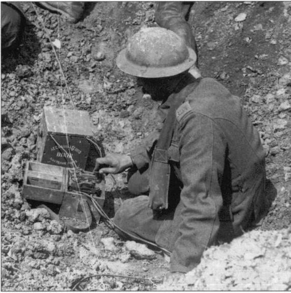
A Royal Garrison Artillery 'Fullerphone' in operation, 1918. More secure than a field telephone, its signal was sent by Morse key. The diagonal white line is a crack in the glass negative. (IWM)
