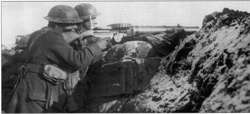
January 1918: Lewis gunners of the 15th Royal Scots (34th Division). Weighing 27lb, the Lewis was a gas-and-spring operated automatic firing .303in ammunition at a cyclic rate of 550 rounds per minute. Its maximum effective range varied from 800 to 1,100 yards according to the skill of the firer. (IWM)
