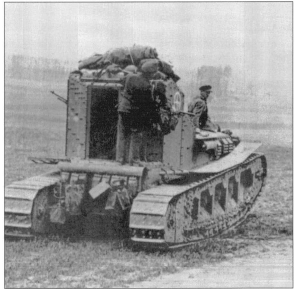
March 1918: a 'Whippet' tank of 3rd Bn, Tank Corps, moves into action. The rear door was the entrance to the fighting compartment, which mounted four Hotchkiss machine guns. (Author's collection)
