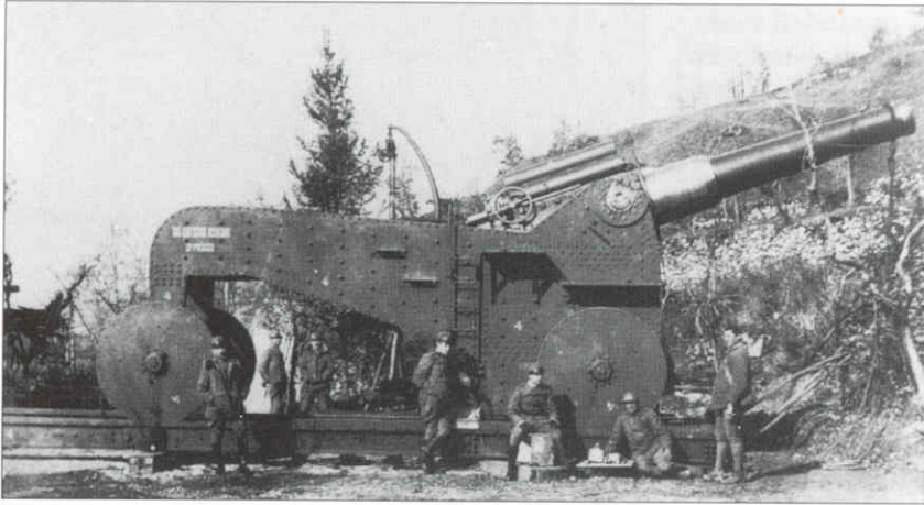
A 305mm howitzer, known in Italy as a 'heavy mortar', on a De Stefano carriage; this distinctive system featured four large solid iron wheels running on rails to absorb the recoil. It came in several sizes, some of which were designed for the largest guns. Among other types of carriage used by the Italian artillery was the Garrone system, which had 'tracks' around the wheels, usually with ramps up which the wheels rolled under recoil. Other heavy ordnance was mounted on trains, including the huge Ansaldo 381/40 railway gun. (A. Curami photograph)
