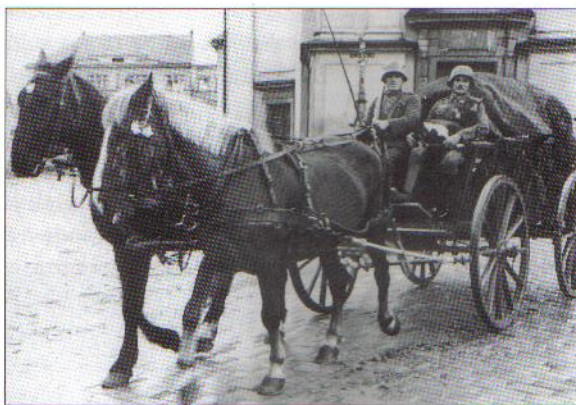
The ubiquitous Hf1 transport waggon and weapons carrier; this weighed 650kg (1,430lbs) empty and could carry a load of 750kg (1,650lbs). Note the low profile canvas cover, and the team's M1925 breast harness. Reins were of hemp or (as here) leather; an outrider was sometimes used. The horse in the foreground is a fine Haflinger. The soldier beside the driver is cradling an animal companion in his lap. (Paul L.Johnson Collection)
